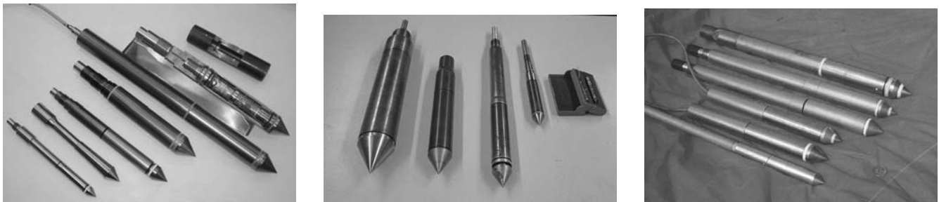
FIGURE 11 Selection of penetrometers from (left) van den Berg series, (center) Fugro series (left to right: 33-, 15-, 10-, 5-, and 1-cm 2 sizes), and (right) Georgia Tech collection (bottom to top): 5-cm 2 friction, four 10-cm 2 piezocones (type 2, type 1, type 2 seismic, dual-piezo-element), and 15-cm 2 triple-element type.
