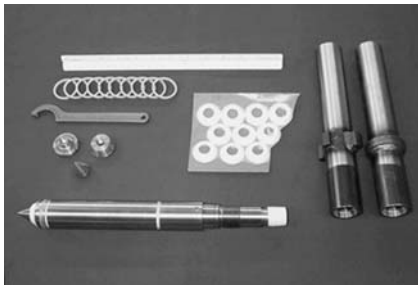
FIGURE 90 Multi-piezo-element penetrometers: (left) dual-element type with midface and shoulder filters (van den Berg type), (center) Fugro triple-element cone, and (right) quad element (Oxford University).
