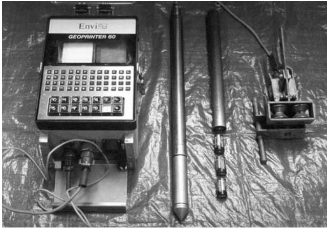
FIGURE 89 Cableless CPT systems: (left) Memocone (ENVI) and (right) audio-signal unit (Geotech AB).
