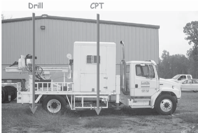
FIGURE 102 Combine rig with both CPT hydraulic rams and drilling capabilities.
