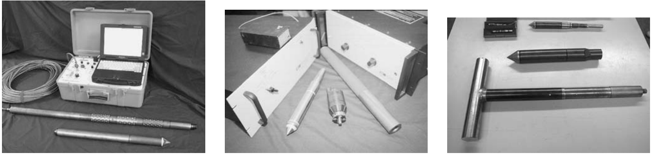
FIGURE 91 CPT modifications: (left) multi-friction sleeve penetrometer, (center) vibro-piezococone, (right) T-bar.
