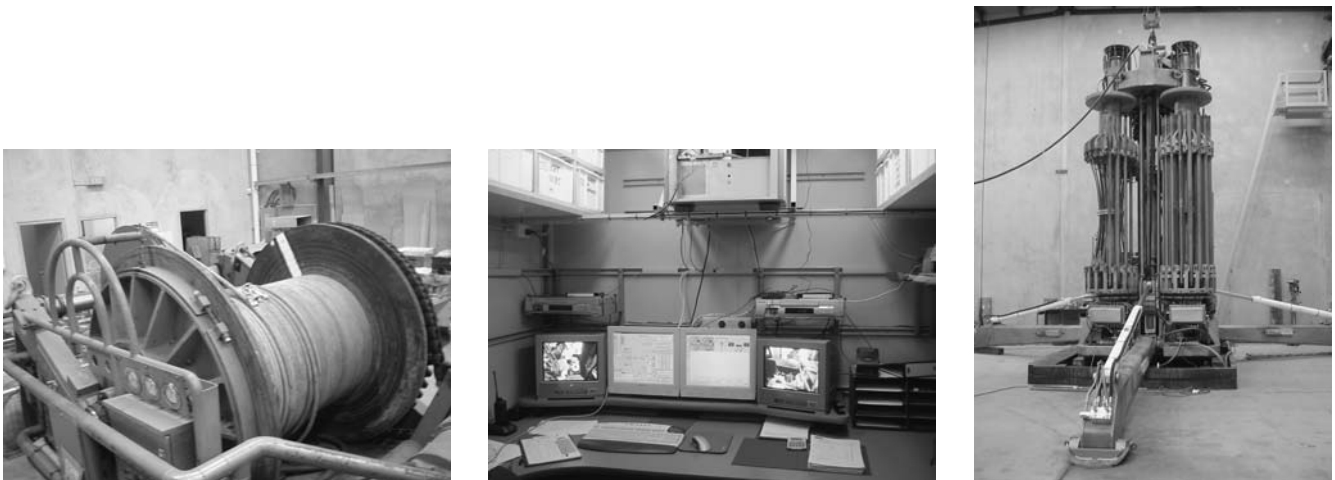
FIGURE 98 Components of portable remotely operated drill (PROD): ( left ) 3000-m-long umbilical cable, ( center ) remote control panel and data acquisition, ( right ) CPT and rotary drill platform.
