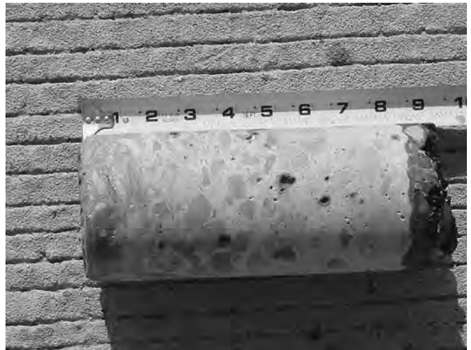
Figure 58. Measuring thickness of PCC above PATB from core.
