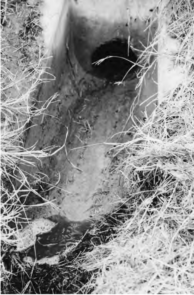
Figure 64. Bubbles from liquid soap used in pilot testing to attempt to measure time to free flow.
