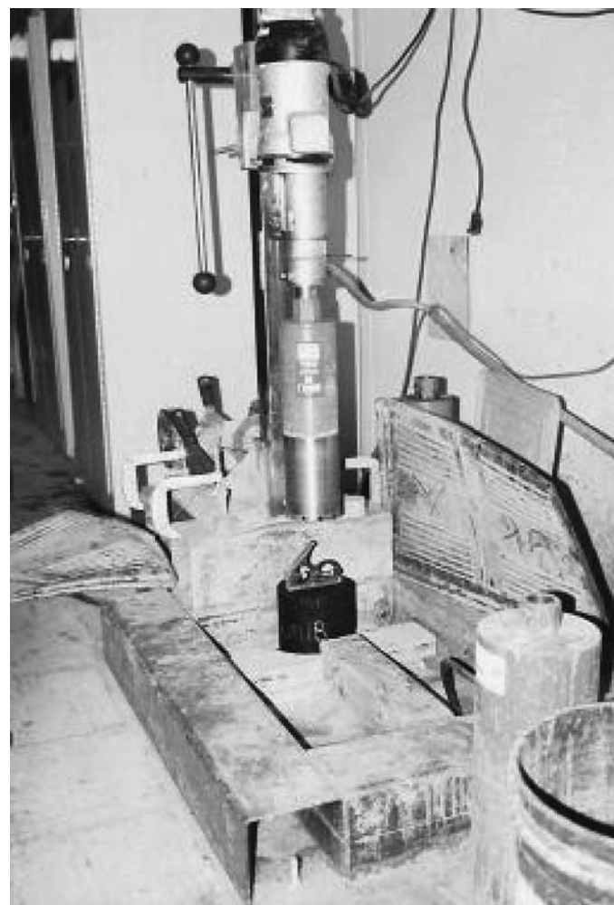
Figure 1. Portable core-drilling machine and stand.
