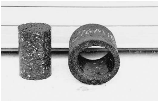
Figure 2. 100-mm-diameter core and waste ring.
