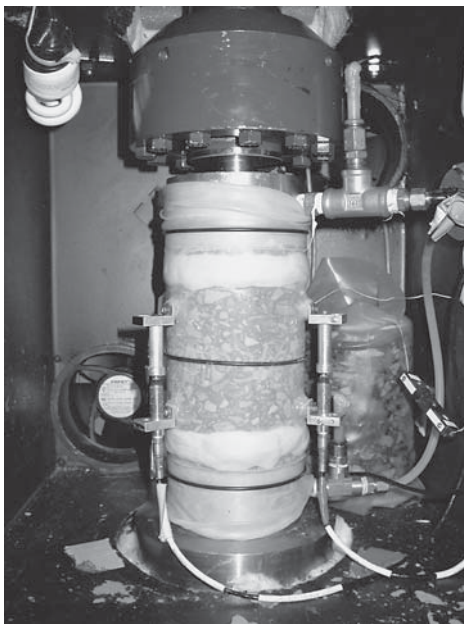
Figure 8. The specimen set-up for testing and the corresponding sinusoidal load.
