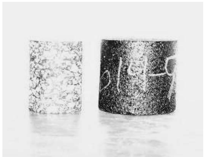
Figure 4. Final dynamic modulus test specimen.
