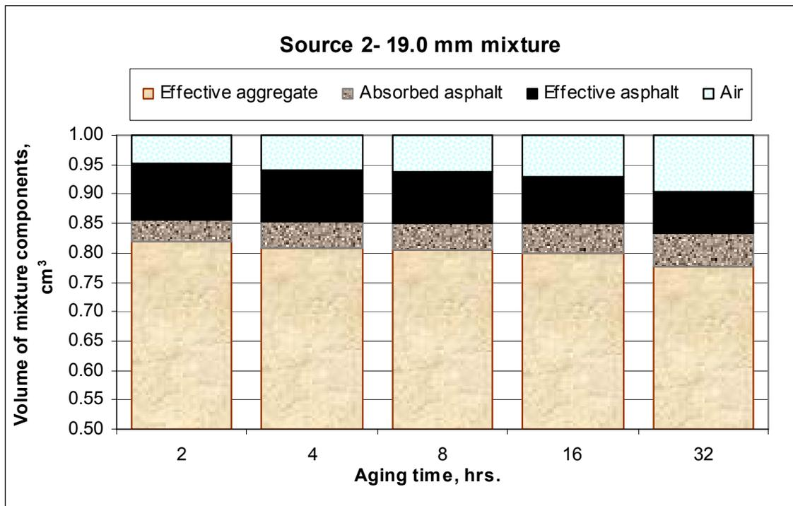
Figure 5-10- The volumetric component diagram of the S2-19-mm mixture at various aging times
