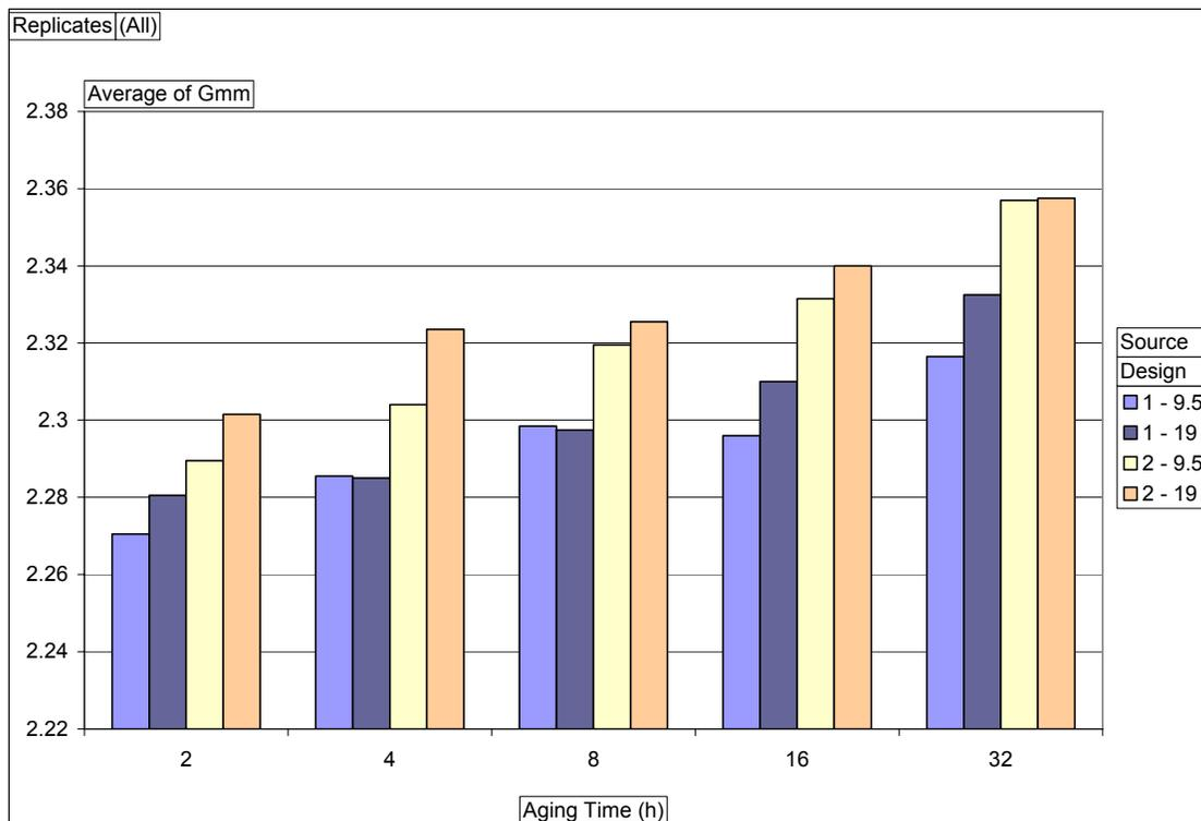
Figure 5-1- Average  $G_{mm}$  values of the four mixtures at various aging times
