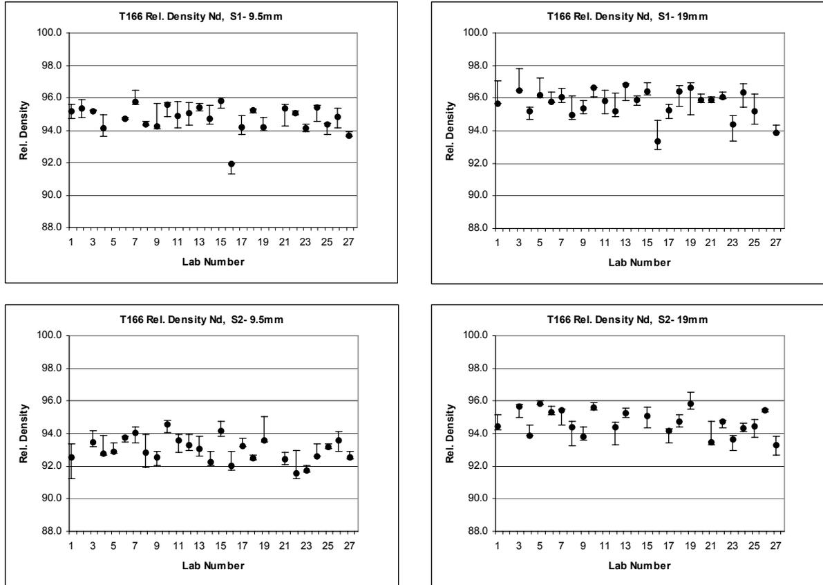
Figure 4-9 - Box plots of relative density at  $N_d$  computed using T 166  $G_{mb}$  values-T312
