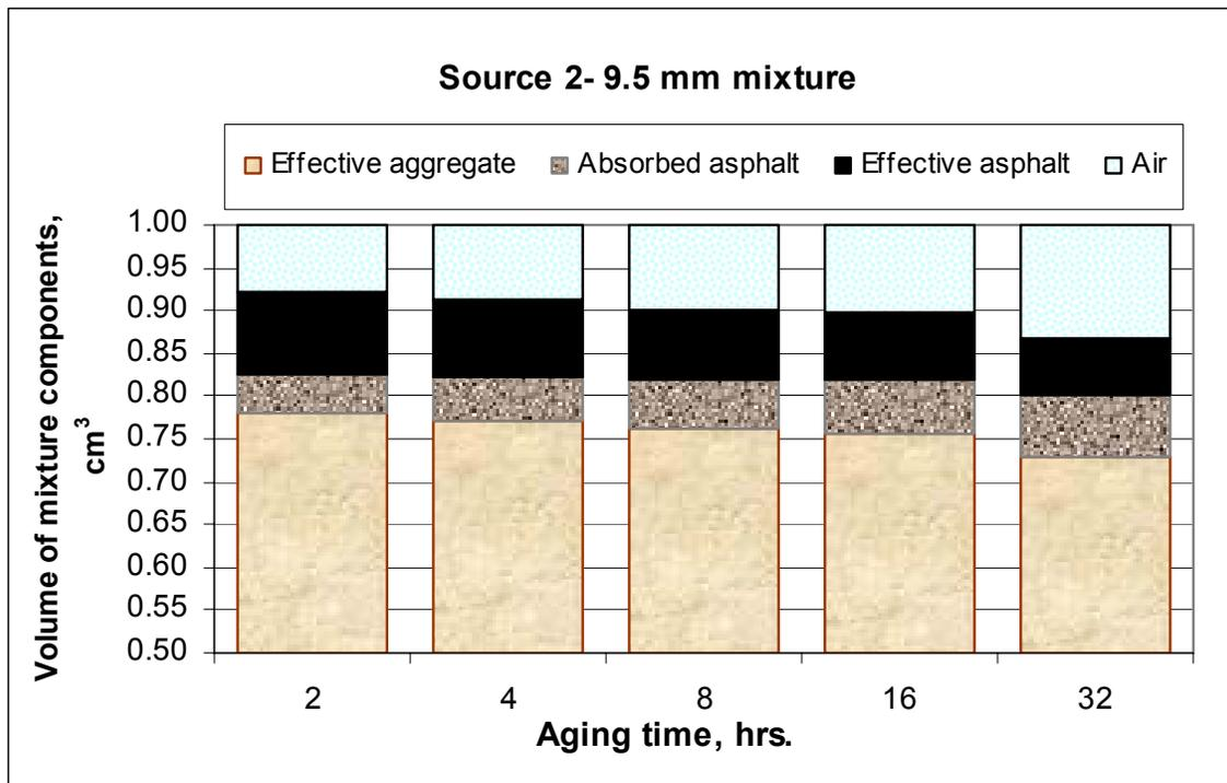
Figure 5-9- The volumetric component diagram of the S2-9.5-mm mixture at various aging times
