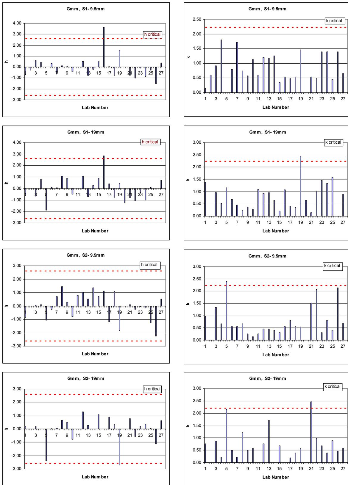
Figure 4-2- h and k consistency statistics of maximum specific gravity ( $G_{mm}$ )-D2041
