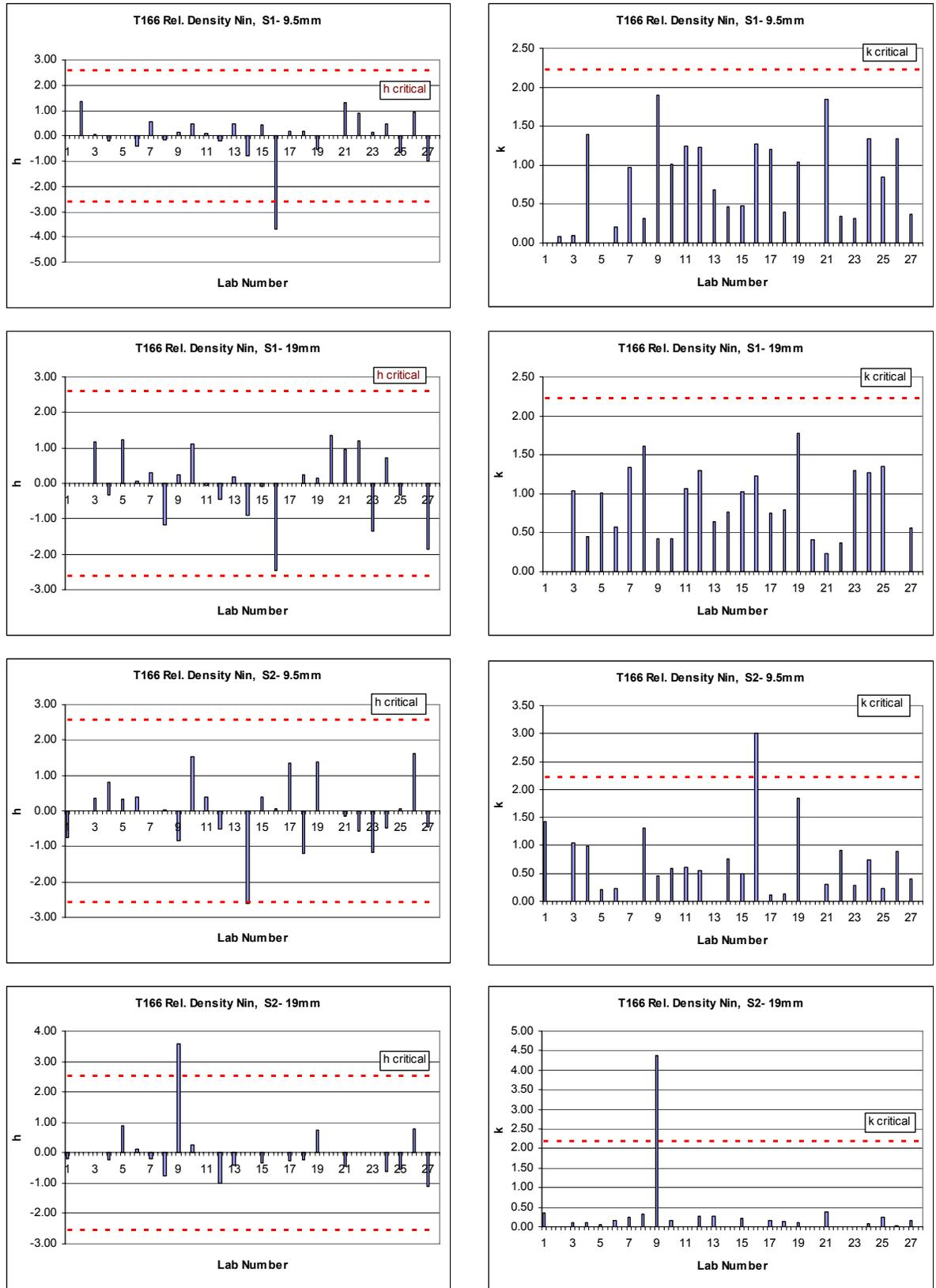
Figure 4-8- h and k consistency statistics of relative density at  $N_{in}$  using T166  $G_{mb}$ -T312
