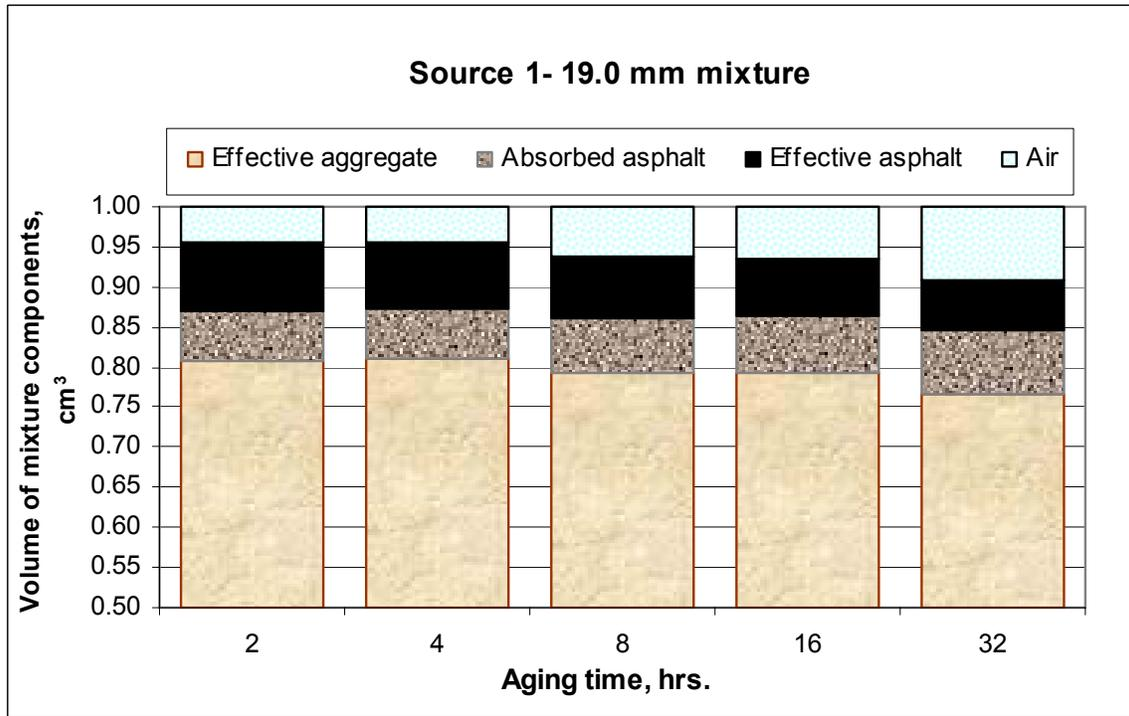
Figure 5-8- The volumetric component diagram of the S1-19-mm mixture at various aging times
