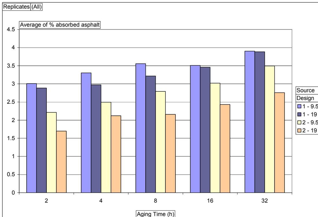
Figure 5-5- Average of % absorbed asphalt of the four mixtures at various aging times
