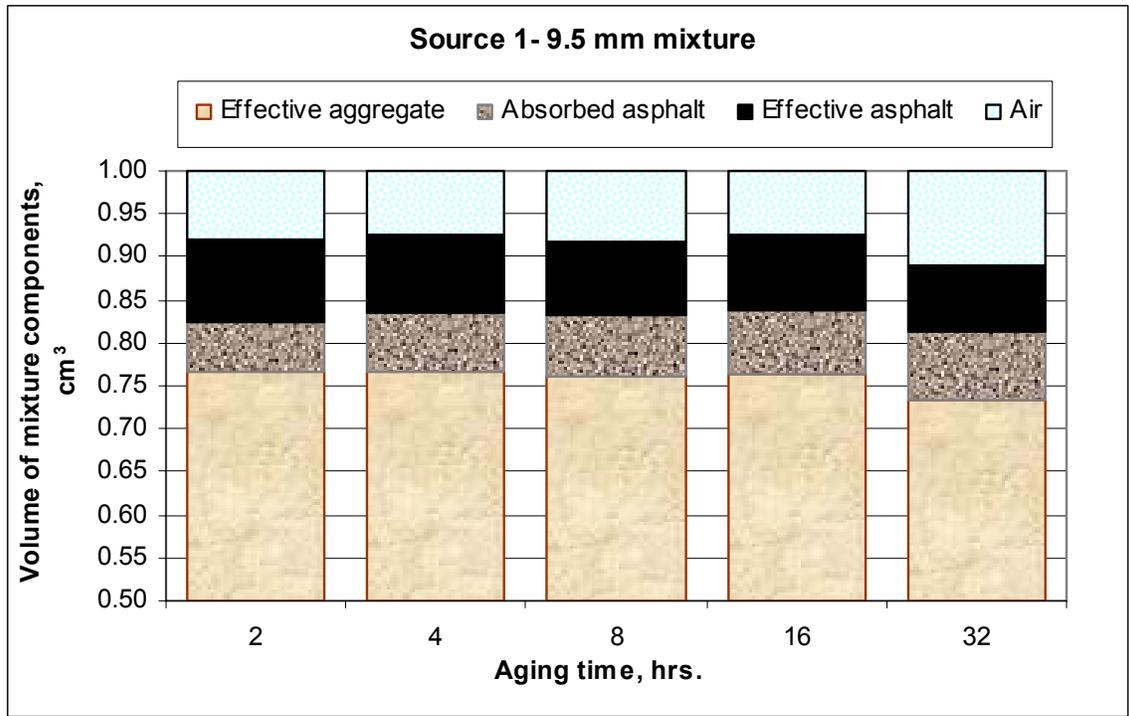
Figure 5-7- The volumetric component diagram of the S1-9.5-mm mixture at various aging times
