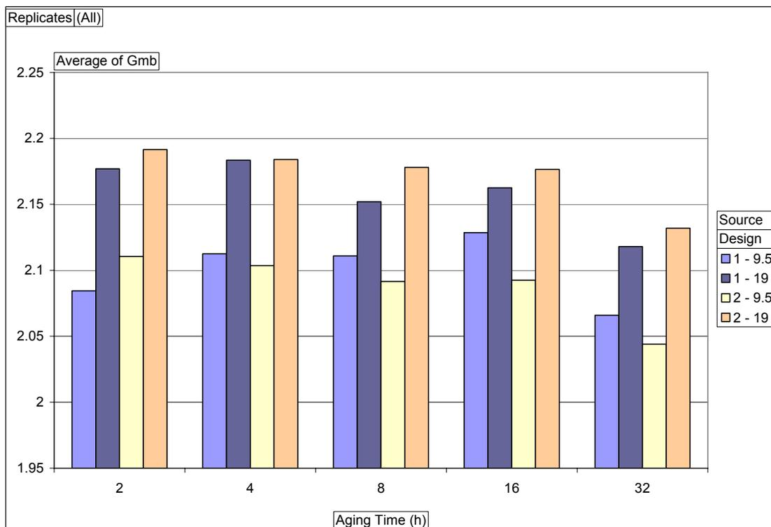
Figure 5-2- Average  $G_{mb}$  values of the four mixtures at various aging times
