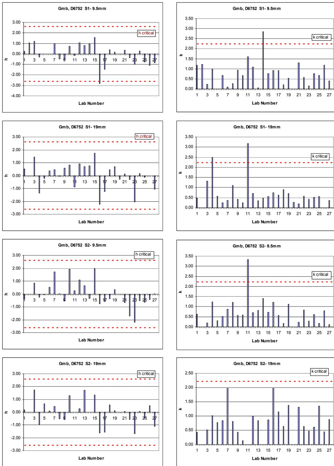
Figure 4-6- h and k consistency statistics of bulk specific gravity ( $G_{mb}$ )-D6752
