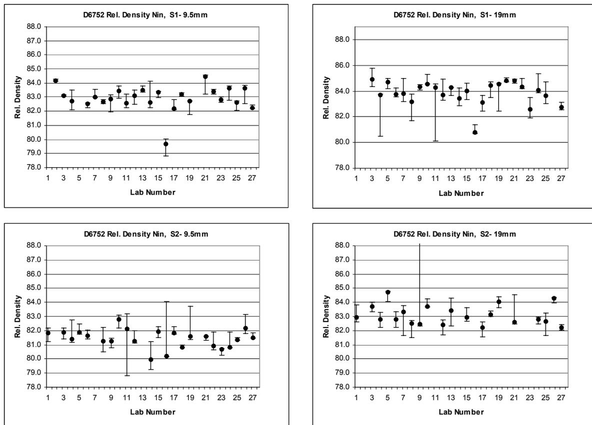
Figure 4-11- Box plots of relative density at  $N_{in}$  computed using D6752  $G_{mb}$  values-T312
