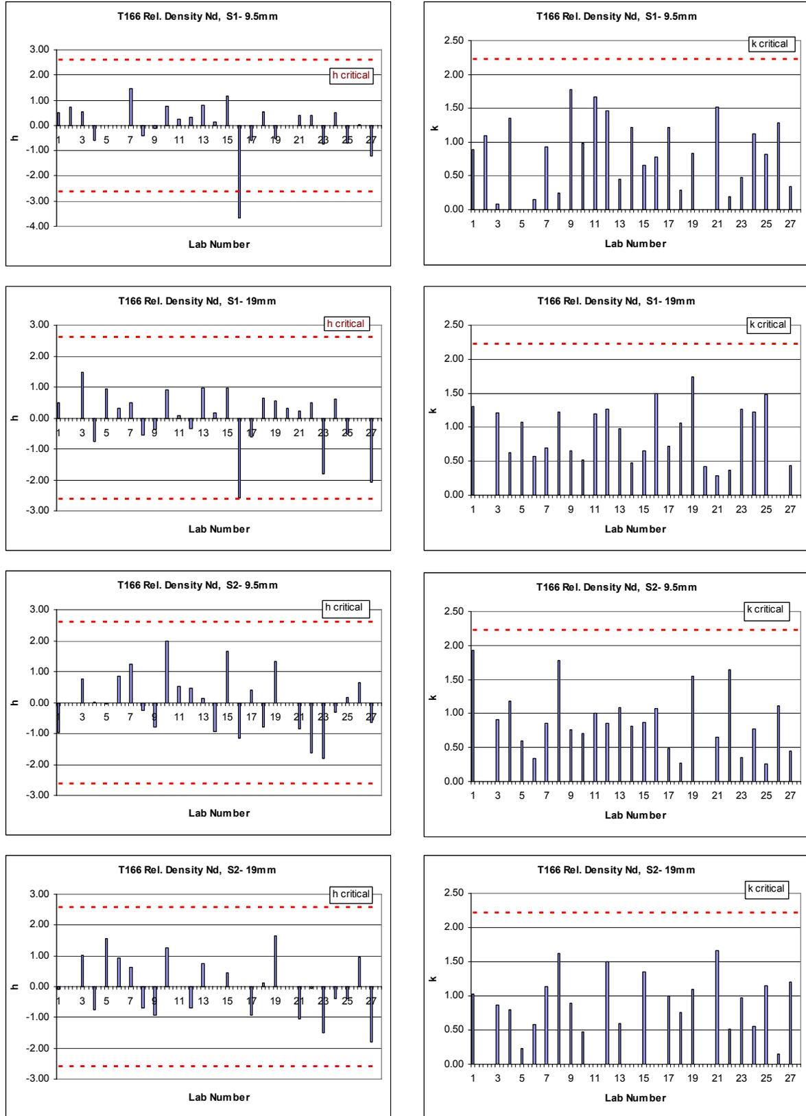
Figure 4-10- h and k consistency statistics of relative density at  $N_d$  using T166  $G_{mb}$ -T312
