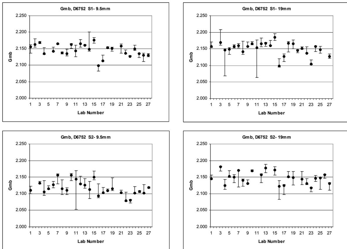
Figure 4-5- Box plots of bulk specific gravity ( $G_{mb}$ )-D6752
