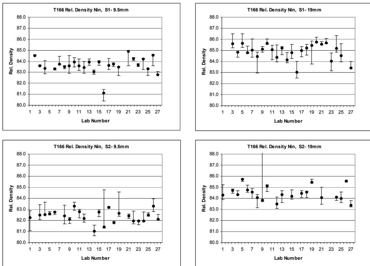
Figure 4-7- Box plots of relative density at  $N_{in}$  computed using T 166  $G_{mb}$  values-T312
