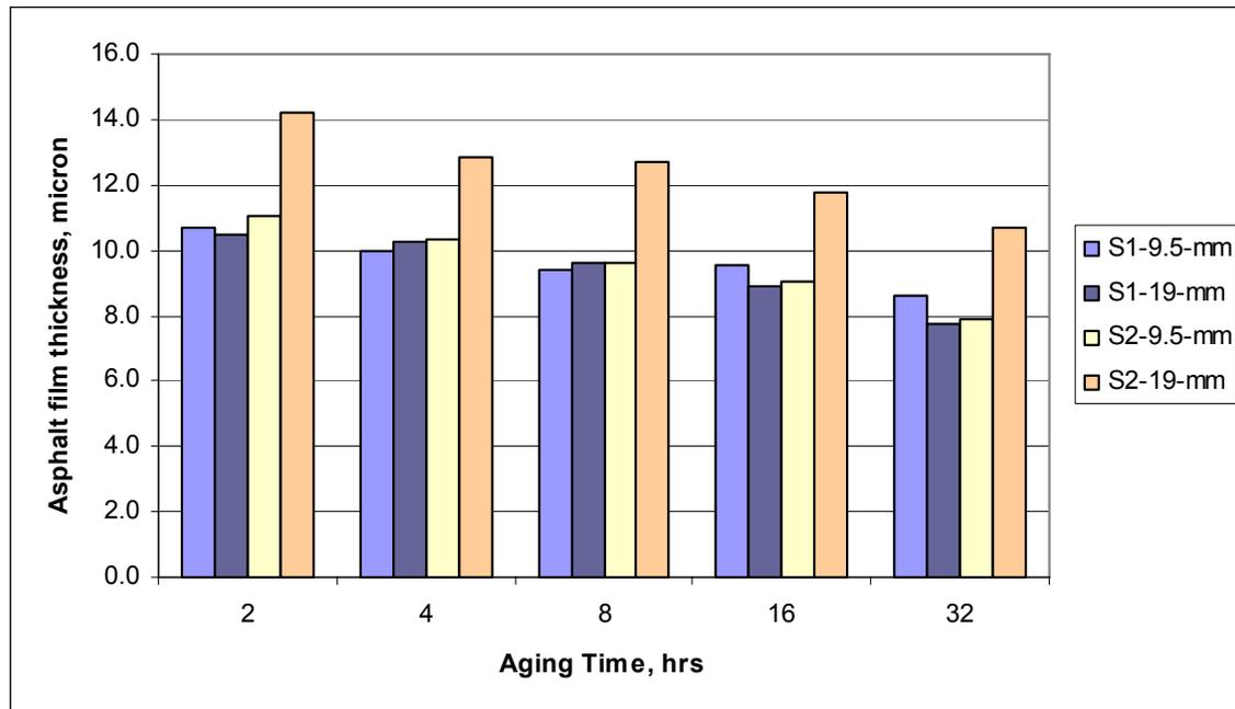
Figure 5-11- Asphalt film thickness in the four mixtures at various aging times
