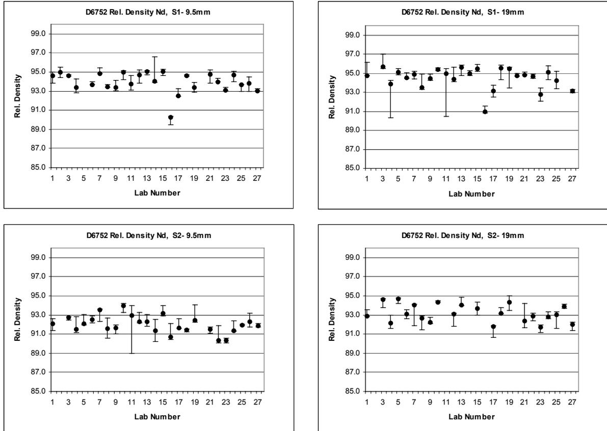
Figure 4-13- Box plots of relative density at  $N_d$  computed using D6752  $G_{mb}$  values-T312
