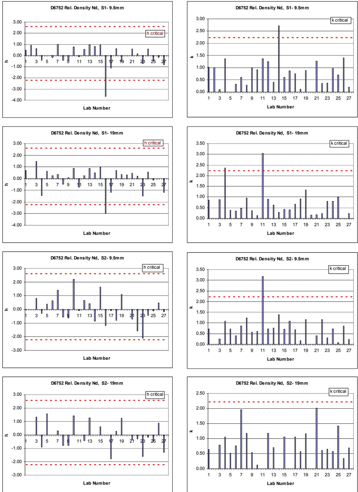
Figure 4-14- h and k consistency statistics of relative density at  $N_d$  using D6752  $G_{mb}$ -T312
