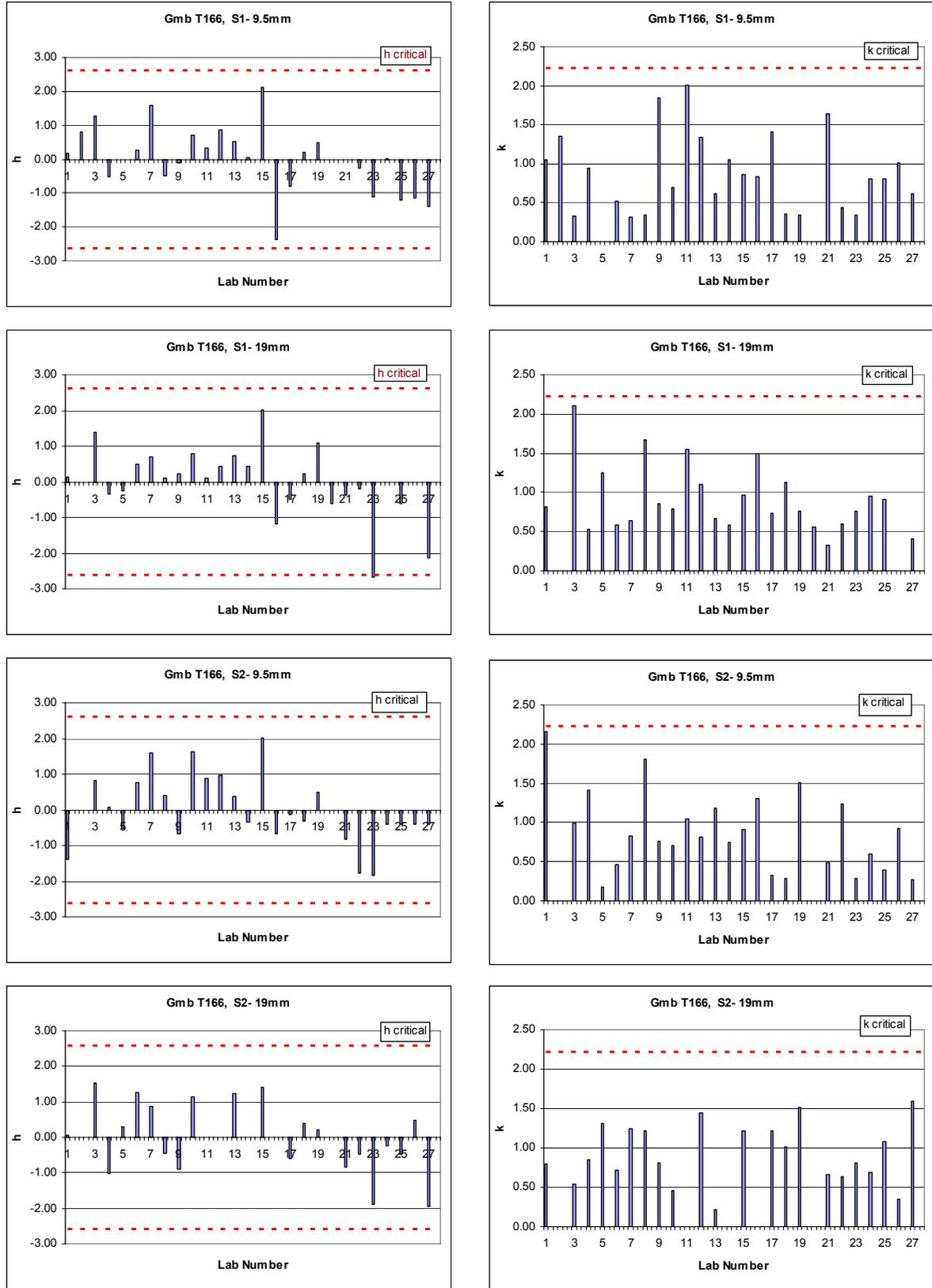
Figure 4-4- h and k consistency statistics of bulk specific gravity ( $G_{mb}$ )-T166
