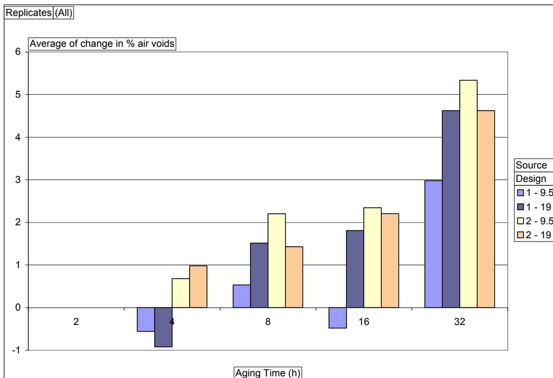
Figure 5-4- Average difference in % air voids of 2-hour and consequent aging times
