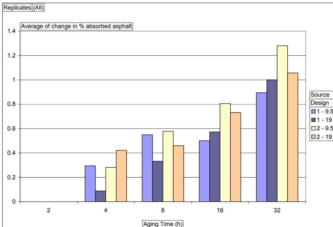
Figure 5-6- Average difference in % absorbed asphalt of 2-hour and consequent aging times
