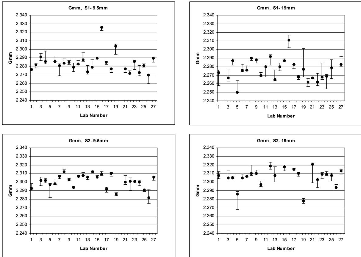
Figure 4-1- Box plots of maximum specific gravity ( $G_{mm}$ ) -D2041
