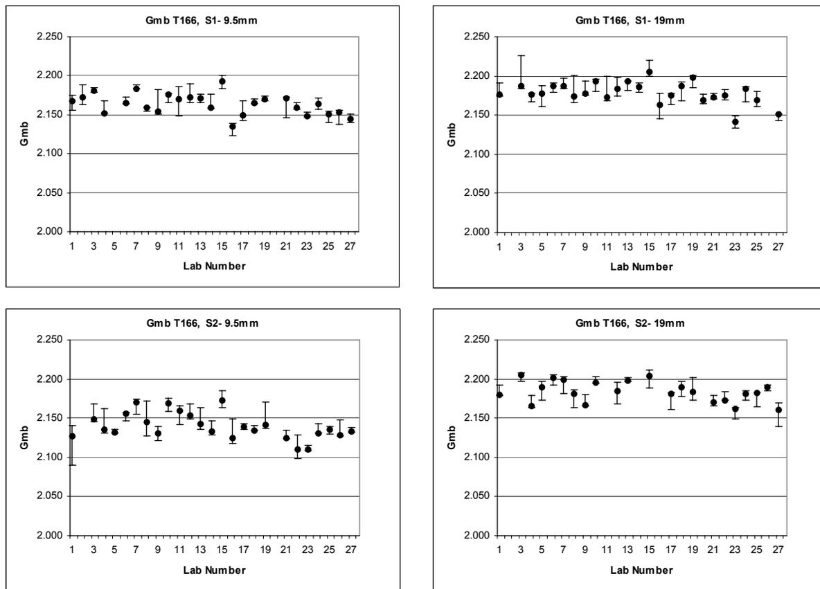
Figure 4-3- Box plots of bulk specific gravity ( $G_{mb}$ )-T166
