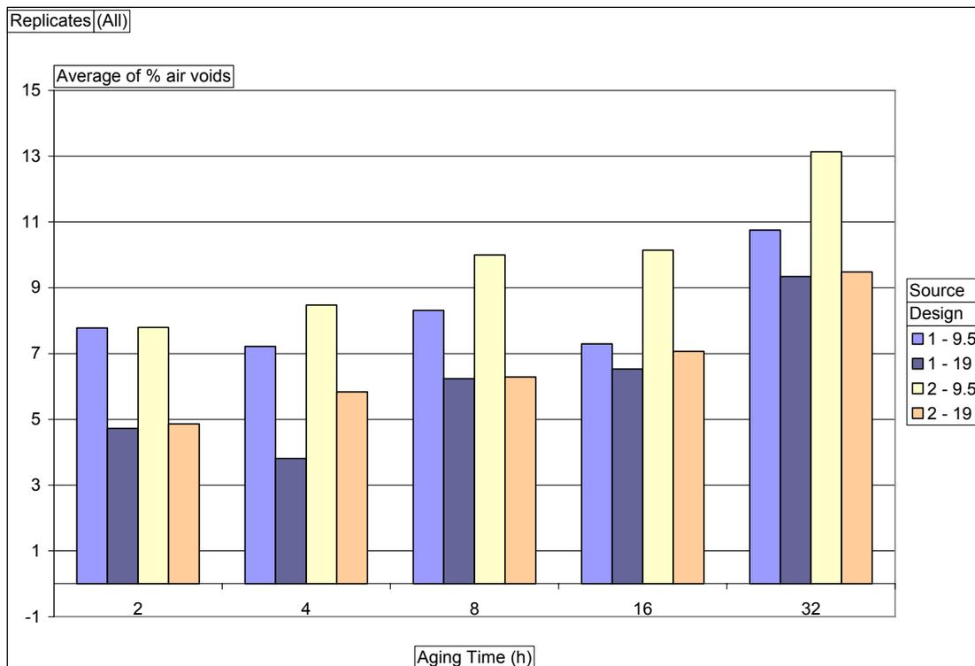
Figure 5-3- Average % air void values of the four mixtures at various aging times
