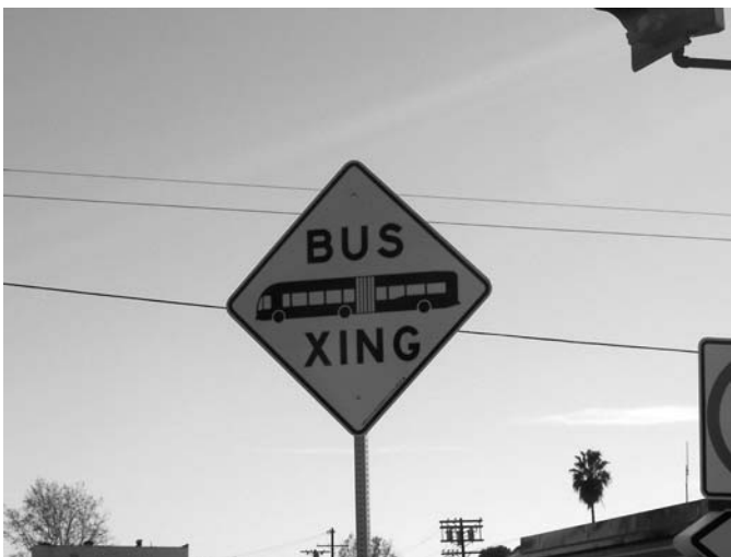
Figure 5-3. LADOT advance busway warning sign used at Orange Line intersections.
