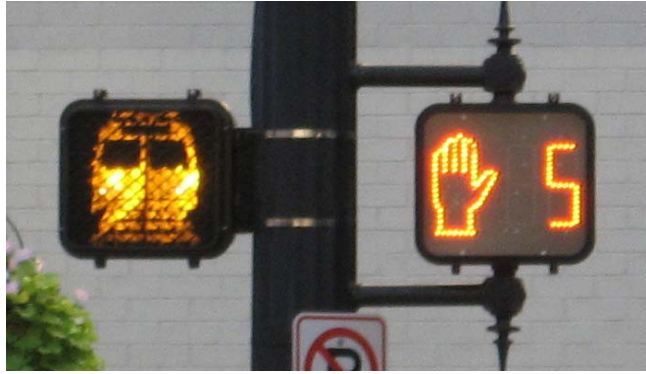
Figure 2 Visual train warning sign
