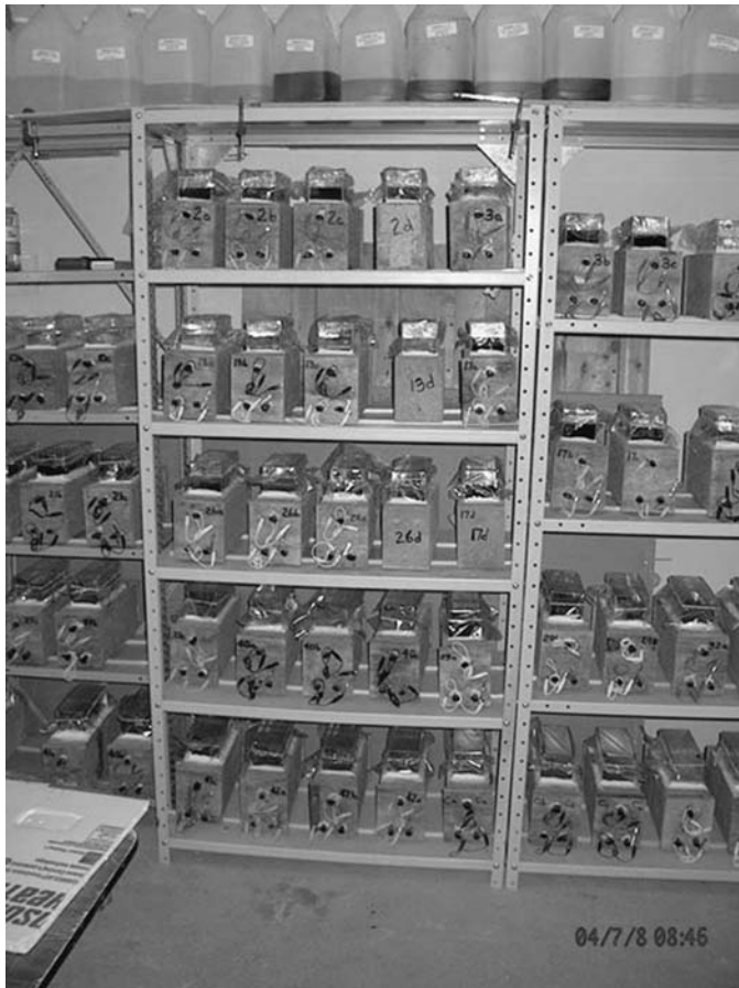
Figure 10-2. ASTM G 109 specimen setup.
