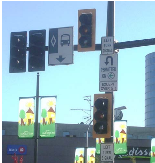
Figure G-8: Placement of Sign Permitting U-Turn
