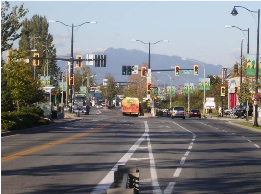
Figure G-3: Example of Painted Separation between Busway and General Purpose Traffic on Capstan Way Intersection Approach
