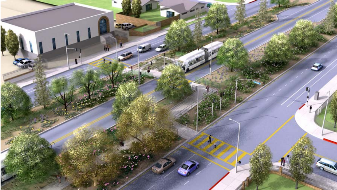
Figure D-1: Graphic Illustrating Zigzag Design at Pedestrian Crossings
