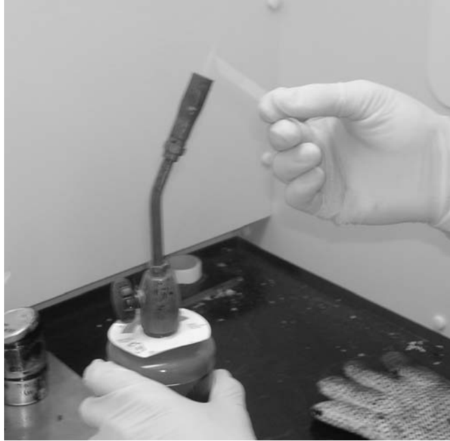
Figure 2 Glass slide dried before immersion by passing it over a propane flame.
