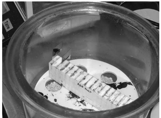
Figure 5 Finished slides stored on slotted holder in desiccator before testing.
