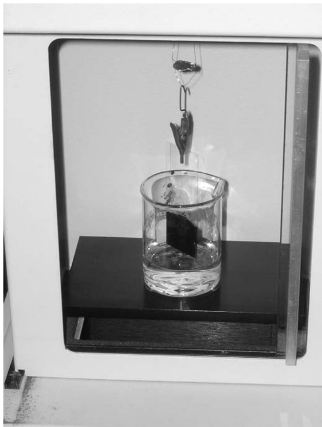
Figure 6 Asphalt binder sample suspended from microbalance for immersion in probe liquid.
