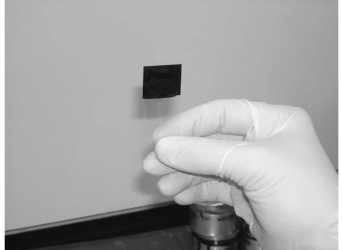
Figure 4 Glass slide coated with asphalt binder for testing with the Wilhelmy plate device.
