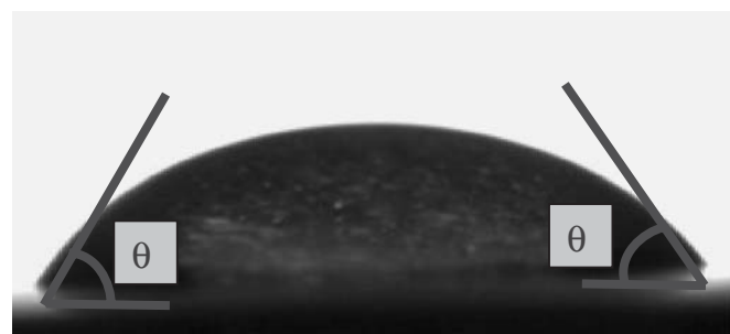
Figure 18 Typical image of sessile drop for contact angle measurement.
