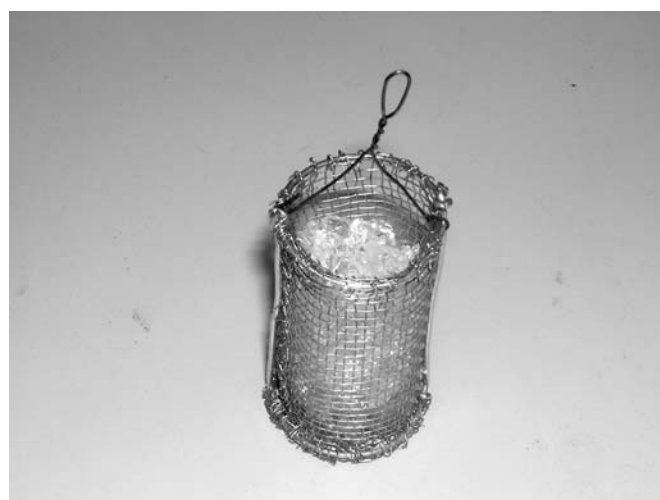
Figure 9 Basket with aggregate sample for testing with the USD.
