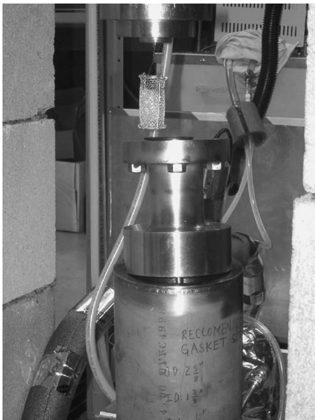
Figure 10 Sample basket suspended from the magnetic suspension balance.
