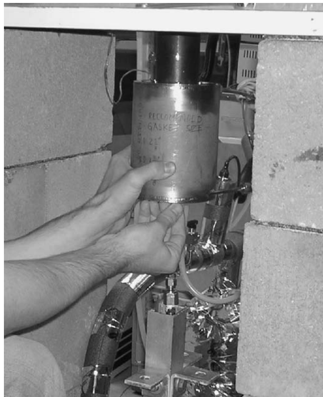
Figure 12 Temperature jacket raised to cover adsorption cell.
