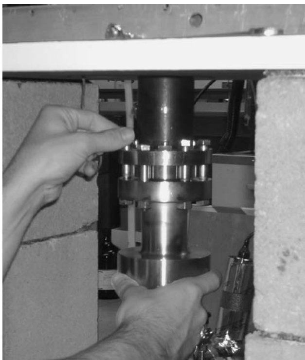
Figure 11 Adsorption cell raised and sealed with sample basket inside.
