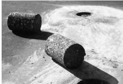
Pavement cores extracted from hot-mix asphalt sections at MnROAD.
