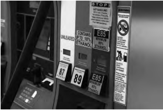
Gas pump in U.S. Midwest offers gasoline blends with up to 10 percent ethanol, as well as E-85, a mixture with up to 85 percent ethanol.
