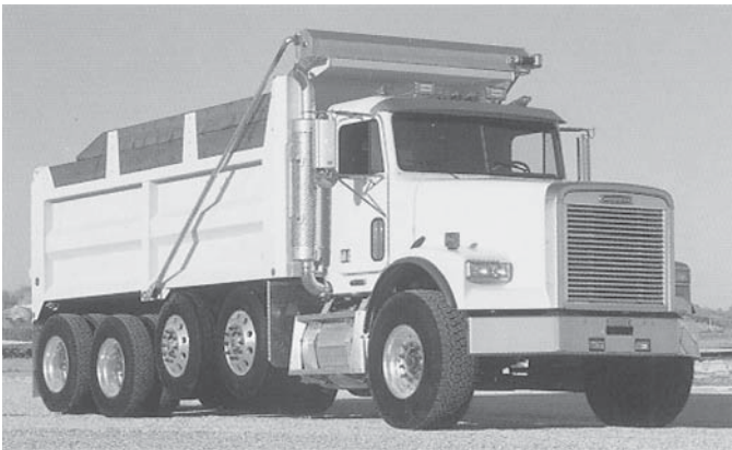
Figure 4. SHVs with liftable axles.
