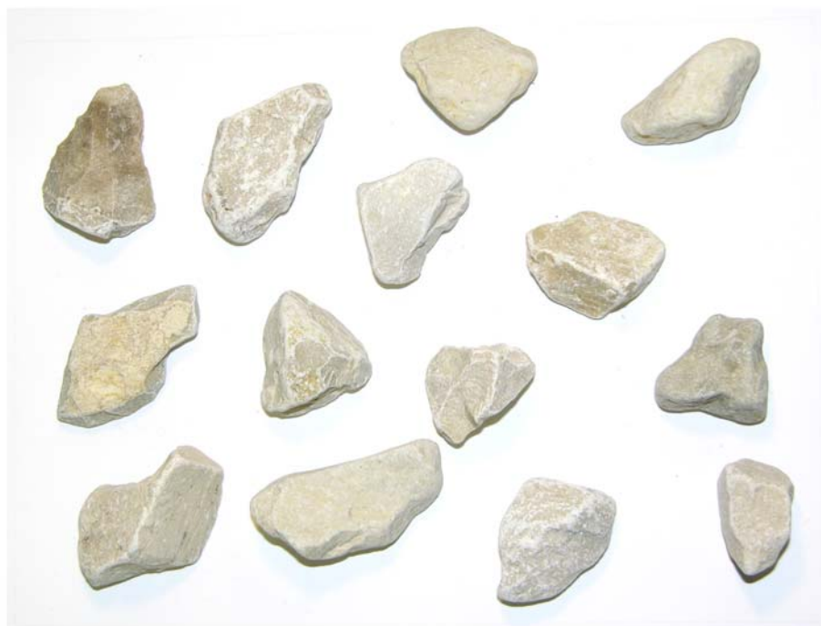
Aggregate 13 (3/4" [19.0 mm] - 1/2" [12.5 mm])
