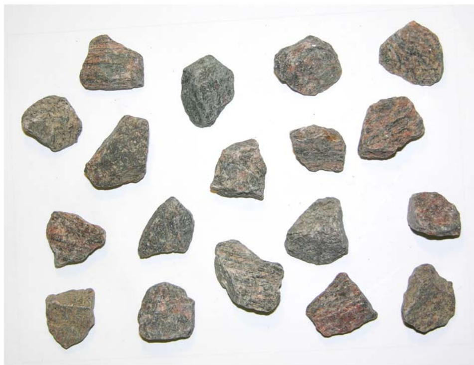
Aggregate 13 (3/4" [19.0 mm] - 1/2" [12.5 mm])
