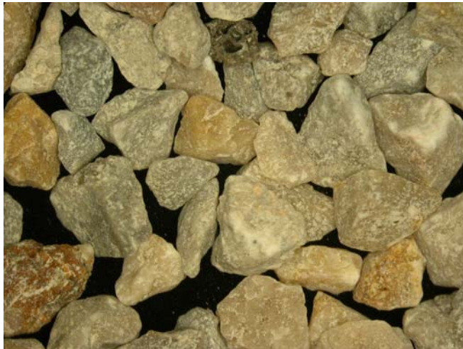
Aggregate 6 (#8 [2.36 mm] - #16 [1.18 mm])
