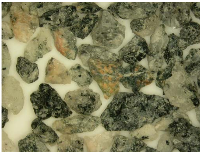
Aggregate 10 (#8 [2.36 mm] - #16 [1.18 mm])
