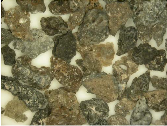
Aggregate 5 (#8 [2.36 mm] - #16 [1.18 mm])
