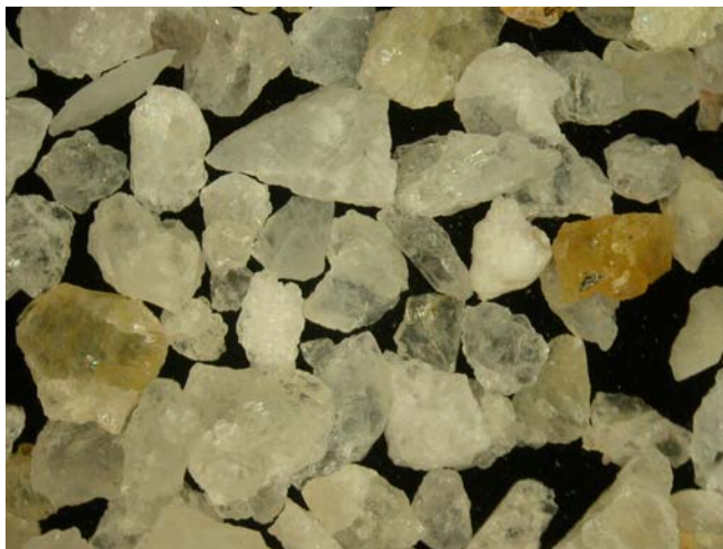
Aggregate 2 (#8 [2.36 mm] - #16 [1.18 mm])
