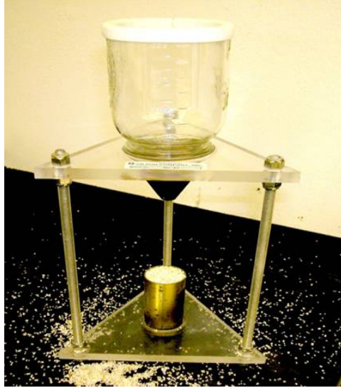
Figure D-1. Uncompacted Void Content of Fine Aggregate Apparatus.
