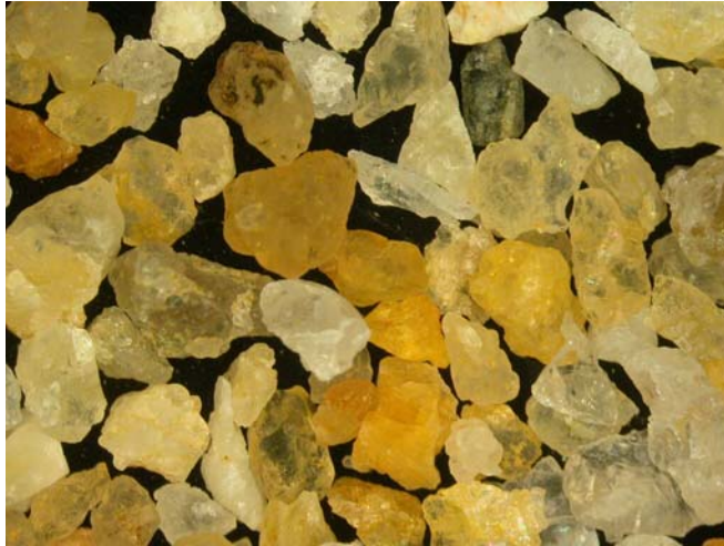
Aggregate 1 (#8 [2.36 mm] - #16 [1.18 mm])
