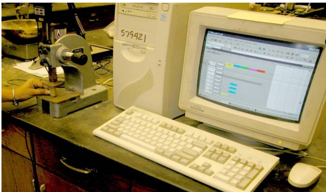
Figure D-10. Improved Digital Multiple Ratio Analysis Device (MRA) by Martin Marietta.
