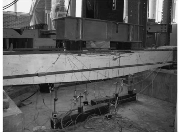
Figure 2-27. Beam tested under combined flexural and axial loading (10BA4).
