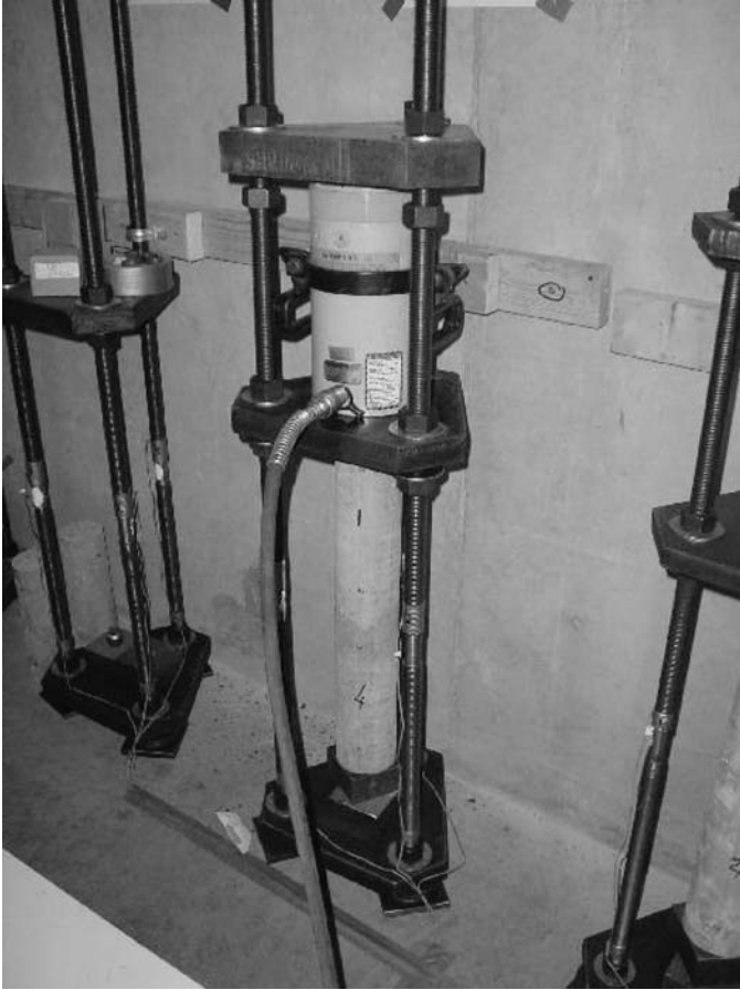
Figure 2-7. Test set-up for creep.
