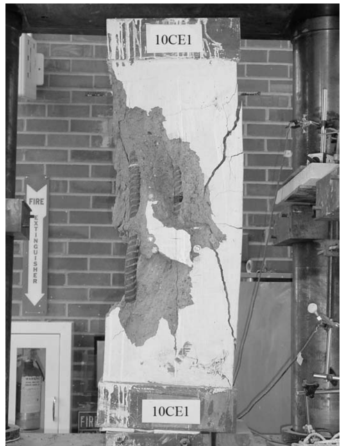
Figure 2-28. Rectangular column tested under small eccentricity (10CE1).
