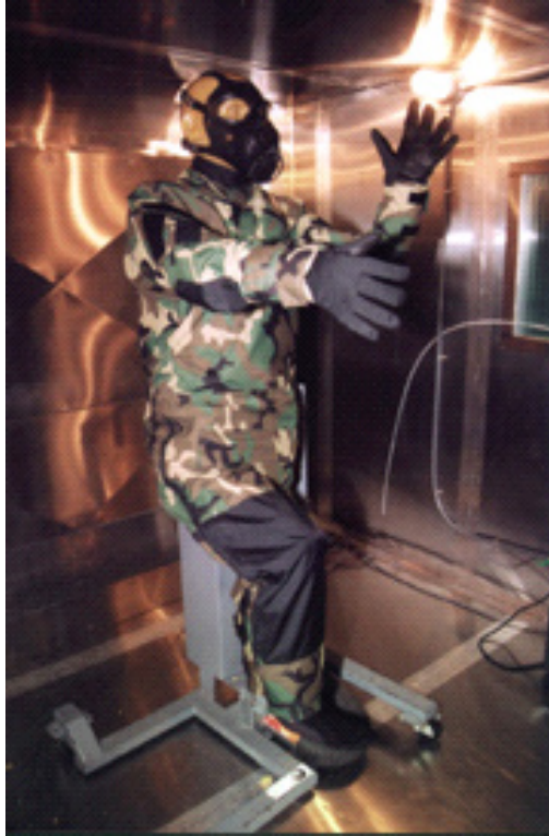
FIGURE 2.2 U.S. Army Soldier and Biological Chemical Command’s Paul mannequin cycling through motions in the Man-in-Simulant Test chamber. SOURCE: “Vapor chamber tests chem/bio protective prototypes” (photo by Curt Biberdorf), http://www.amc.army.mil/amc/pa/Aug02Issue.html . Accessed August 7, 2007.
