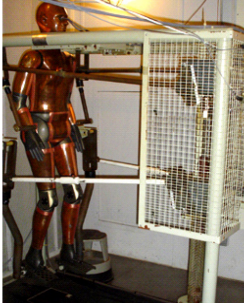
FIGURE 2.1 U.S. Army Research Institute of Environmental Medicine’s (USARIEM’s) Uncle Wiggly thermal mannequin in its own climate-controlled test chamber for measuring thermal and vapor resistance values of clothing ensembles.
