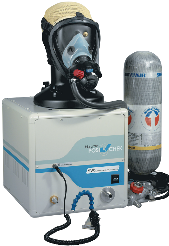
FIGURE 2.7 PosiChek 3 air-supplied breathing apparatus tester. SOURCE: Used with permission of Biosystems LLC, Middletown, Connecticut.
