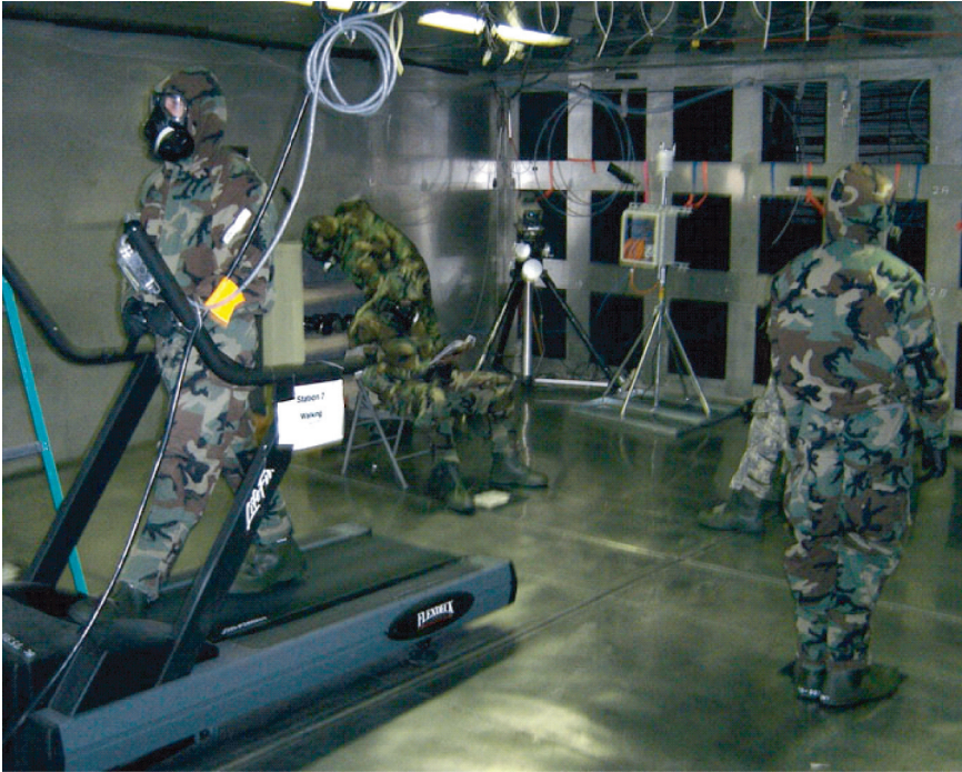
FIGURE S.1 Man-in-Simulant Test exercises in the chamber. The PETMAN system is required to perform the same set of exercises as the soldiers shown.
