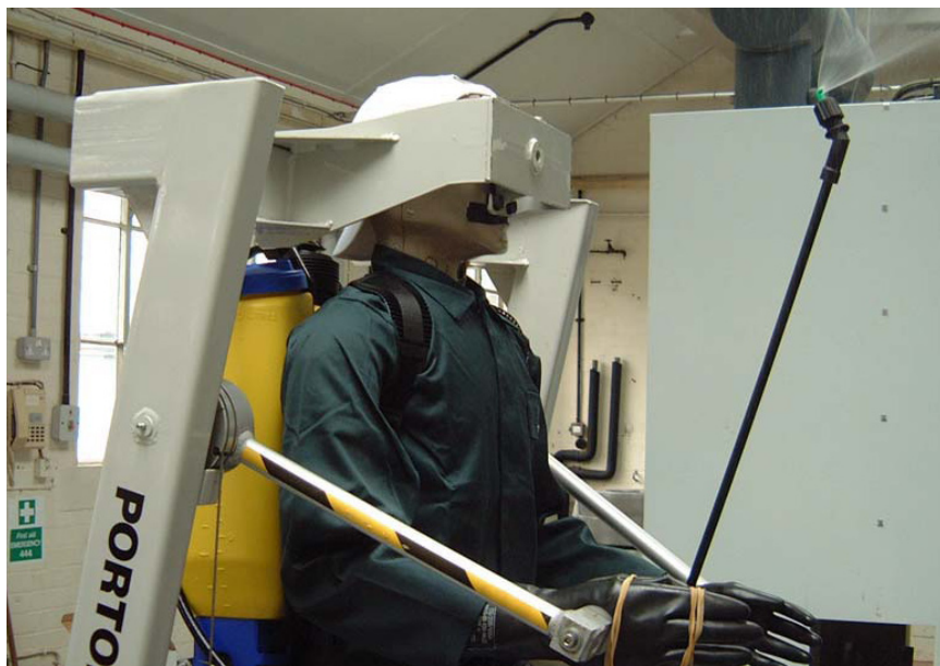
FIGURE 1.4 Portonman mannequin with knapsack sprayer in operation, simulating application of agricultural pesticides.
