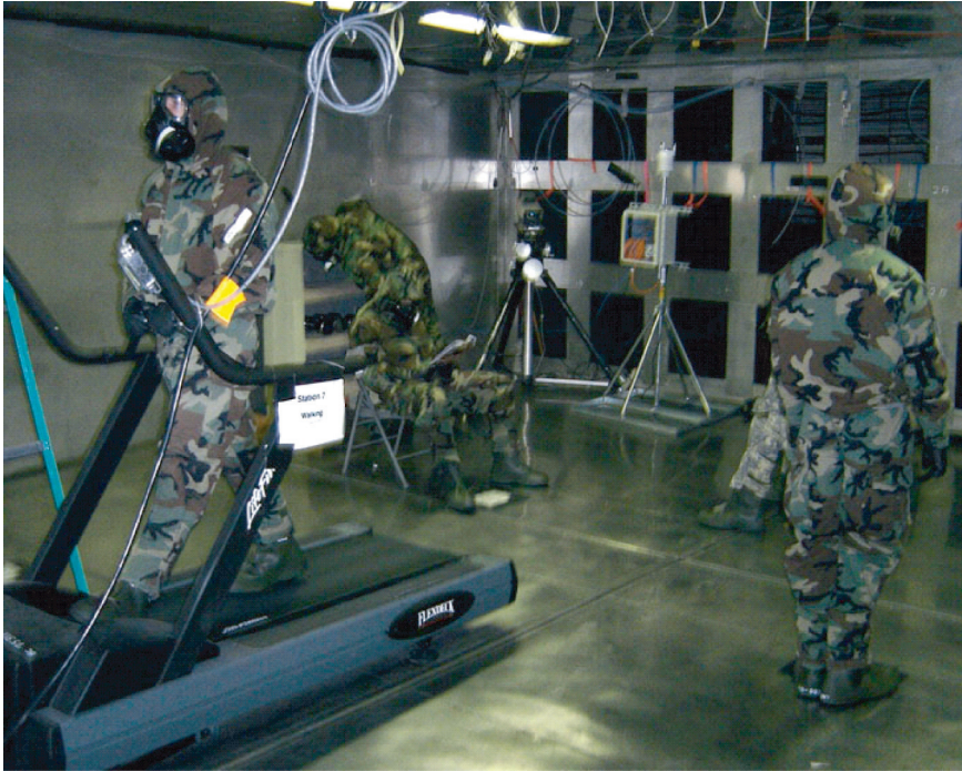
FIGURE 1.3 Man-in-Simulant Test exercises being performed in a chamber. SOURCE: Charles Walker, Dugway Proving Ground, U.S. Department of Defense.
