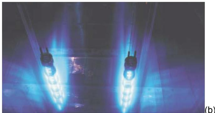
FIGURE 6-1 (a) An artist's rendition of an MDS Nordion JS-10000 panoramic irradiator, which uses a panel-type source rack (not necessarily to scale), and (b) a photograph of different source racks for an MDS Nordion Pallet Irradiator. SOURCE: Images courtesy of MDS Nordion (2002).
