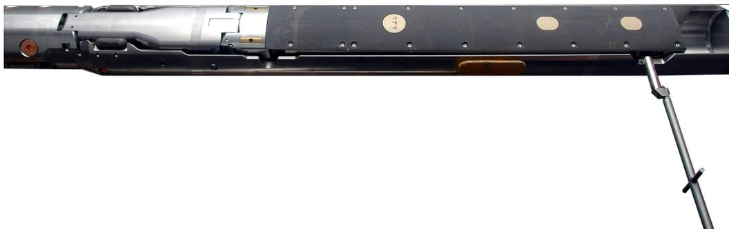
FIGURE 9-3 Atlas Densilog, which uses a vitrified cesium-137 source for wireline density measurements. The rod extending downward is a source handling device. The light-colored circles are windows for the source and detectors. SOURCE: Photo courtesy of Baker Hughes Inc.
