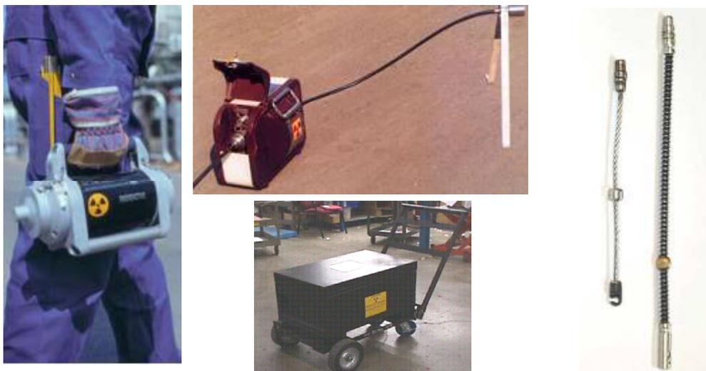
FIGURE 8-3 Radiography cameras. Note that the hand-held device is an iridium-192 radiography camera, as is the sealed source mounted on the end of the cable shown to the right. The device on wheels is a cobalt-60 radiography camera. SOURCE: Images provided by the committee.
