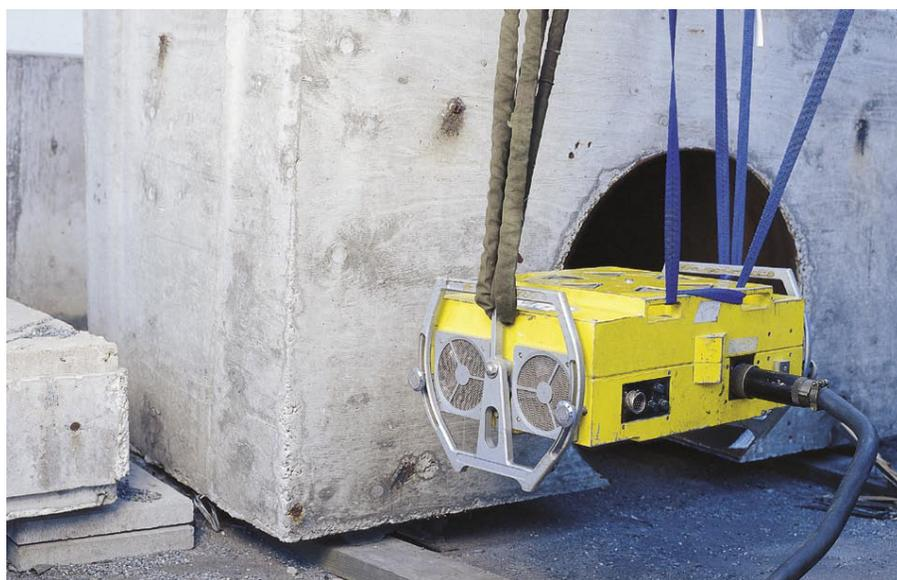
FIGURE 8-5 Photograph of an Inspecta betatron particle accelerator hanging in a harness and used for nondestructive examination. The x-ray energy can be varied from 2 MeV up to 6 MeV, which allows the radiographer to examine thick sections of steel or concrete. SOURCE: Copyright Inspecta.
