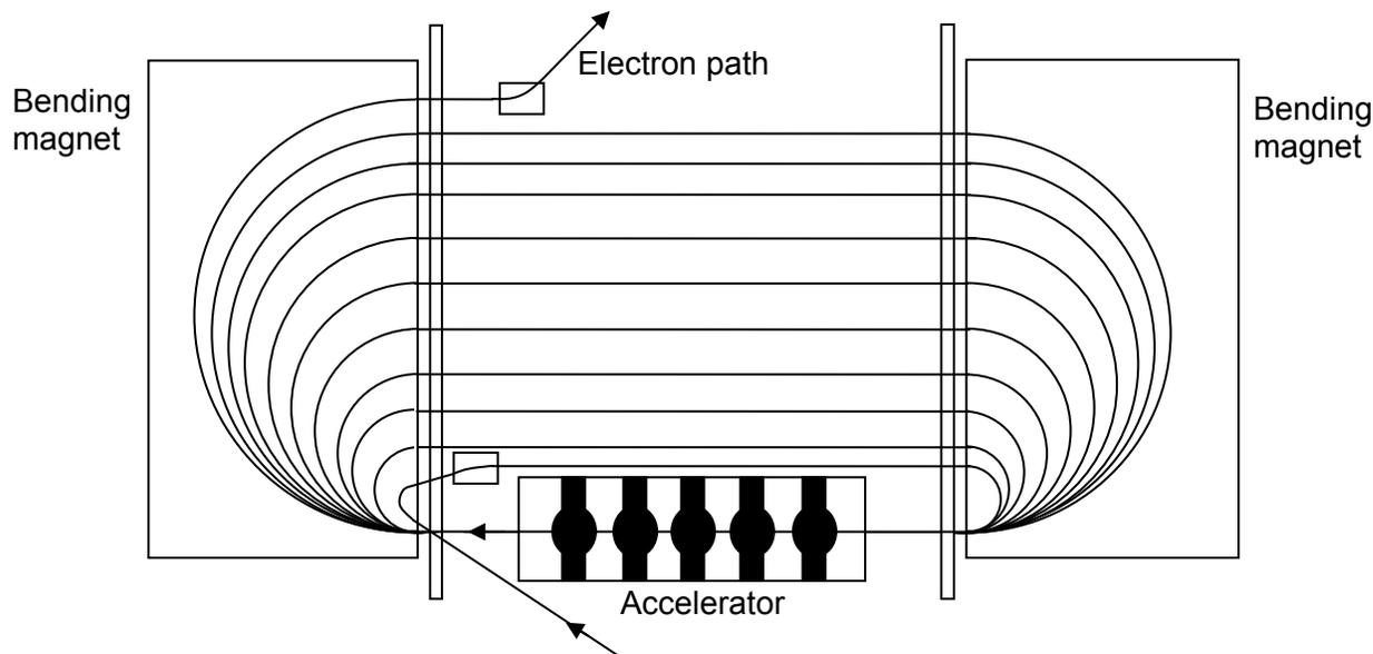
FIGURE 4-6 Diagram of a microtron. SOURCE: Image provided by the committee.
