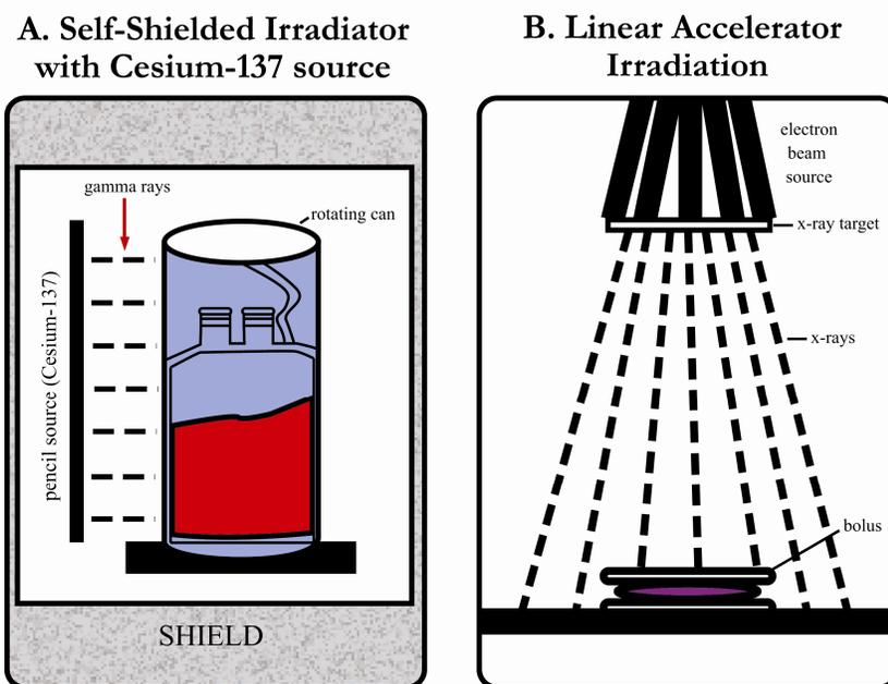
FIGURE 5-2 Diagrams of (A) a configuration of a gamma irradiator using cesium-137 and (B) a configuration of a linac irradiator. The plastic bolus is a container that enhances the dose uniformity in the irradiation configuration shown. SOURCE: Image provided by the committee.
