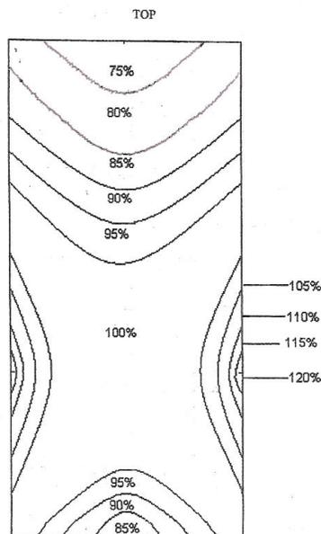
FIGURE 5-4 Typical dose map in a blood irradiation canister. SOURCE: Unpublished data on isodose curve in percentages for Gammacell 1000, provided by the American Red Cross, 2007.
