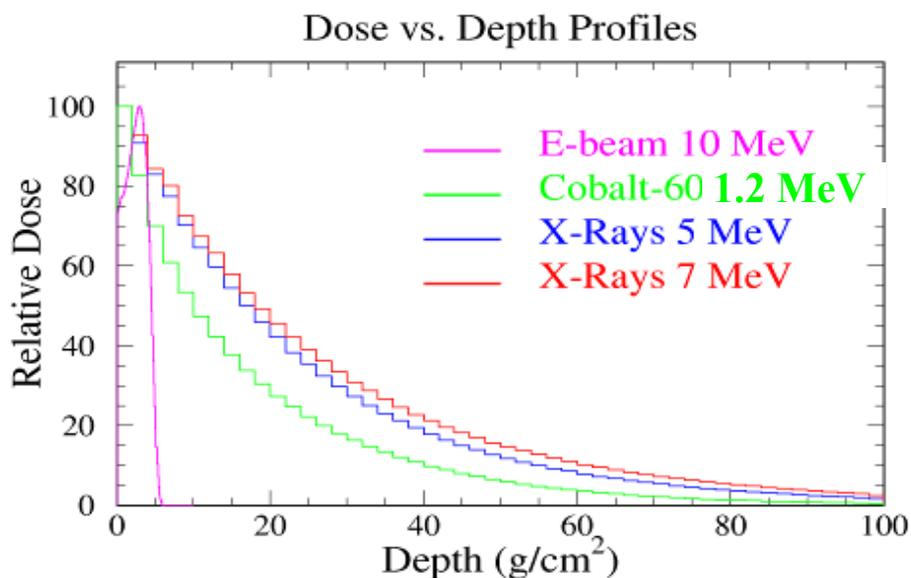
FIGURE 6-3 Relative dose versus depth in material for four different radiations. The highest relative dose for all depth values greater than 5 g/cm<sup>2</sup> is the 7-MeV x-ray. The 5-MeV x-ray is just below that, and the cobalt-60 curve is next. The e-beam curve drops to zero relative dose at about 6 g/cm<sup>2</sup>. SOURCE: Image courtesy of Cleland, M. (2006).
