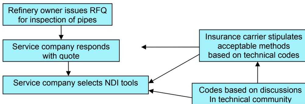
FIGURE 8-4 Process for selecting nondestructive testing method on the left, and factors that influence or dictate the process on the right. NOTE: RFQ = Request for quote. SOURCE: Provided by committee.
