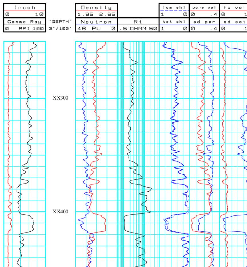
FIGURE 9-1 Typical logs and evaluation results from a string of well logging tools, including a natural gamma-ray log, a neutron log, an array induction log, and resistivity logs. The hydrocarbon volume result is also shown at the right. SOURCE: van Popta et al. (2004), courtesy of the Society of Petrophysicists and Well Log Analysts.
