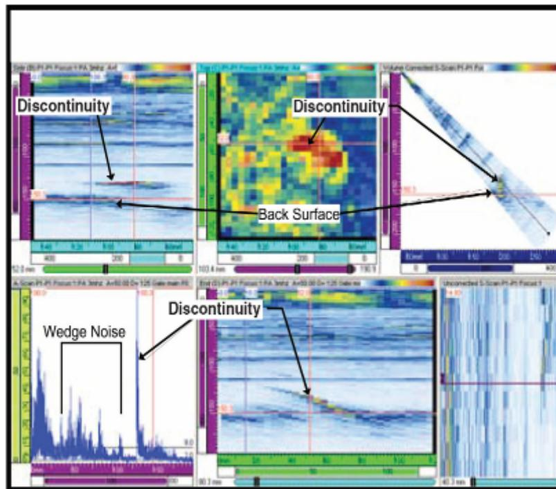
FIGURE 8-7 (a) Radiograph of a metal tube inside another larger metal tube. (b) Typical output from ultrasonic testing (of a different component) illustrating six panels of information obtained from the same component. SOURCE: (a) Blettner, A., et al. (2000), (b) Crech, M. (2006).
