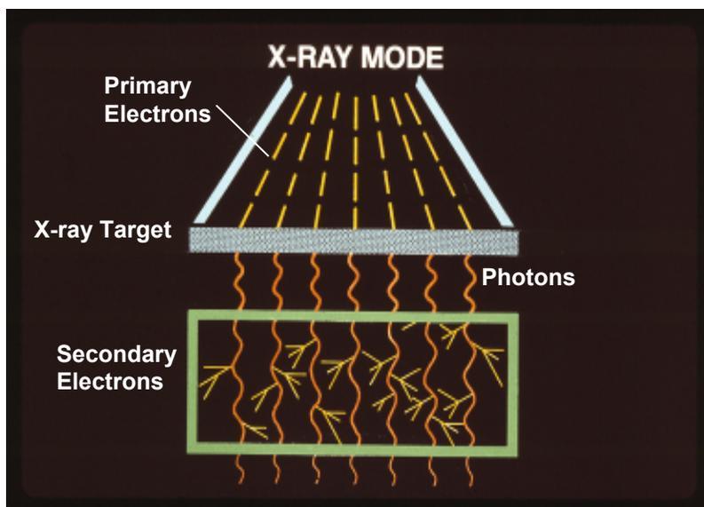
FIGURE 6-4 X-ray irradiation. SOURCE: Image courtesy of Cleland, M. (2006).
