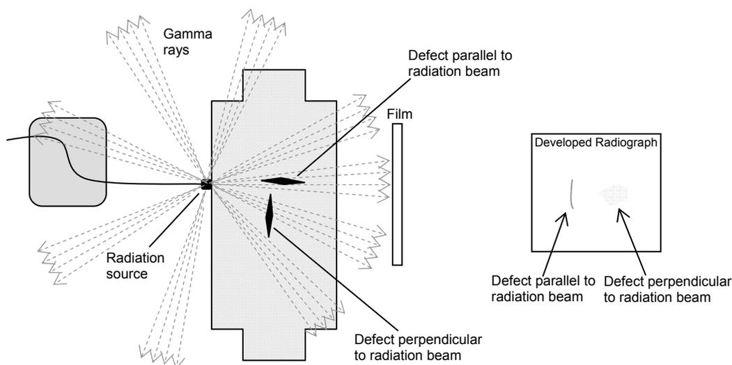
FIGURE 8-6 Cartoon of radiographic examination of a component with a parallel defect. SOURCE: Image provided by committee.
