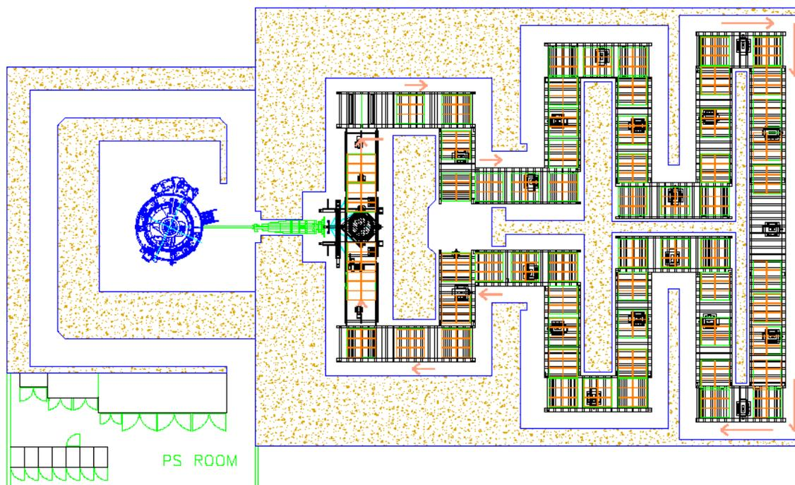
FIGURE 6-5 Conceptual plan view of an x-ray irradiator using the IBA Rhodotron for the electron beam and the Palletron for handling the products. SOURCE: Image courtesy of Cleland, M. (2006).
