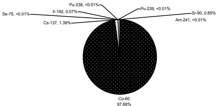
FIGURE 2-4 Share of total activity in radiation sources in the United States by radionuclide. SOURCE: Constructed with data from U.S. NRC (2007a).
