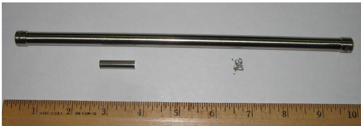
FIGURE 2-1 Typical cobalt-59 pencil and slug, which is irradiated to make industrial cobalt-60 sources. Also shown is a pile of cobalt-59 pellets, which can be irradiated in a high-flux reactor to make cobalt-60 teletherapy and industrial radiography sources. The ruler uses English units (1 inch = 2.54 cm). SOURCE: Image provided by committee.
