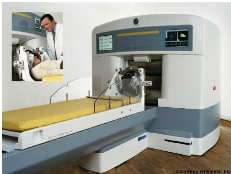
FIGURE 7-4 A Gamma Knife<sup>®</sup> installation showing the main body of the unit containing 201 cobalt sources (at 30 Ci = 1.11 TBq each source), the treatment couch, and a collimator helmet attached to the treatment couch. The inset shows an up-close image of the automatic positioning system used to position the patient for treatment. SOURCE: Image courtesy of Elekta.
