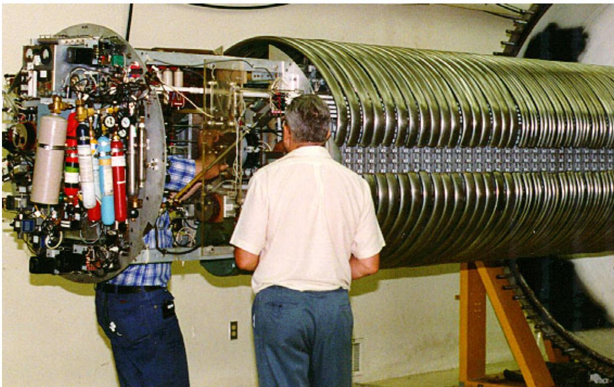
FIGURE 4-4 A Dynamitron showing the accelerator column. SOURCE: Image courtesy of ION Beam Laboratory, State University of New York at Albany.
