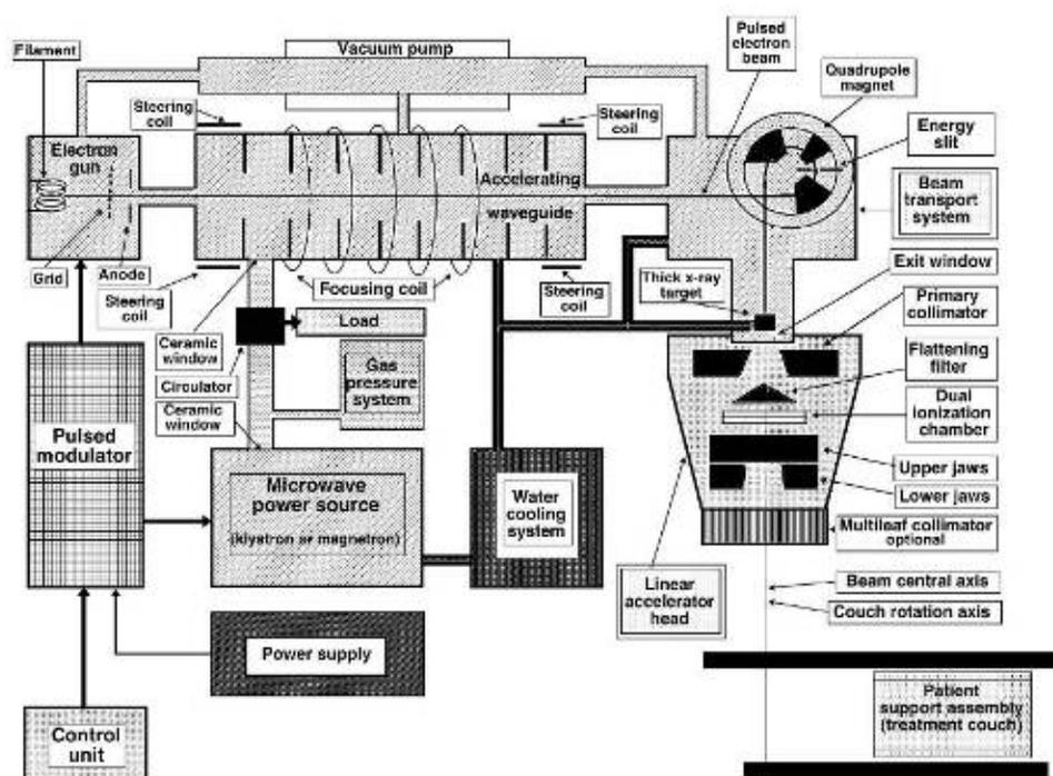
FIGURE 4-1 Schematic diagram of a typical medical electron accelerator with x-ray conversion target. SOURCE: Image provided by committee.
