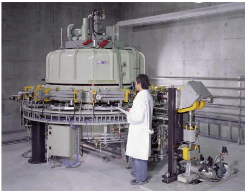
FIGURE 4-7 This 200-kW Rhodotron is used to irradiate U.S. mail at a facility in New Jersey. SOURCE: Image courtesy of IBA-RDI.
