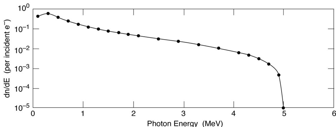
FIGURE 4-3 Bremsstrahlung x-ray (photon) energy spectrum from a 5-MeV electron beam. The ordinate (vertical axis),  $dn/dE$ , shows the number of x-rays within a certain energy range per incident 5-MeV electron. SOURCE: Image provided by the committee.
