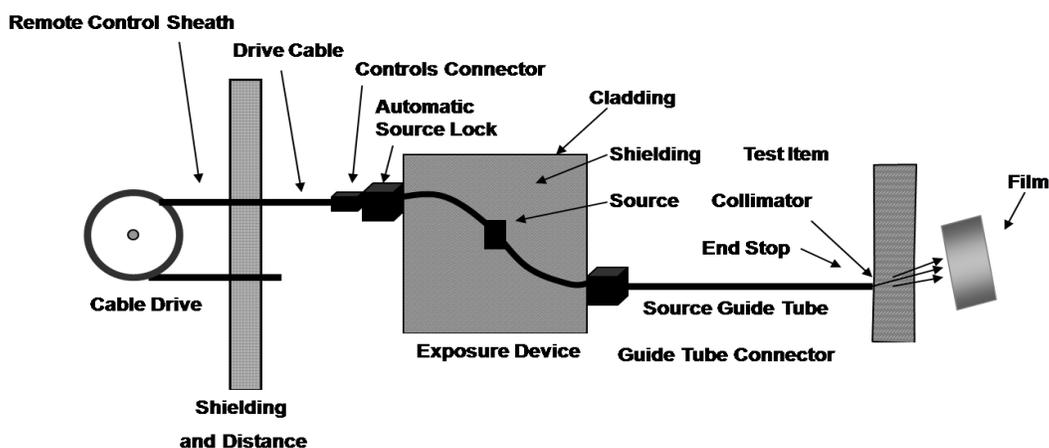
FIGURE 8-1 Schematic of the internals of a portable, hand-held radiography camera. Such a system typically uses iridium-192 as the gamma source. SOURCE: Image provided by the committee.
