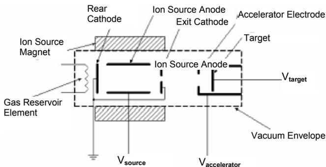
FIGURE 4-10 Schematic of a neutron tube. SOURCE: Image courtesy of Burkhart, B. (2006).
