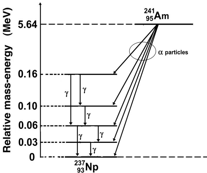
FIGURE B-5 Decay scheme for the alpha decay of americium-241 into neptunium-237 with a half-life of 432 years. A spectrum consisting of five discrete alpha particle energies is emitted and the alpha particles produce neptunium-237 in four excited states in addition to the ground state. All excited states instantaneously decay through various excited states into the ground state of neptunium-237 through emission of gamma photons. SOURCE: Image provided by committee.
