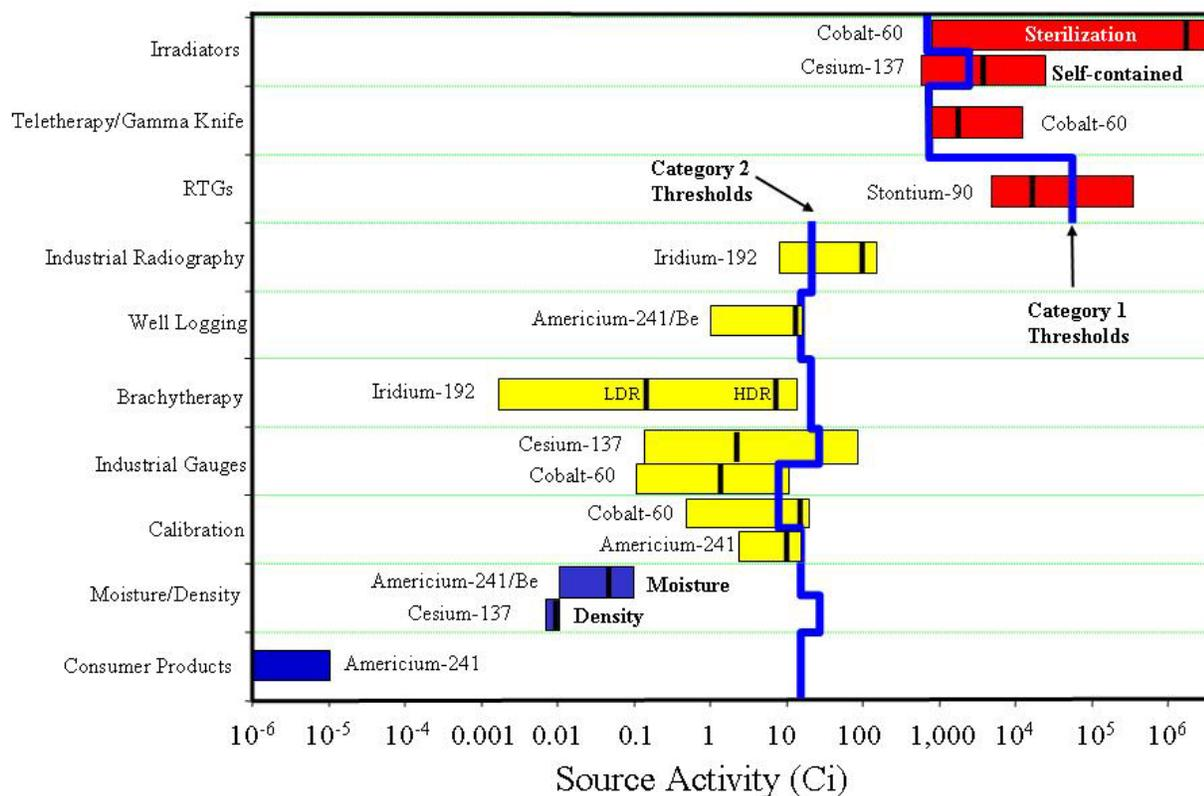
FIGURE 3-3 Radiation source applications, radionuclides, and activity ranges. NOTE: 1 Ci = 0.037 TBq. SOURCE: Modified from IAEA (2005a).
