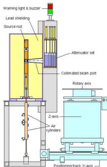
FIGURE 5-7 Typical gamma calibrator configuration for survey instrument calibration. SOURCE: Image provided by Hopewell Designs, Inc. (2007).
