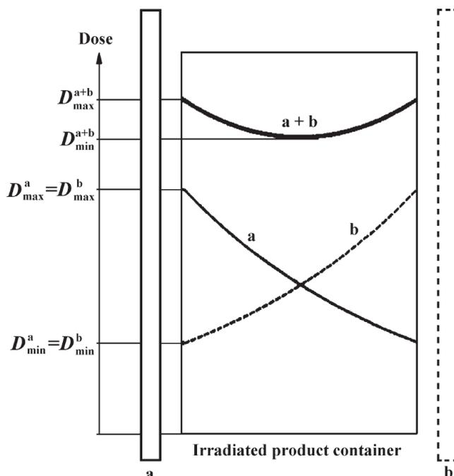
FIGURE 6-6 Depth-dose distribution in a product container irradiated from opposing sides with a cobalt-60 source. Curve a represents the depth-dose distribution when the product is irradiated by a source rack in position a. Curve b is for the source rack in position b. Curve a + b shows the sum of doses from irradiation on both sides. SOURCE: Image courtesy of IAEA (2004b).
