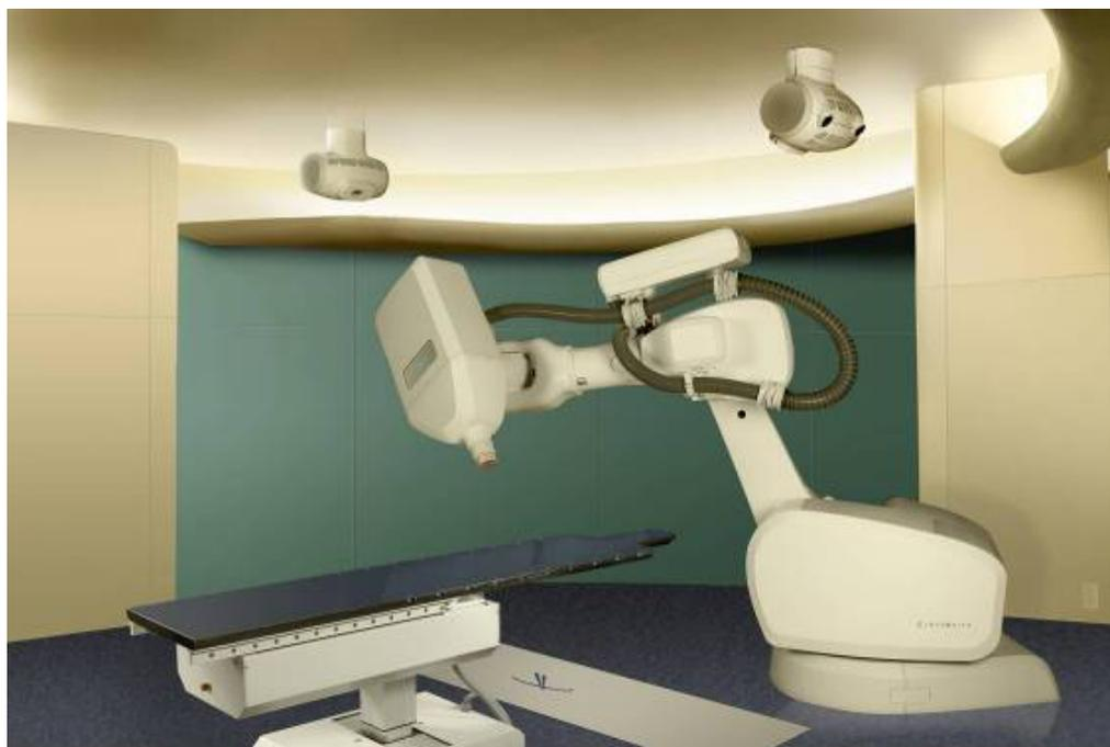
FIGURE 7-7 CyberKnife® installation consisting of miniature linac mounted on a robotic arm, treatment couch, and imaging device: ceiling-mounted x-ray tubes and floor-mounted image intensifiers. SOURCE: Image courtesy of Accuray, Sunnyvale, CA.
