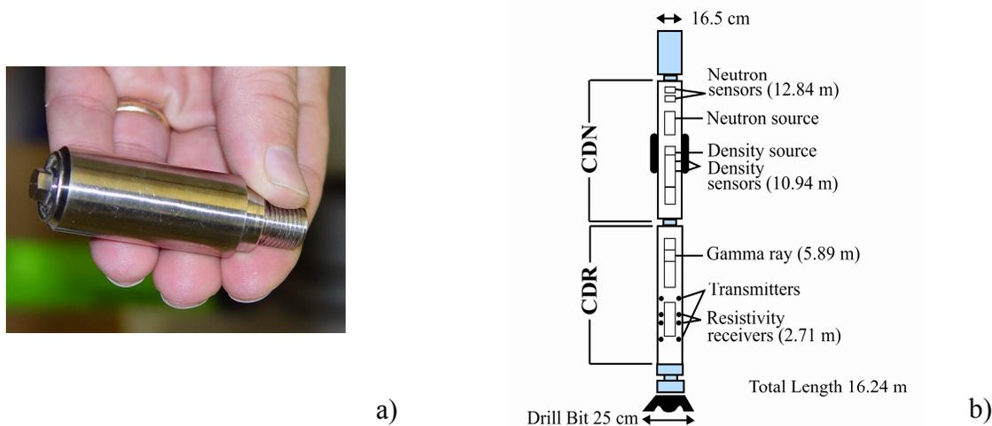
FIGURE 9-2 Photograph of an Am-Be neutron source used in well logging (a) and a diagram of a sonde mounted on a drill for logging while drilling (b). SOURCE: (a) Image courtesy of Sandia National Laboratory (William Rhodes, III), (b) Provided by the committee.
