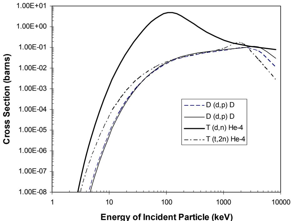
FIGURE 4-9 Fusion reaction cross sections as functions of kinetic energy. SOURCE: Image provided by the committee.
