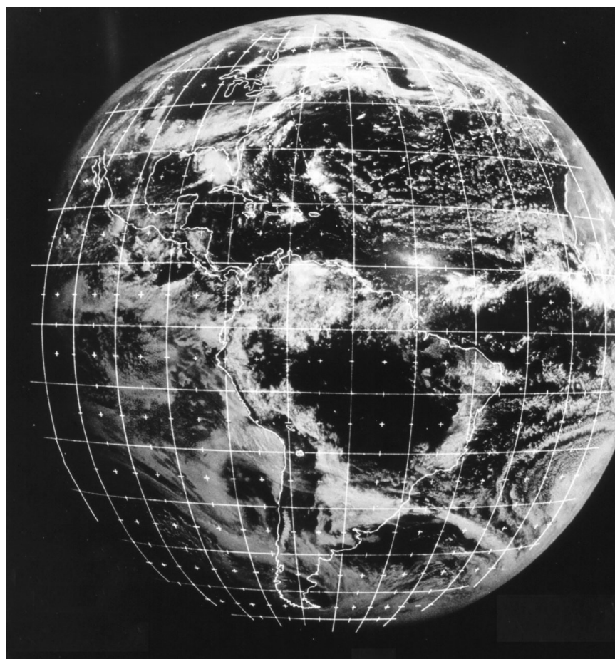
FIGURE 3.4 Example of the hemispheric coverage of a geostationary satellite. Taken by NASA's Applications Technology Satellite 3 (ATS 3) at 1402 UTC on July 21, 1970. Note that Tropical Storm Becky can be seen in the Gulf of Mexico near Florida. SOURCE: NOAA Photo Library.
