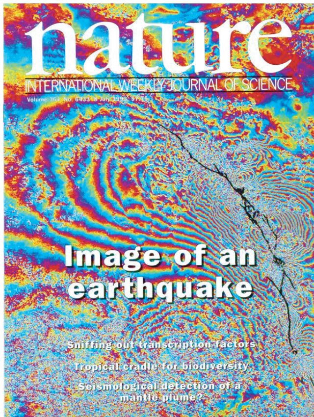
FIGURE 11.4 Cover of the journal Nature showing the first-ever image of an earthquake. This interferogram was produced by combining the pair of ERS-1 SAR images taken before and after the Landers earthquake of June 28, 1992. Each cycle of colored shading represents a range difference of 28 mm between the before and after images, used to detect changes in the position of the ground surface. SOURCE: Massonnet et al. (1993). Reprinted with permission from Macmillan Publishers Ltd., copyright 1993.
