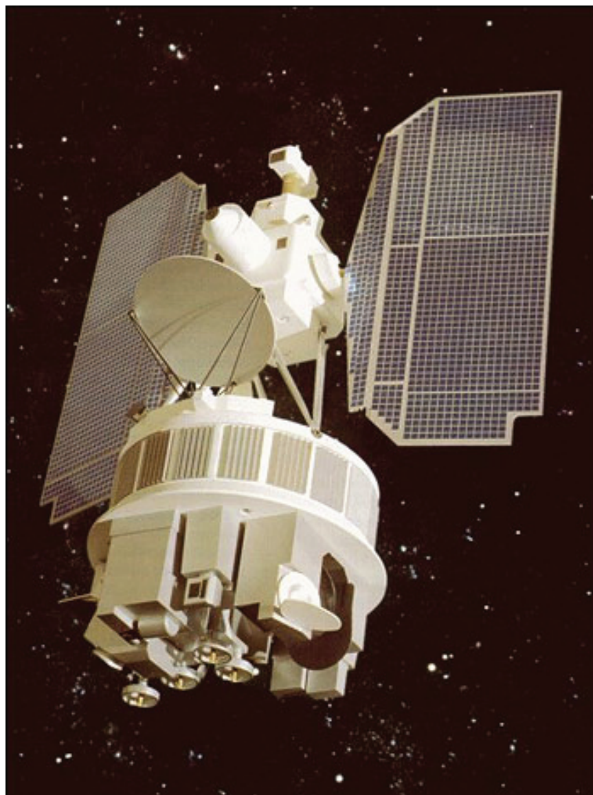
FIGURE 2.9 Artist's drawing of the general design of the Nimbus series of satellites. SOURCE: C. R. Madrid, ed. (1978). The Nimbus 7 Users' Guide , Goddard Space Flight Center, NASA.
