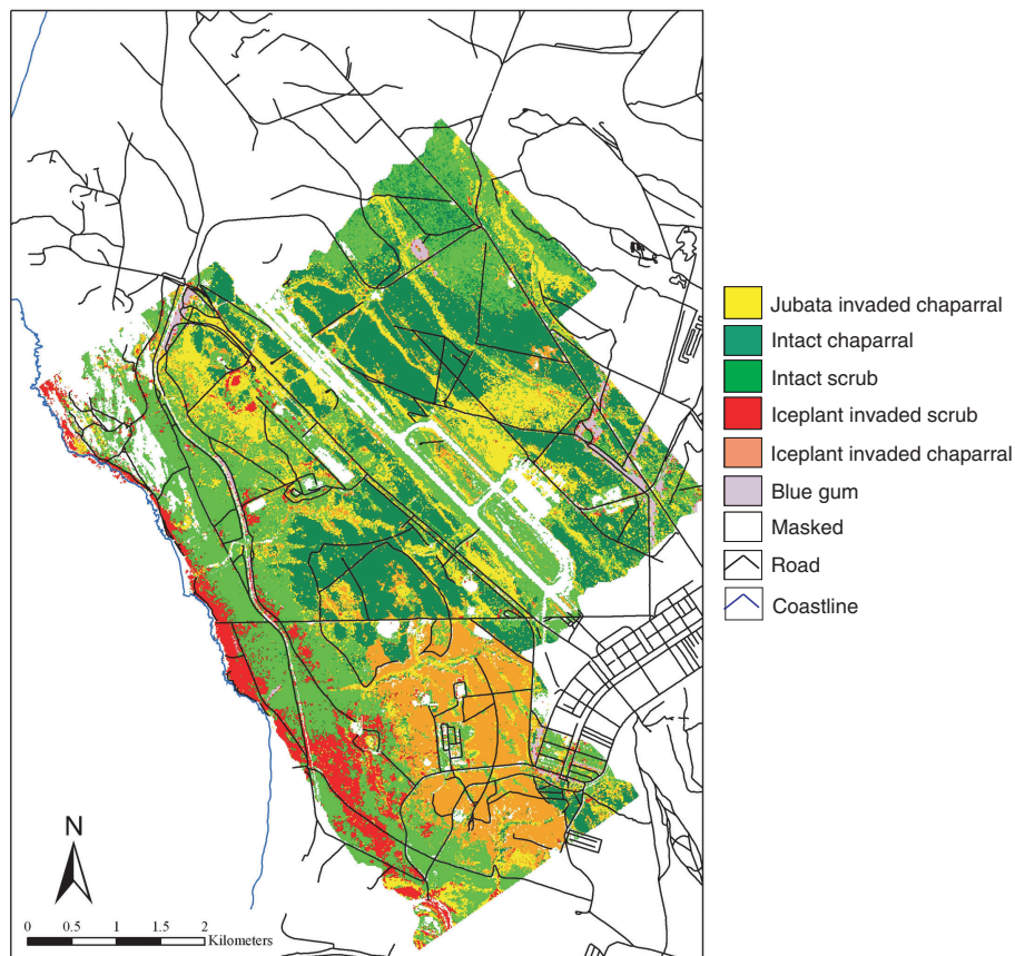
FIGURE 9.7 Distribution of three invasive species—iceplant, jubata grass, and blue gum—in two native shrub ecosystems—coastal sage scrub and Burton Mesa chaparral—on the central coast of California. The map was produced from a mosaic of flightlines acquired from airborne NASA AVIRIS data, a 224-band imaging spectrometer measuring from the visible through the solar infrared (400-2,500 nm) and measured at a nominal 3-m pixel resolution. SOURCE: Underwood et al. (2006). Reprinted with kind permission of Springer Science and Business Media, copyright 2006.
