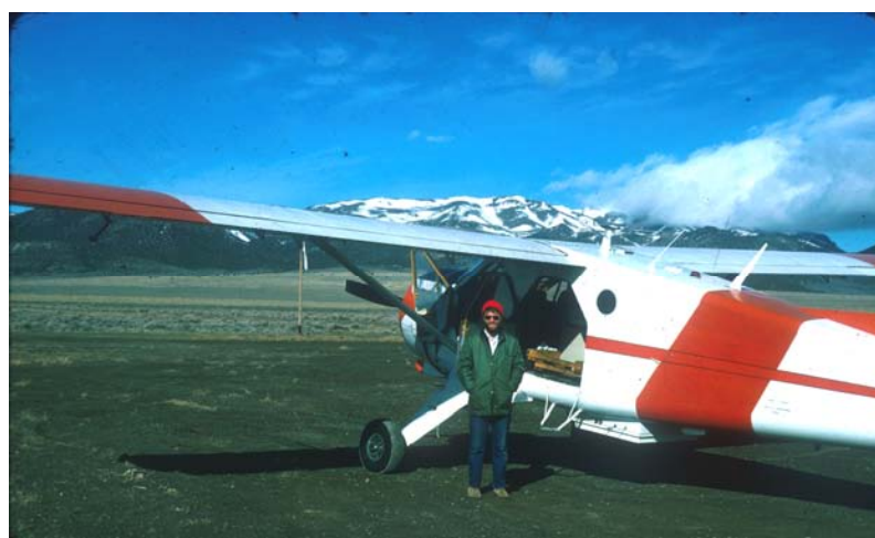
FIGURE 2-9 High-end and low-end airborne sensing. (a) A Lockheed C-130 airplane, extensively modified by NASA for use as a research platform and supporting a wide variety of onboard sensors, including multispectral scanners, radiometers, air sampling equipment, and aerial cameras. SOURCE: Available online (b) A de Havilland Canada Beaver configured for airborne geophysics in the 1970s. The primary instrument was a 1.4 GHz profiling radiometer. SOURCE: Photos courtesy of Gordon Johnson, U.S. Geological Survey.
