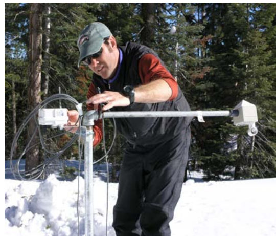
FIGURE 4-22 One pod in a sensor web that was installed to measure snow depth over a 20,000 m 2 study area in Yosemite National Park. Depth sensor is on right and wireless pod on left. Photograph courtesy of Margot Wholey Photography.
