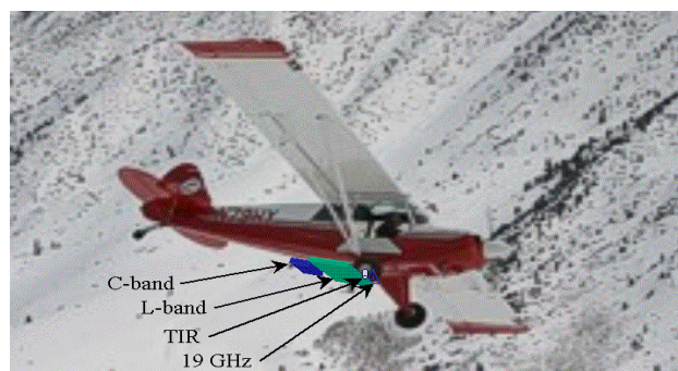
FIGURE 4-13 An Aviat Husky aircraft showing location of radiometers in a pod attached to the float fittings of the aircraft. The design study included 1.4, 6.9, and 19 GHz nadir-viewing, profiling radiometers, and a thermal infrared (TIR) profiling sensor. All sensors have a 17^\circ beamwidth yielding 30 m footprints at 100 m heights above ground. Radiometers were Dicke-capable with two-point calibration and digital detection. 60 kn airspeeds yield 110 ms integration times with a 10 percent footprint smear, a NEAT of \sim 0.8 K at 1.4 GHz, and \sim 0.4 K at higher frequencies. Modified, with permission, from Aviat Aircraft, Inc., Afton, Wyoming.
