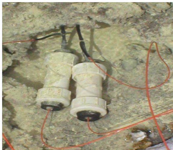
FIGURE 2-6 In-situ continuous flow reactors for microbiologic community and activity sampling. SOURCE: Reprinted, with permission, from E. Boyd and G. Geesey, Montana State University.
