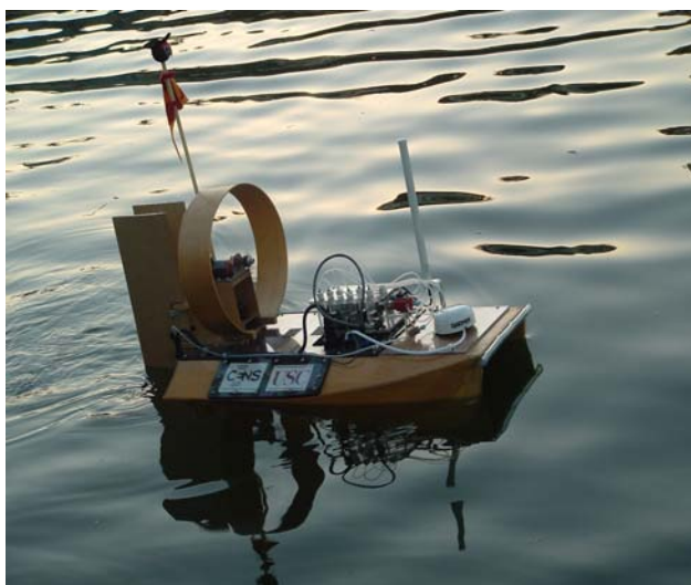
FIGURE 2-7 A robotic boat for microbiologic sampling. SOURCE: Reprinted, with permission, from Dhariwal et al. (2006). © 2006 by IEEE.
