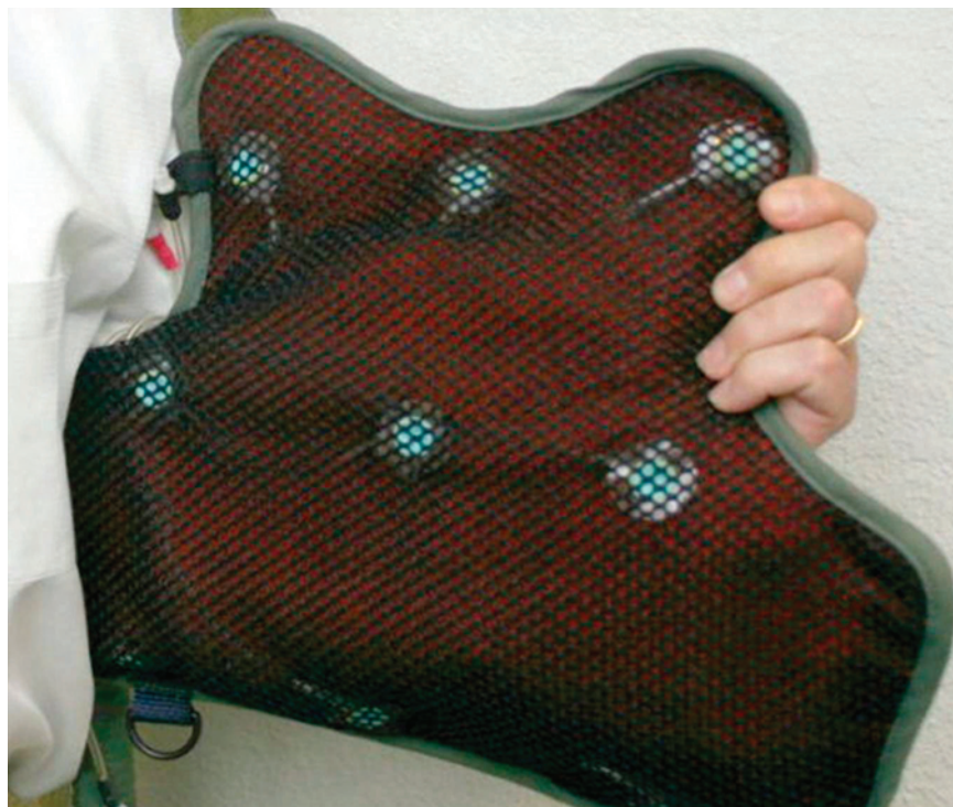
FIGURE 3-4 Vibrotactile displays for pilots experiencing sensory overload or cognitive illusions have been a successful application of sensory substitution technologies. Pilots, operators of complex equipment, and analysts monitoring large amounts of data can benefit as information is made available through underused sensory modalities that are more effective in some contexts than vision or hearing. SOURCE: Raj et al. (2005).
