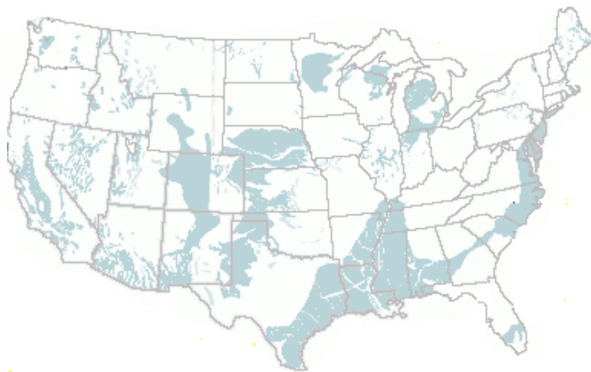
FIGURE 5-3. Areas where subsidence has been attributed to groundwater withdrawal. SOURCE: Galloway et al. (1999).
