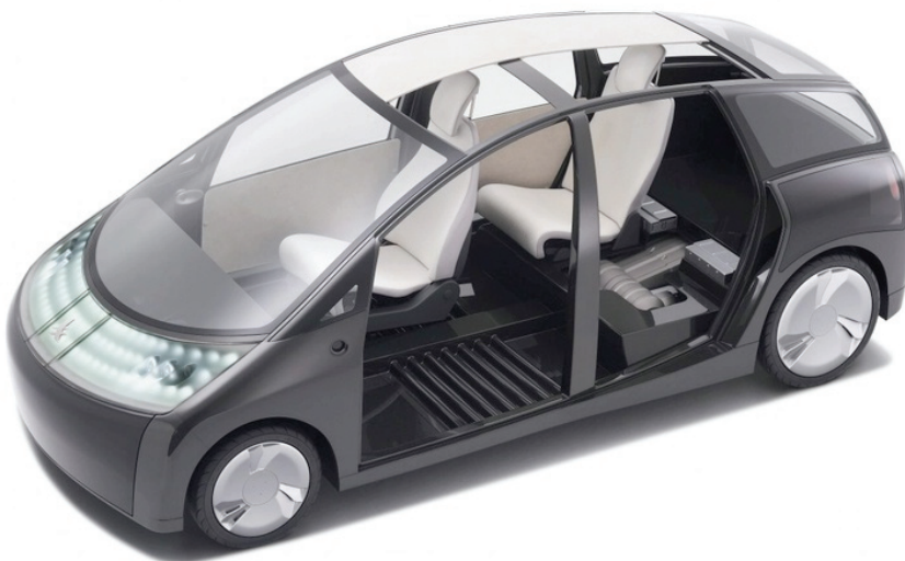
FIGURE 9.2 The 1/X concept car, designed by Toyota, that weighs one-third as much as a Prius, uses half as much energy, and yet has the same interior volume. SOURCE: Toyota Motor Corporation.
