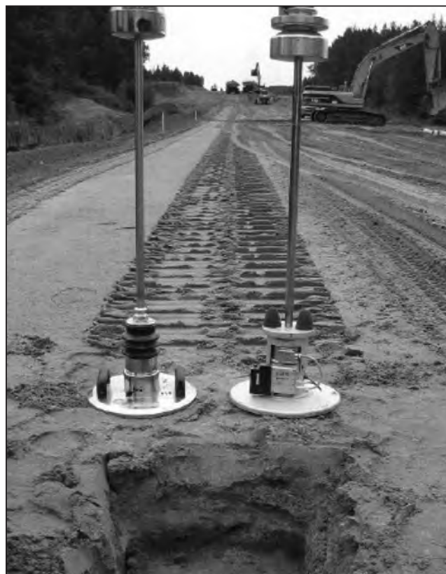
FIGURE 54 LWD devices in field operation (White et al. 2007).
