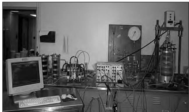
FIGURE 25 Triaxial unit with data acquisition and control panel unit.
