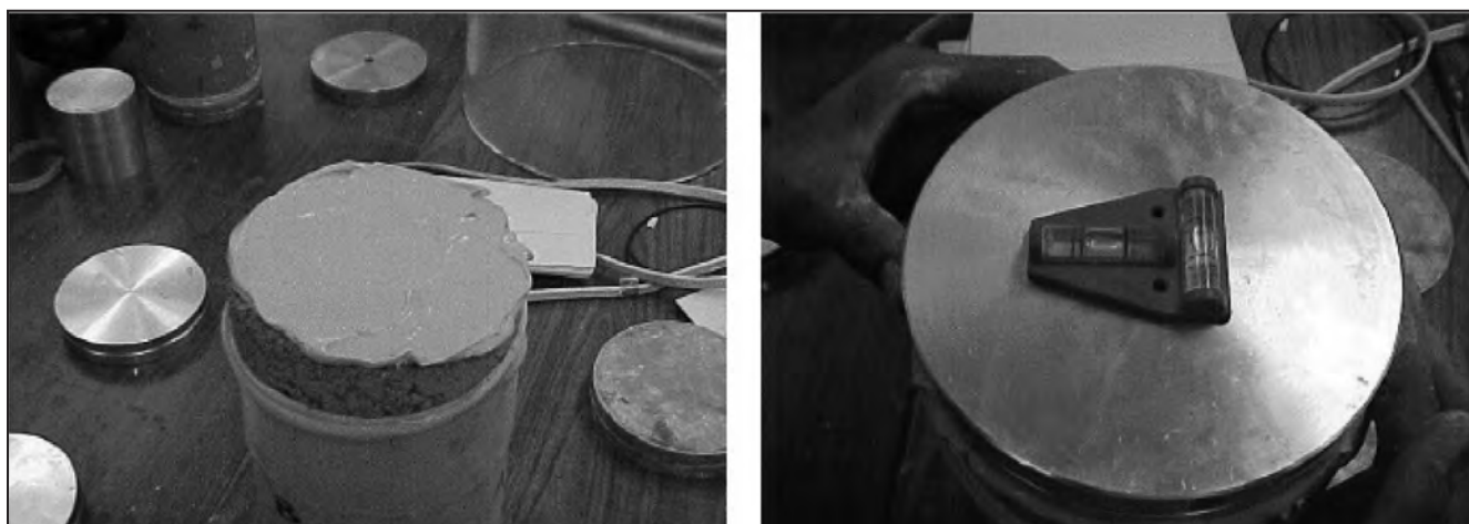
FIGURE 38 (left) Grout used for specimen ends; (right) Leveling measurements on the top cap (Gandara et al. 2005).
