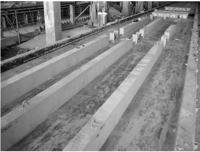
Figure 3.17. Fabrication of rectangular beams.
