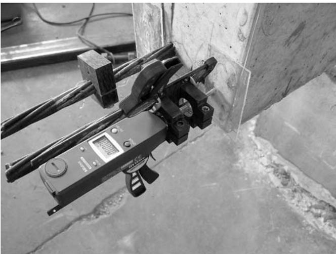
**Figure 3.38.** Mechanical deflection gage arrangement for measuring strand end slips at the beam end opposite to the test end.
