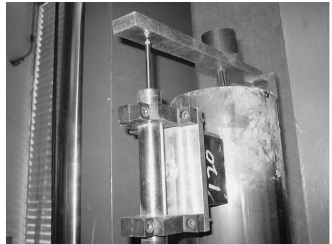
Figure 3.5. LVDT on NASP Test specimen.
