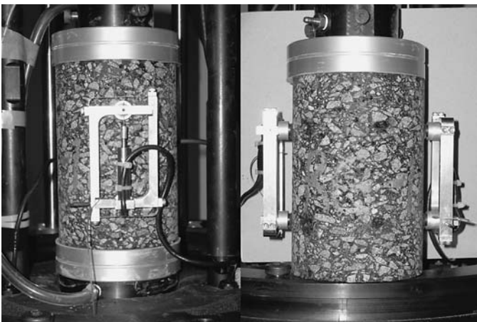
Figure 18. MDTs specimen mounted deformation measuring system.
