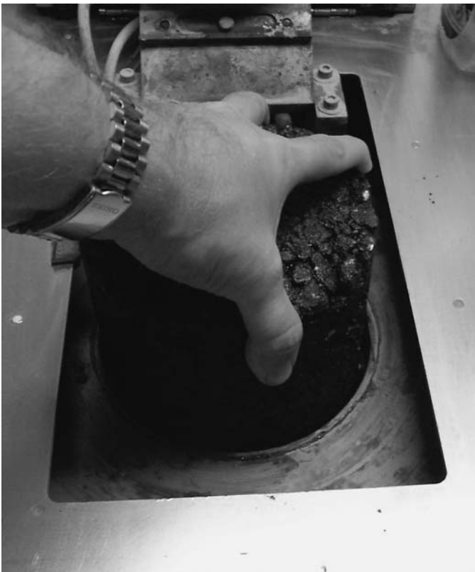
Figure 28. Inserting gyrotory specimen in the FlexPrep™ chuck.
