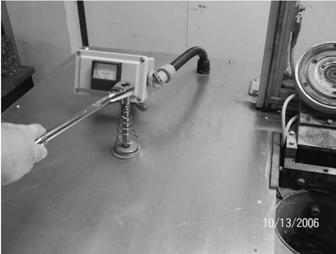
Figure 27. Opening chuck using a socket wrench.
