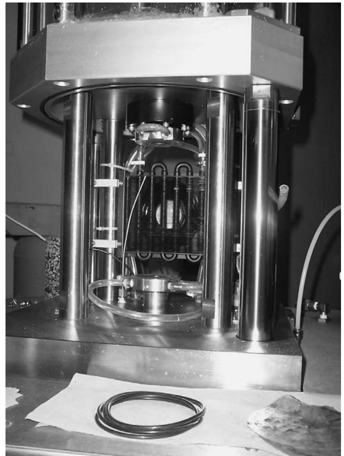
Figure 12. Open test chamber for the upgraded Interlaken SPT.
