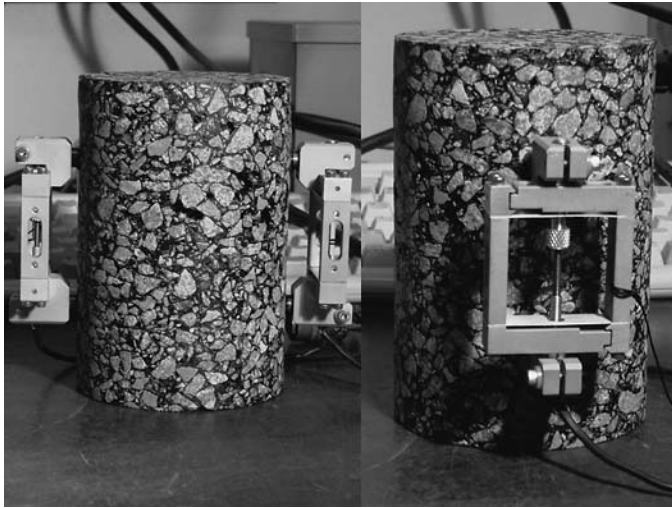
Figure 13. Interlaken specimen mounted extensometer system.
