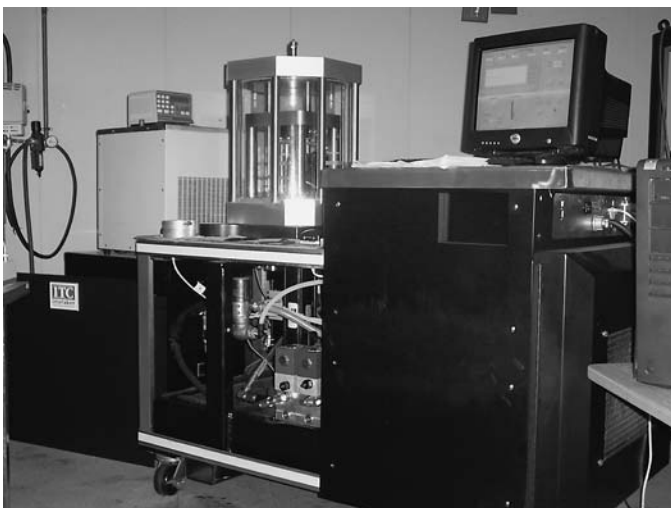
Figure 11. Overall view of upgraded Interlaken SPT (main cabinet removed to show system hydraulics).
