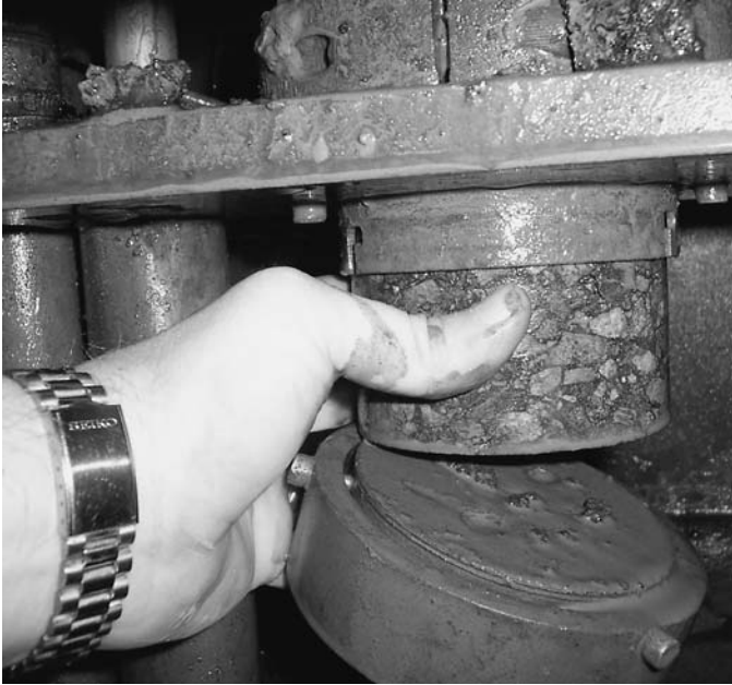
Figure 31. Removing finished test specimen from the bottom of the core barrel.
