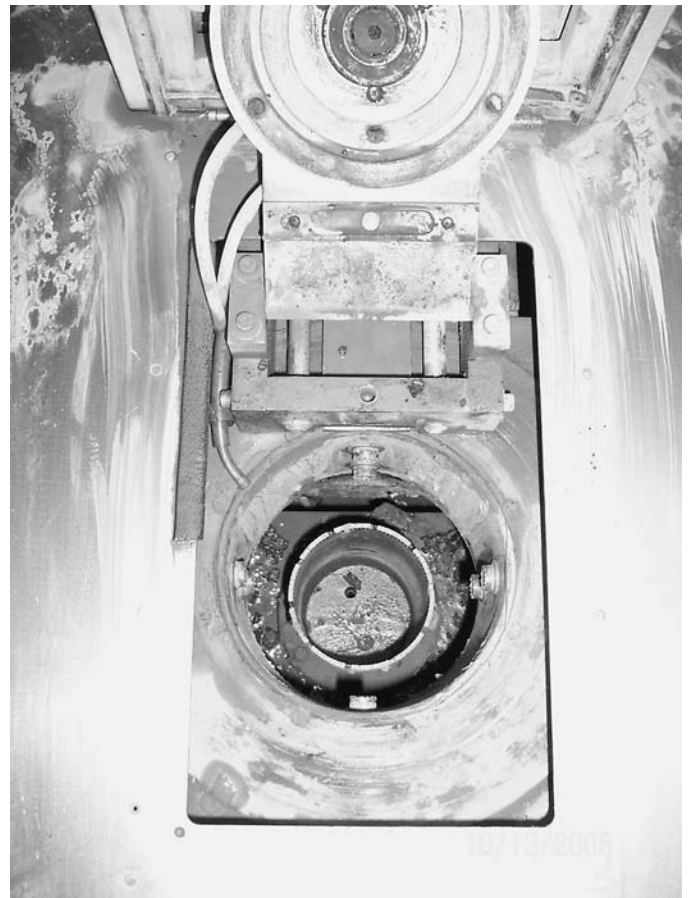
Figure 26. Top view of FlexPrep™ chuck with upper door and specimen back-up plate open.
