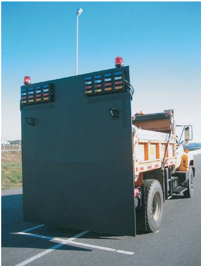
Rotating beacons placed on the top of the panel.
