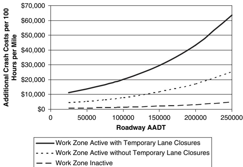
**Figure 15. Effect of strategies to reduce work zone frequency and duration: daytime conditions.**
