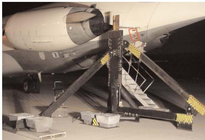
**Figure 5. Probe rake assembly used during Phase 1 of the Delta Atlanta-Hartsfield Study.**
