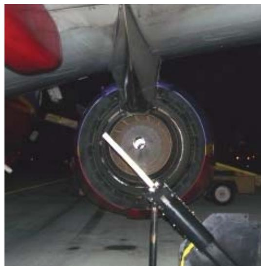
Figure 7. Layout of the mobile laboratories in the GRE and probe rake assembly used in JETS-APEX2.
