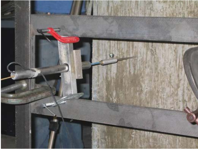
Figure B-25. Close-up view of LVDT used to measure end slip. Note single king wire of strand extends through the concrete.
