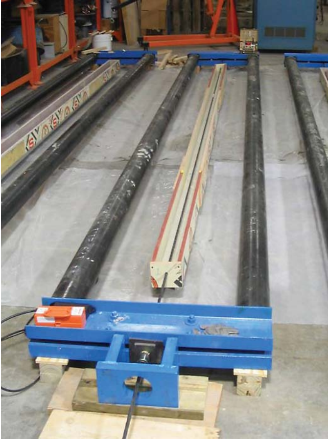
Figure B-5. Tensioned strand in form used for casting transfer length specimen.
