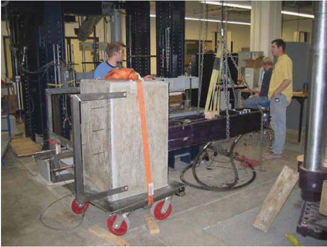
Figure B-21. Test set-up. Concrete block is turned on its side, loading apparatus placed at one side (live end) and measurement of end slip instrumentation mounted at the other side (dead end).
