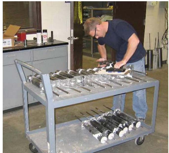
Figure B-48. Completed specimens ready for test.
