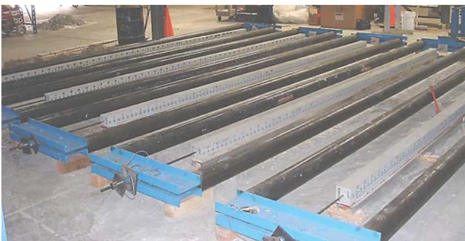
Figure B-6. Specimens with Whittemore buttons attached.
