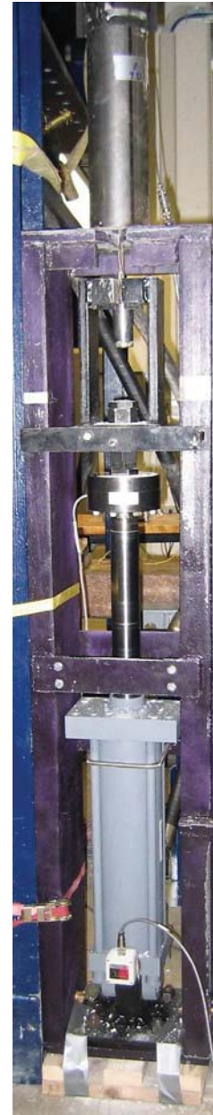
Figure B-29. NASPA test specimen at KSU. Note stiff frame.
