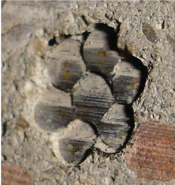
Figure B-11. Strand appearance after mid-point saw cut of transfer length prism.
