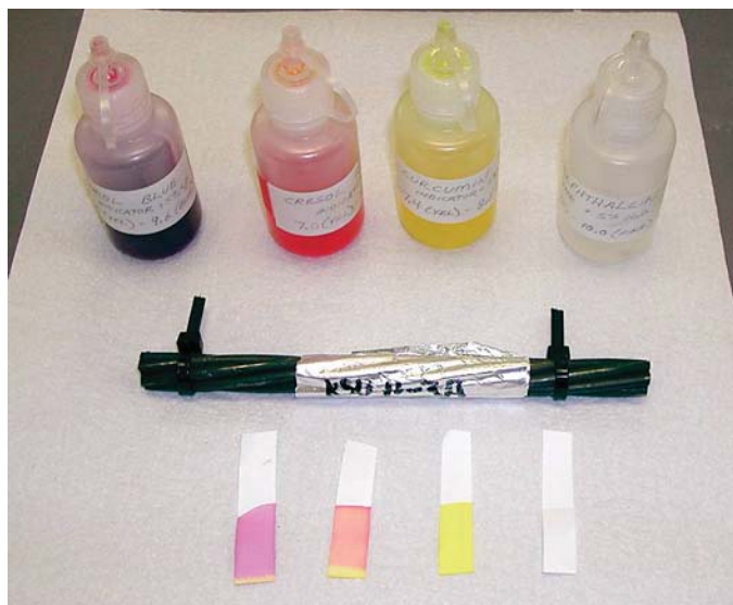
Figure B-59. Indicator solutions (from left to right, Thymol Blue, Cresol Red, Curcumin, Phenolphthalein) and strips of indicator-treated paper that had been applied to strand surface.
