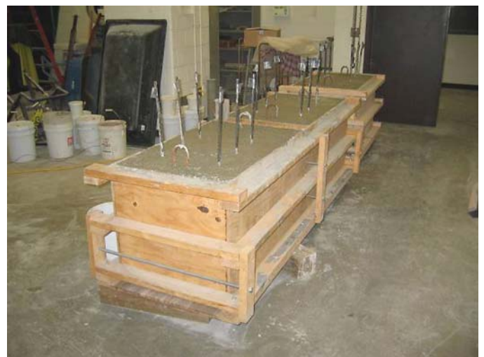
Figure B-24. Large blocks immediately after casting. Concrete is cured at lab room temperature.
