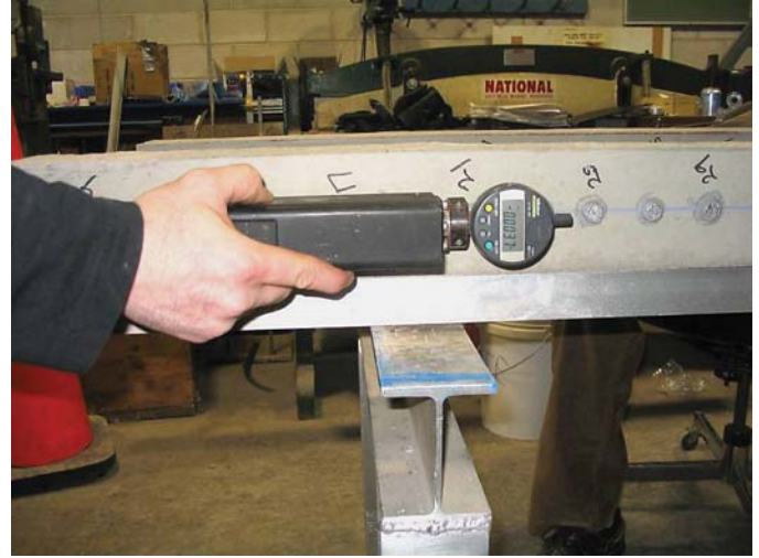
Figure B-7. Whittemore gauge readings used to calculate strain.
