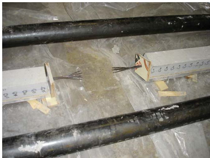
Figure B-15. Strands between specimens after torch cut.
