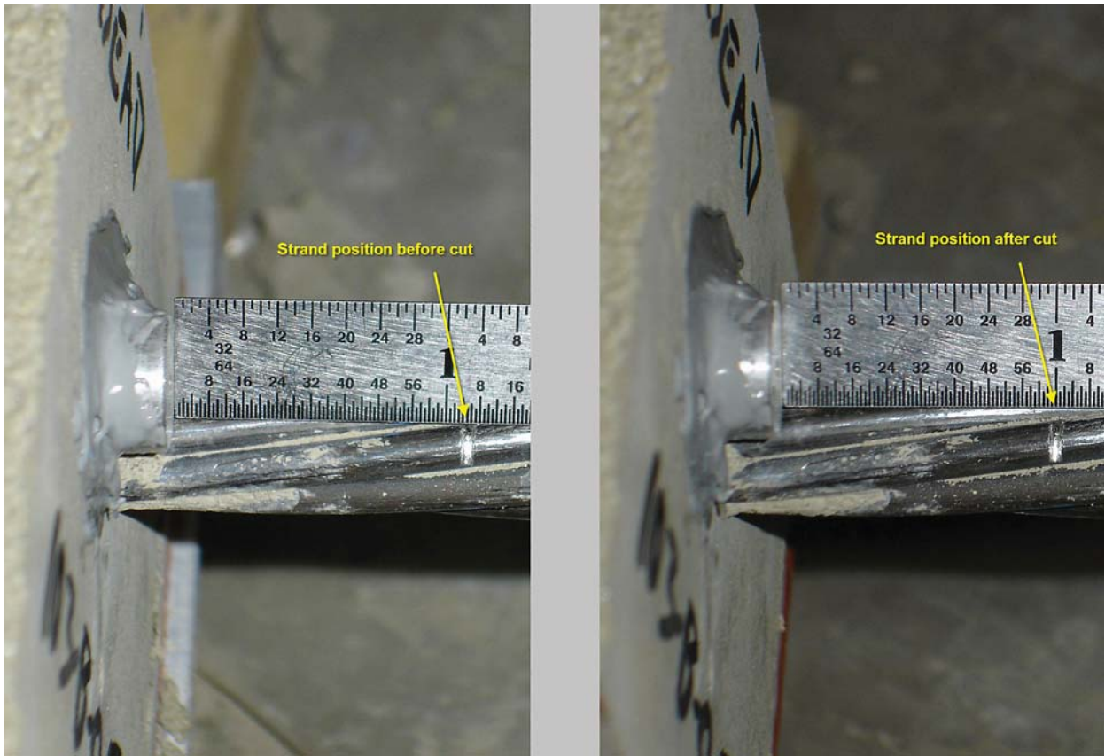
Figure B-8. Measurement of strand slippage from dead end—Strand 103B.
