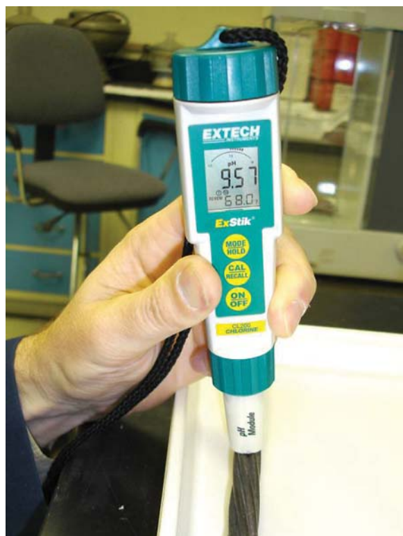
Figure B-60. Exstik hand-held pH meter.
