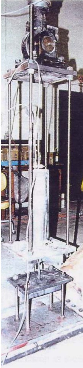
Figure B-28. NASPA test specimen at OU. Note flexible frame.
