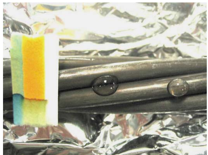
Figure B-58. Surface of strand during pH testing (the bottom of the universal indicator paper, as shown, was touched to the water and has changed color).
