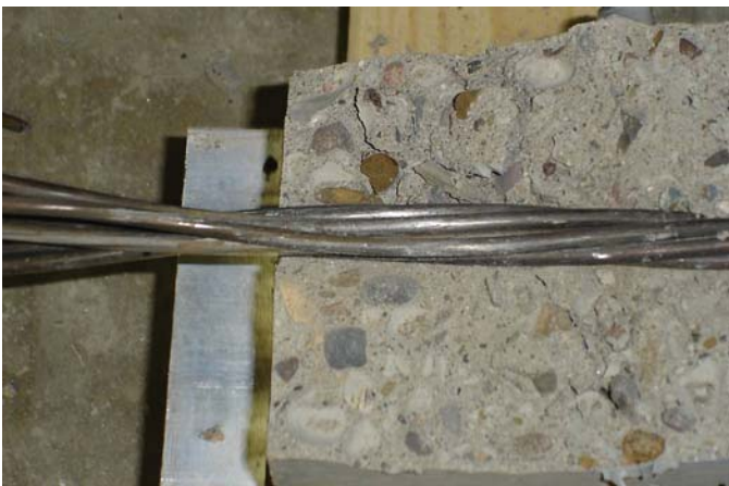
Figure B-9. Fractured end of prism after rapid release of strand.
