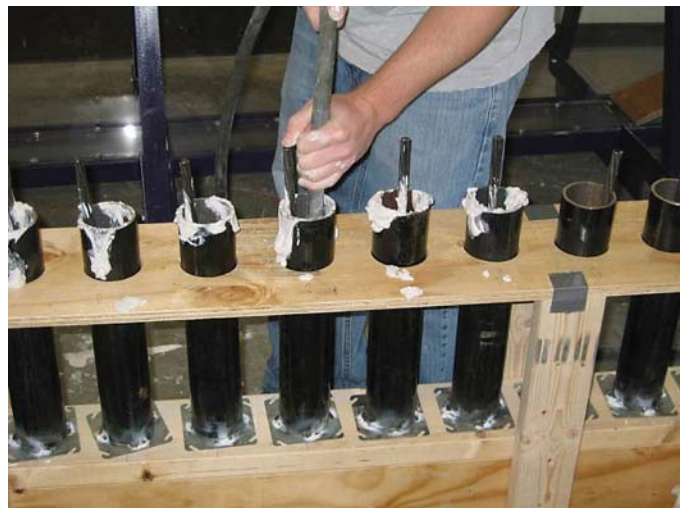
Figure B-46. Vibrating the Hydrocal mixture.
