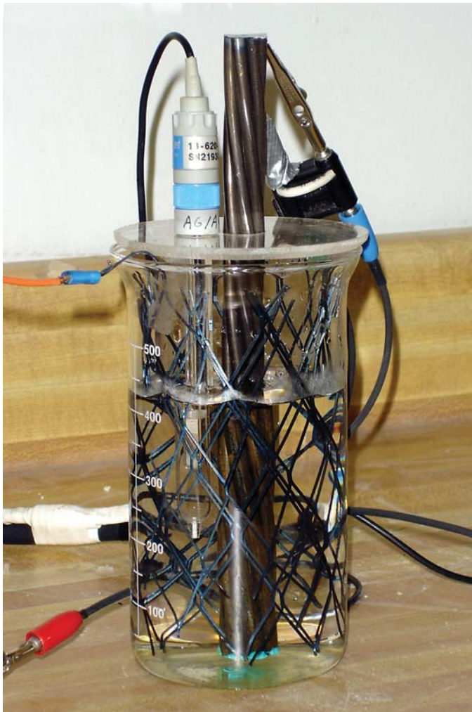
Figure B-66. Setup for corrosion rate testing.
