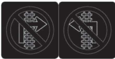
FIGURE 10 No left-/right-turn-activated blank-out signs with tracks symbol (Courtesy: Metropolitan Transit Authority of Harris County, Texas).
