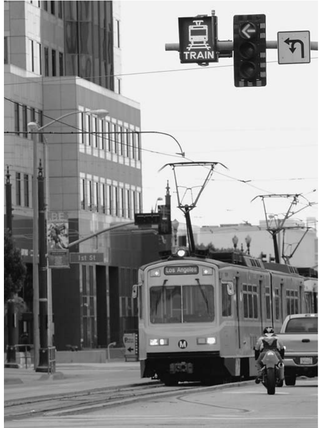
FIGURE 6 Train-activated warning sign in Los Angeles.
