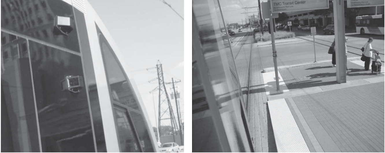
FIGURE 27 Houston METRO's train-mounted camera ( left ) and view from camera ( right ) ( Courtesy: Houston METRO ).
