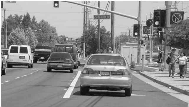
FIGURE 9 No right-turn activated blank-out sign in Sacramento (Courtesy: Sacramento Regional Transit District).
