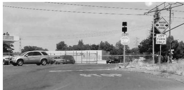
FIGURE 33 Ahern Street approach to 12th Street with pedestrian head train approaching warning sign (Courtesy: Sacramento Regional Transit District).
