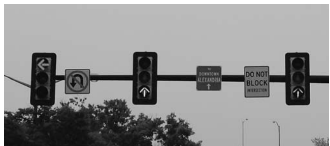
FIGURE 20 Use of arrows to control traffic movements.
