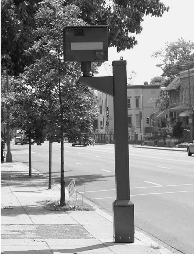
FIGURE 25 Photo enforcement camera (Courtesy: Los Angeles County MTA).
