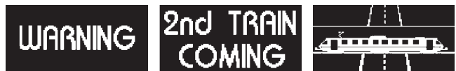
FIGURE 17 Second train coming warning sign (Courtesy: Ziad Sabra, Sabra, Wang and Associates, Inc.).
