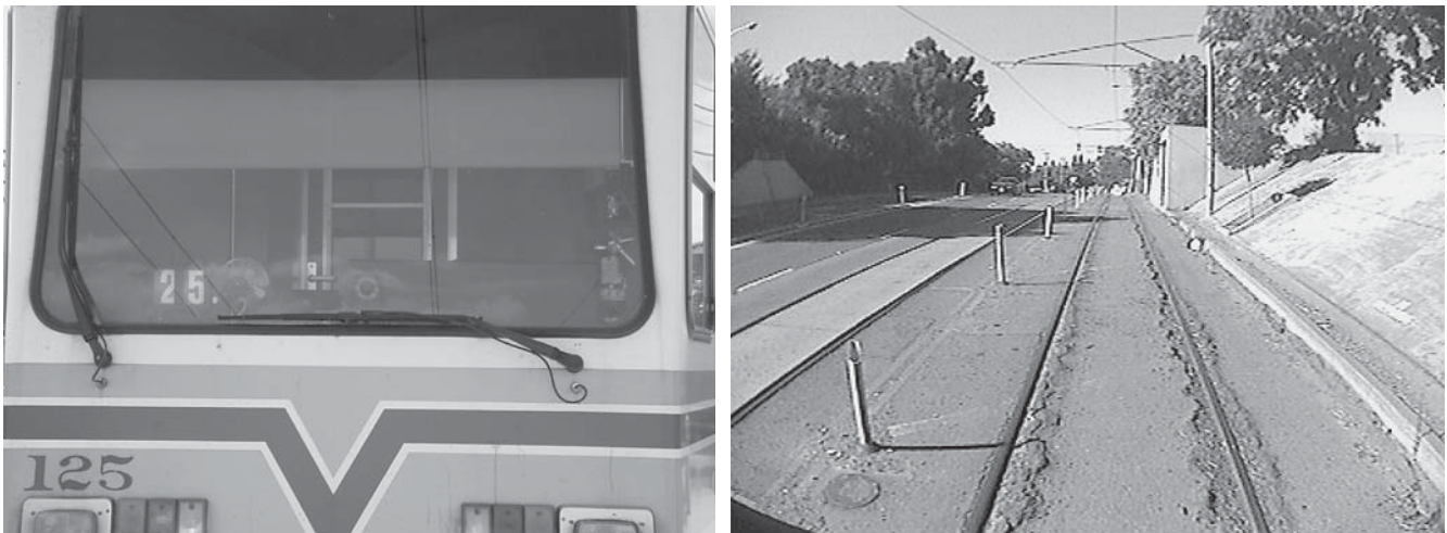
FIGURE 26 Sacramento RT's train-mounted camera (left) and view from camera (right) (Courtesy: Sacramento Regional Transit District).
