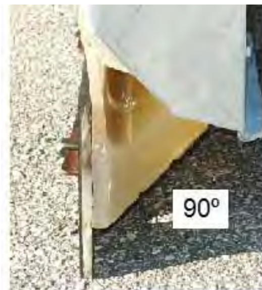
FIGURE 5 New cutting edge, 90-degree angle.
