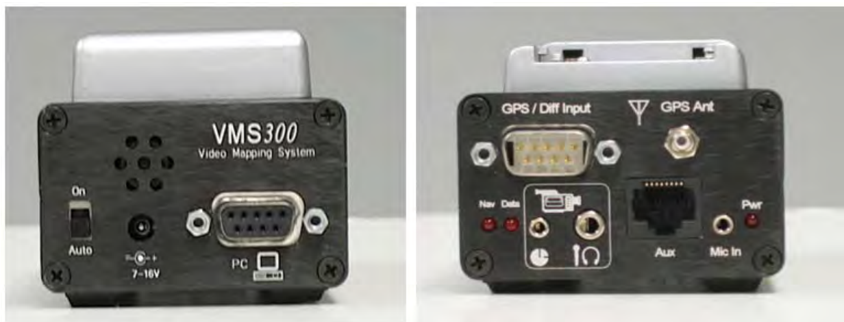
FIGURE 4 Front and rear views of RedHen GPS–video unit. Input and output ports for a laptop, GPS antenna, telephone, microphone, and video camera are shown.
