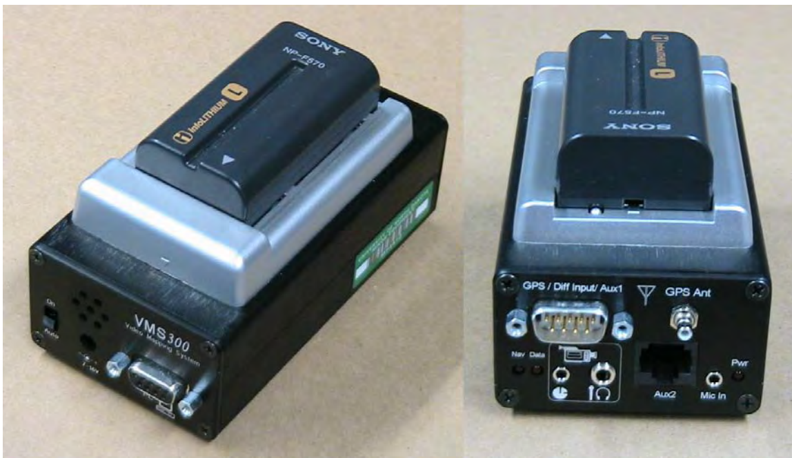
FIGURE 3 Red Hen Systems, Inc., VMS 300 GPS unit used to collect GPS data.
