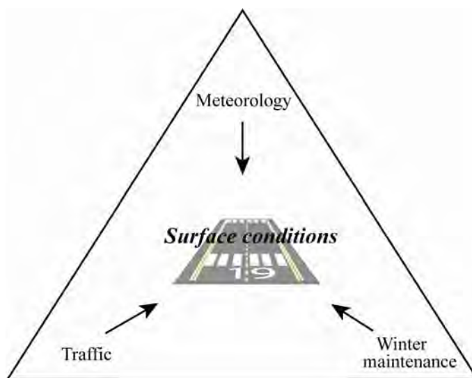
FIGURE 1 Basic conceptual model of processes affecting runway surface conditions.
