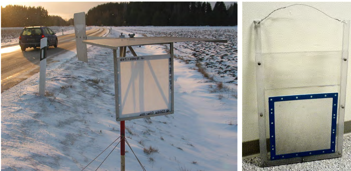
FIGURE 2 A salt vane for sampling airborne salt spray from the road. To the right: dissolving the chloride in deionized water.
