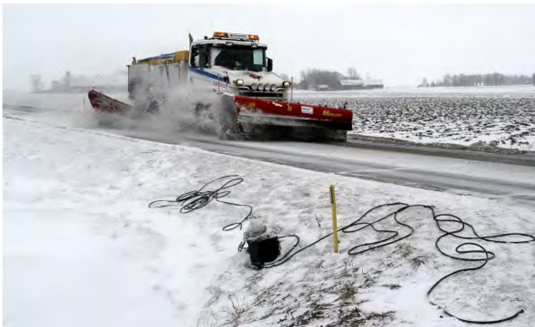
FIGURE 3 The plowing truck passing by at the field site. The traffic counting rubber tube is temporarily disconnected to facilitate the plowing truck's passage.
