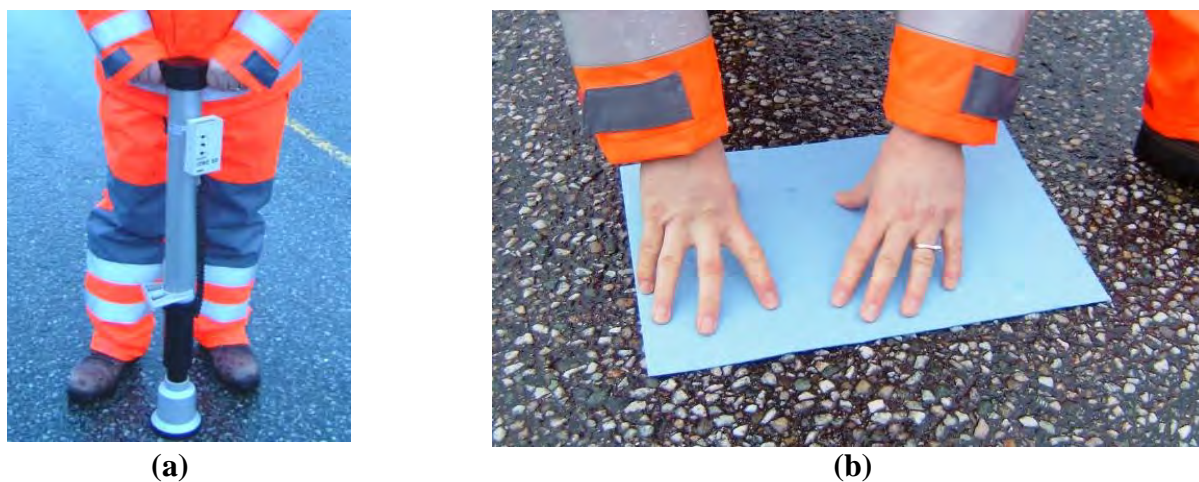
FIGURE 3 Measuring (a) salt amount with SOBO 20 and (b) water amount with Wetex textile.
