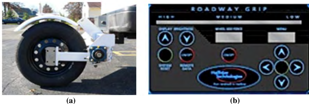
FIGURE 1 Close-up view of (a) RT3 auxiliary wheel, GEM hub and tow hitch and (b) RT3 software console mounted in the research vehicle.
