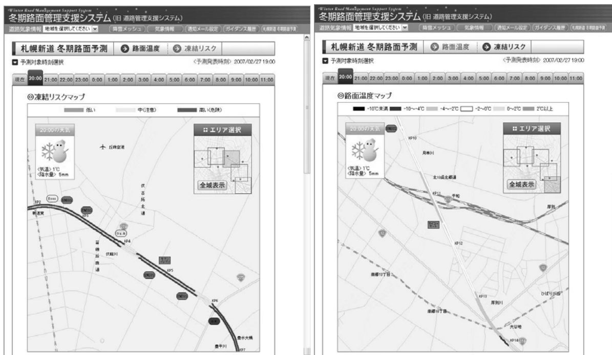
FIGURE 10 Area expansion screen (left, road surface temperature; right, road icing risk).
