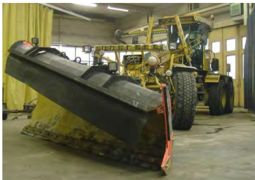
FIGURE 9 Grader with front-mounted plow and plowshare.
