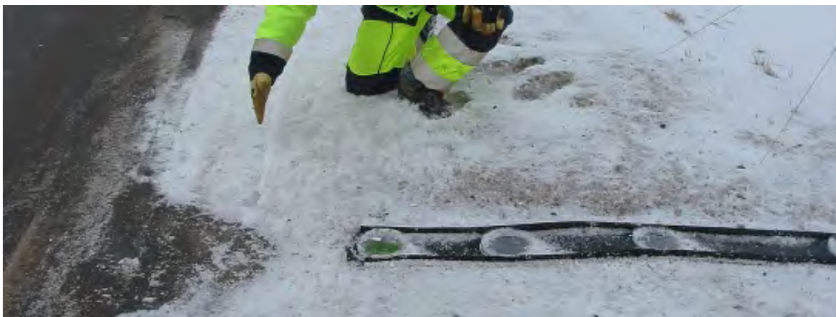
FIGURE 4 Salt deposition in plastic petri dishes on an hourly basis. The closest petri dish is at a distance of one meter from the road borderline. Please note the closeness of the cutting edge of the plow to the first petri dish.
