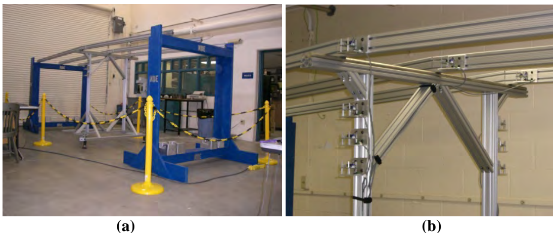
FIGURE 3 Photograph of test bridge (a) and sensors on pier and (b) superstructure.
