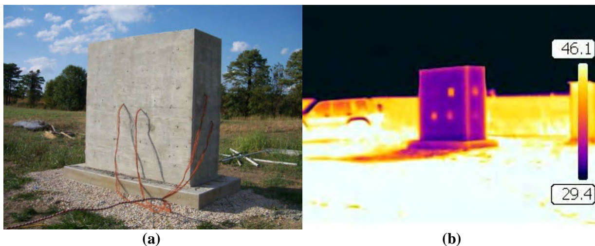
FIGURE 2 (a) Completed test block being monitored and (b) IR image of same block showing subsurface targets at 1, 2, and 3 in. (5-in. deep target is not apparent).
