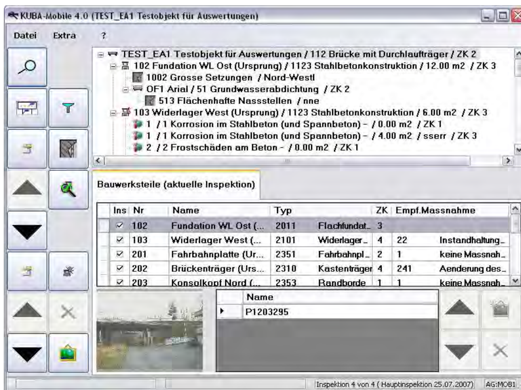
FIGURE 8 Collection of inspection data in KUBA.
