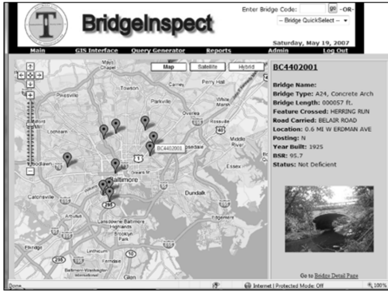
FIGURE 6 Interactive mapping interface showing bridges matching a search and specific bridge highlighted.
