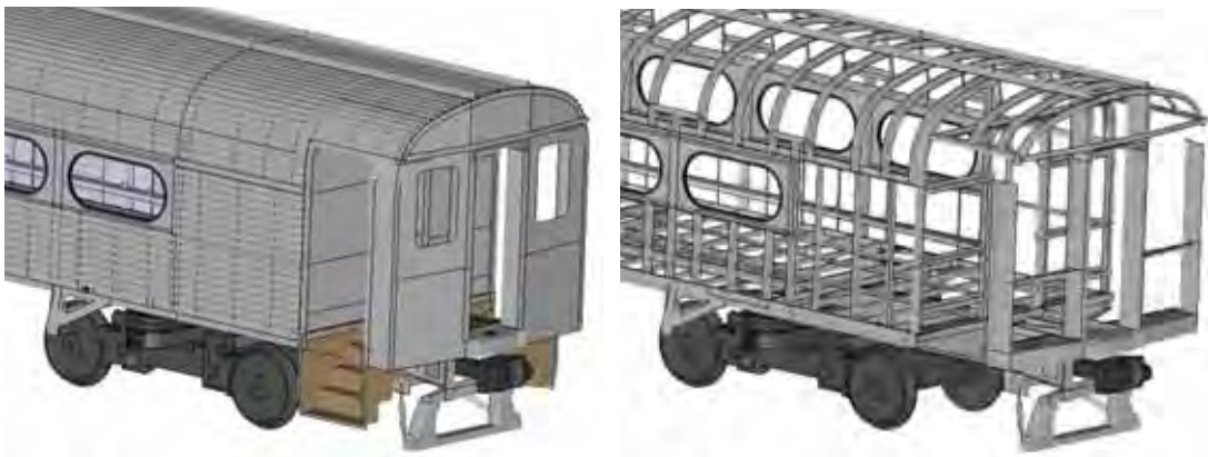
Figure 16. Detailed finite Element Model of a Pioneer Passenger Coach Car.
