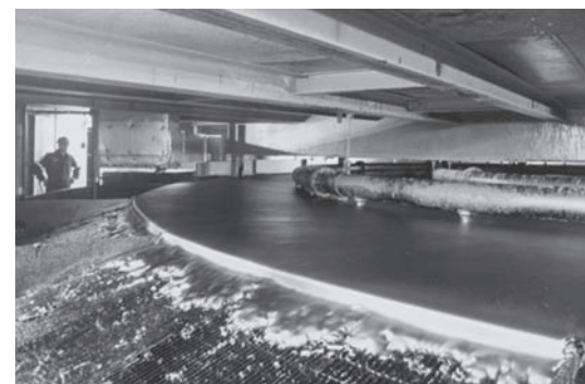
A separation cell is one step in the extraction of bitumen from tar sands mixed with water.
