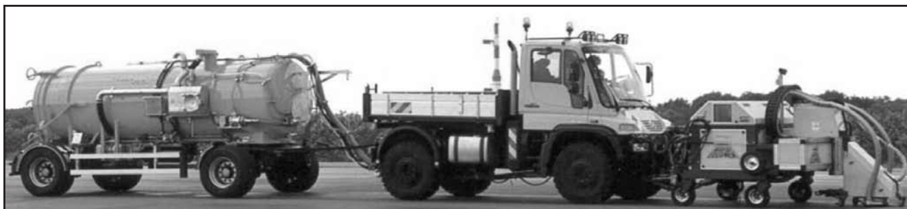
FIGURE C2 European vehicular-mounted and controlled waterblaster (Pade 2007).
