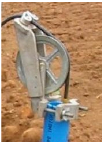
FIGURE 4 Cable control fixture.
