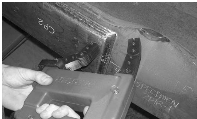
Figure 1.15. Magnetic particle inspection—placement of the magnetic field.
