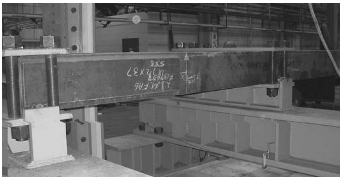
Figure 1.7. Typical setup of a specimen in the drop-weight machine.
