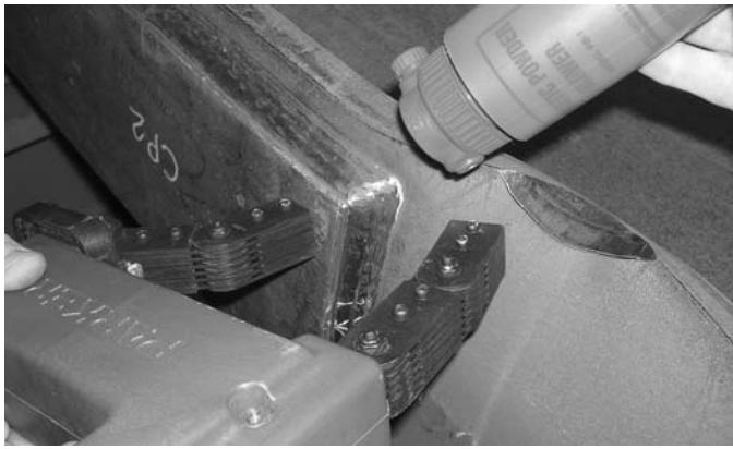
Figure 1.16. Magnetic particle inspection—application of magnetic particles.
