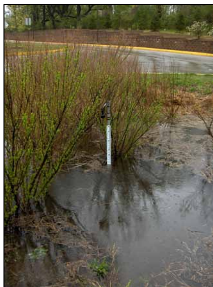
FIGURE 5-51 Staff gauge attached to ultrasonic sensor after a storm. SOURCE: Reprinted, with permission, from VUSP. Copyright by VUSP.
