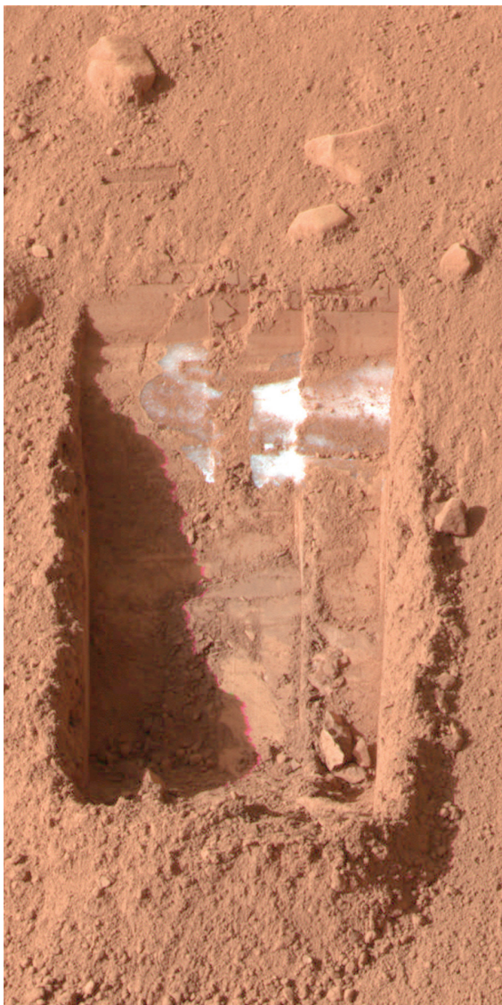
FIGURE 2.1 Image acquired by the Surface Stereo Imager on NASA's Phoenix lander. The view is of a 22-centimeter-wide trench excavated by the lander's robotic arm on Sol 18. The white material exposed in the floor of the trench is interpreted to be water ice. SOURCE: Courtesy of NASA/Jet Propulsion Laboratory-California Institute of Technology/University of Arizona/Texas A&M University.
