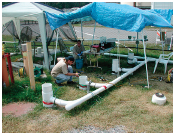
FIGURE 3.4 Oak Ridge Field Research Center. Site-specific data are required for characterizing geohydrology and measuring contaminant transport and effects of remedial actions. A specific location on a site, including dedicated boreholes, water wells, and equipment, may be developed for this purpose. Monitoring wells located around the site and surface water sampling also provide field data. Geohydrological parameters usually change slowly, so maintaining these facilities for years or decades is necessary.
