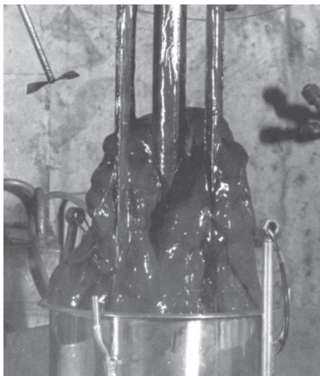
FIGURE 2.2 Sludge sampled from an SRS tank. Tank sludge was formed by neutralizing acidic waste from the reprocessing of nuclear fuels and recovery of nuclear materials. This sludge flowed like a thick paste. Other sludges are more viscous or nearly solid, which makes them difficult to remove from the tanks. This approximately 2-liter sample was opened inside a shielded laboratory cell like that shown in Figure 3.2 in the late 1970s.
