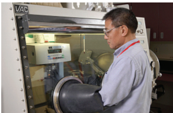
FIGURE 3.1 Glove box in a radiochemical laboratory. Glove boxes provide safe containment for laboratory work with radioactive or chemically hazardous materials. Substantial amounts of radionuclides that do not emit penetrating radiation (e.g., Pu-239) can be handled in a glove box. Glove boxes offer good visibility and access, but the thick, often lead-lined gloves limit the manual dexterity of scientists and technicians.
