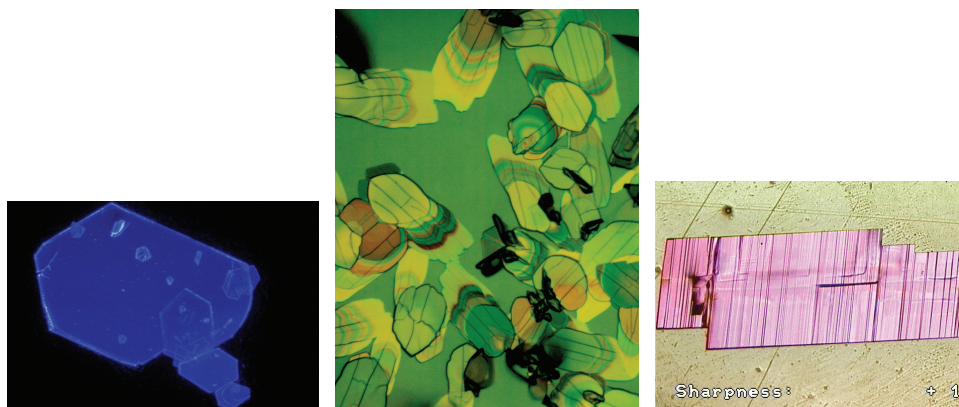
FIGURE 2.16 Examples of organic single crystals with possible use in solar cells. (Left) Anthracene seen in blue backlight, (middle) \alpha -hexathiophene, and (right) fluorinated copper phthalocyanine showing growth steps. SOURCE: Courtesy of Christian Kloc, Nanyang Technological University.
