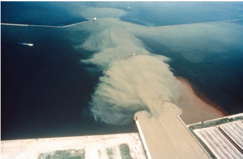
FIGURE 2-15 Milwaukee River emptying into the Lake Michigan harbor following a period of high flow and attendant creation of a plume. Note the breakfront and the southerly movement of the plume. SOURCE: Image courtesy of Kathy Blair.
