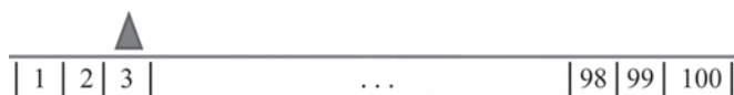
FIGURE 15.1 A random walk on a line with 100 locations. Unless the marker is at the left-most or the right-most location, it moves 1 space to the right if the tossed coin lands heads and 1 space to the left if the coin lands tails.
