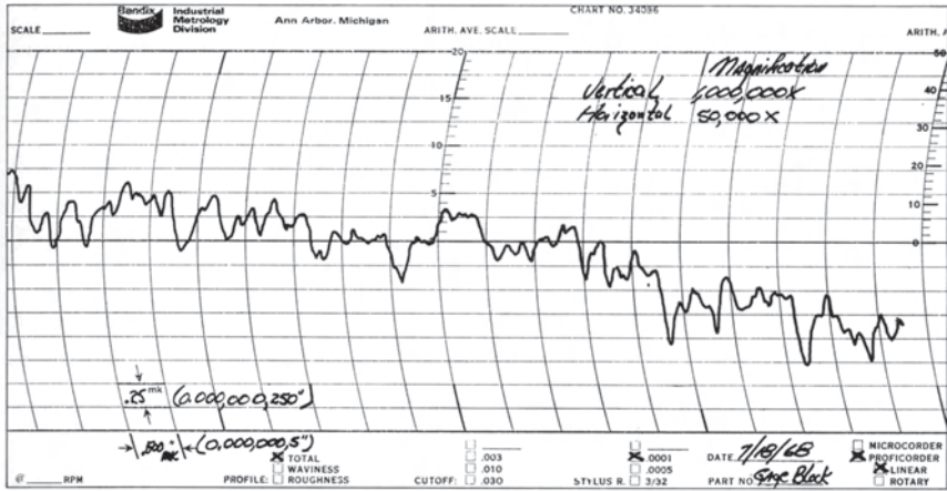
FIGURE 17.4 A surface trace of a precision gauge block at 1 million times vertical magnification, illustrating the representation of deviations from perfection. SOURCE: Reproduced with permission from Moore (1970) (Copyright 1970, Moore Special Tool Company).
