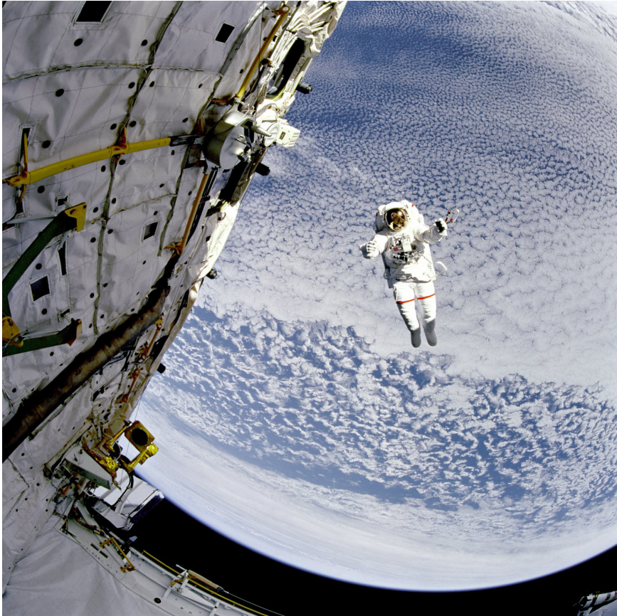
FIGURE 2.4 An astronaut tests the Simplified Aid for Extra-Vehicular Activity Rescue system during an extravehicular activity. SOURCE: Courtesy of NASA.
