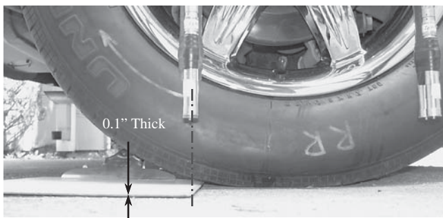
Figure 2. Orientation of the OBSI probe to the edge of the tire contact patch—trailing edge position.
