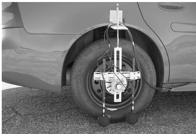
Figure 8. OBSI equipment installed on DPG test vehicle.
