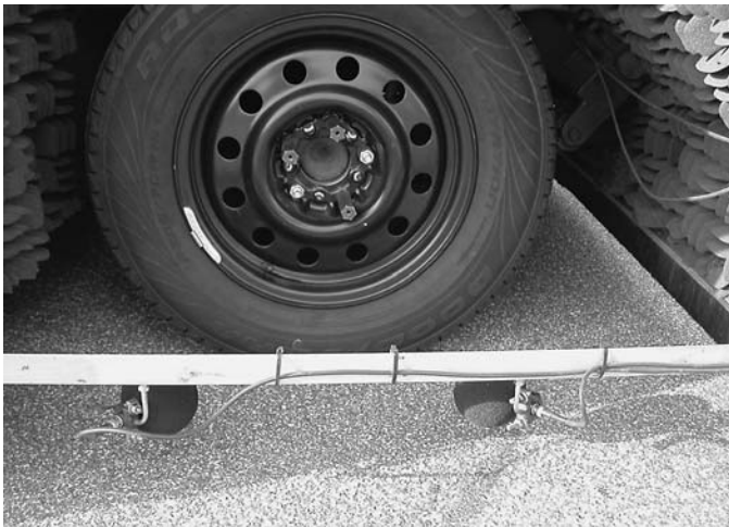
Figure 1. CPX tire-pavement noise measurement configuration.
