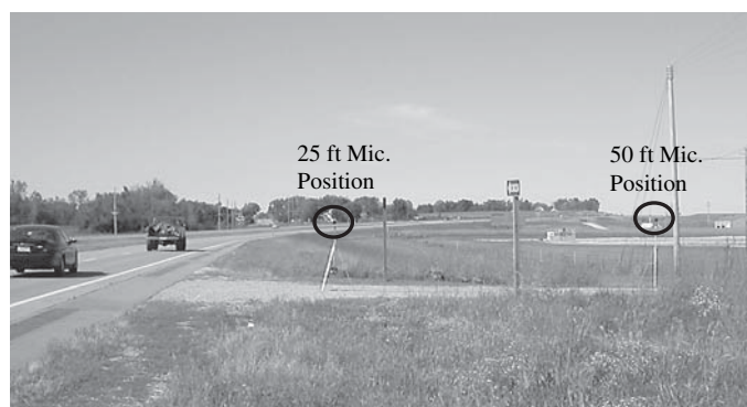
Figure 12. Typical passby measurement setup.
