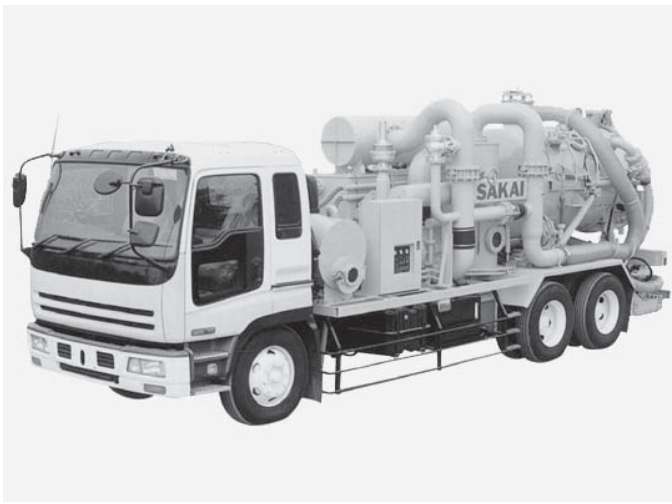
Figure 40. Truck mounted PFC cleaning system (65).
