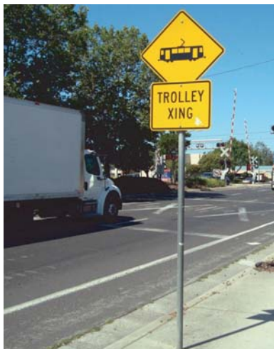
Photo (courtesy José Farrán) shows a typical retroreflective advance warning sign from San Jose.
