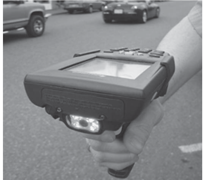
Figure H.3. Handheld license plate reader for conducting license plate inventories.
