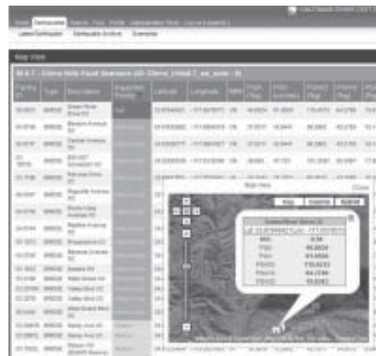
ShakeCast website and visualization tools. (MMI = Modified Mercalli Index; PGA = peak ground acceleration; PGV = peak ground velocity; PSA = peak spectral acceleration for 0.3 s, 1 s, and 3 s.)
