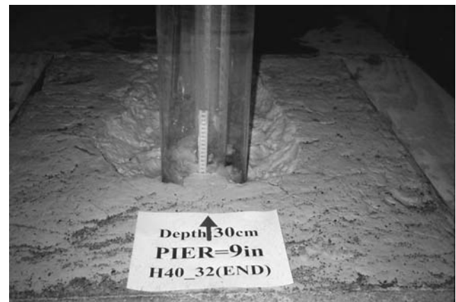
FIGURE 19 Flume test showing scour hole behind a pier in cohesive soil (Courtesy: Texas A&M University).
