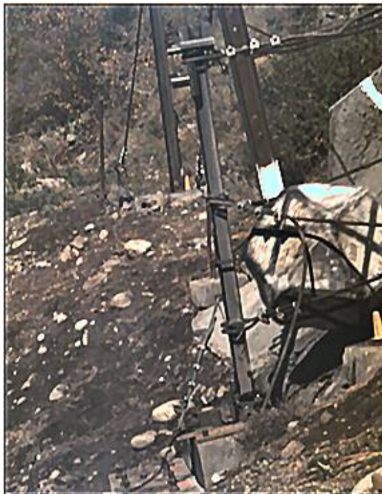
FIGURE 63 Test No. 120 (pin-connection post just prior to impact).
