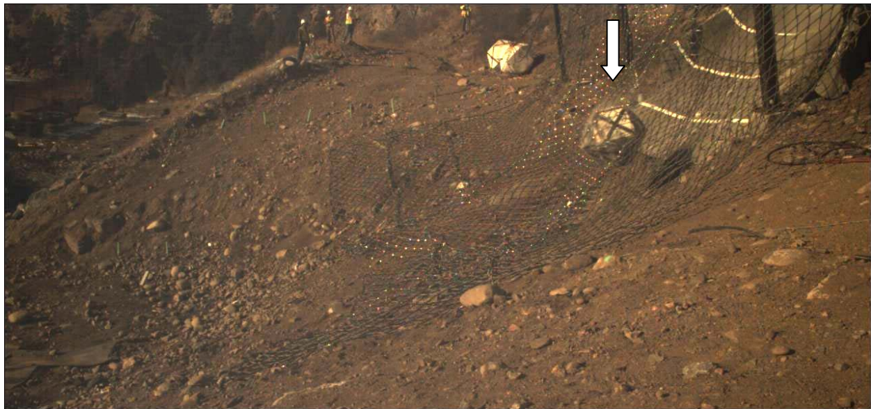
FIGURE 46 Cuboctahedron rock (in upper right corner) prior to impacting panel depicted by white arrow.
