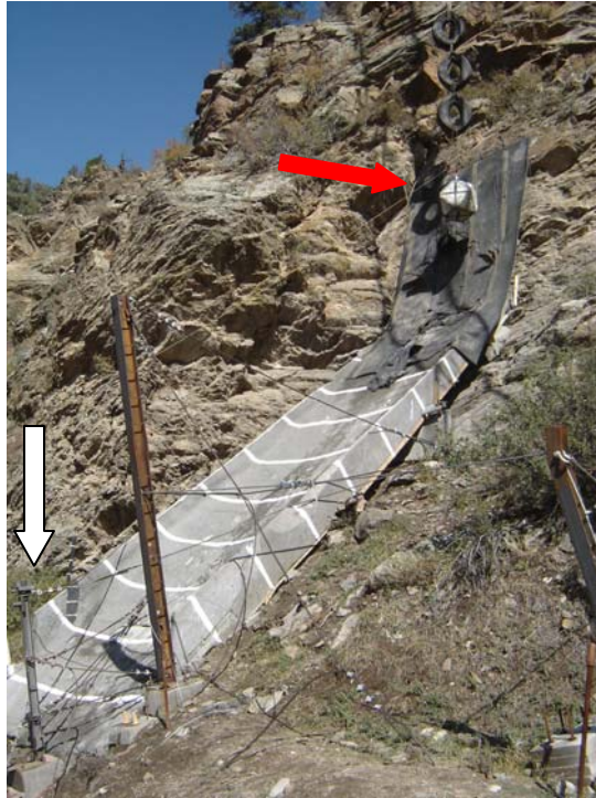
FIGURE 62 Test 120 prior to release of rock at mid-height on ramp (red arrow indicates location of rock prior to drop; white arrow indicates pin-connection post at bottom of ramp).
