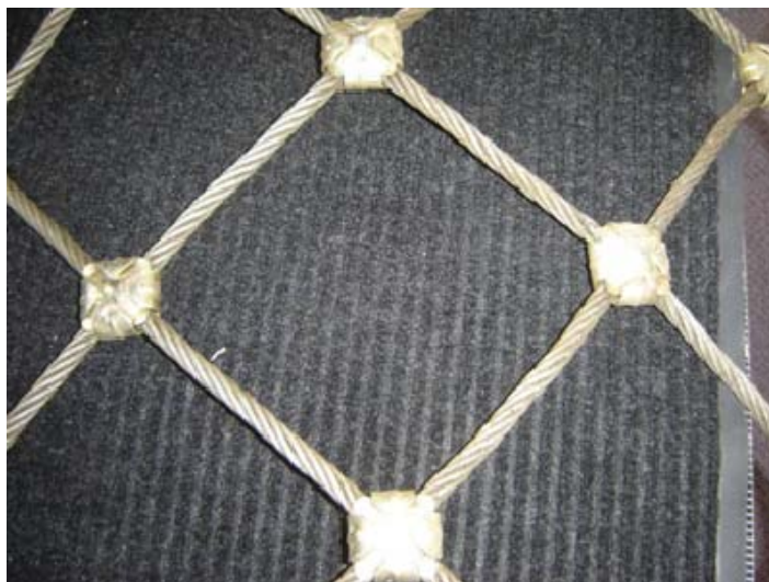
FIGURE 22 Cable net made with 12-mm diameter wire and overlap clamp style, diagonal weave.
