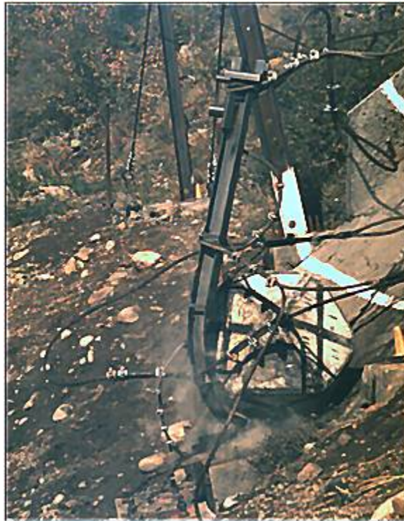
FIGURE 64 Test No. 120 (pin-connection post during impact).
