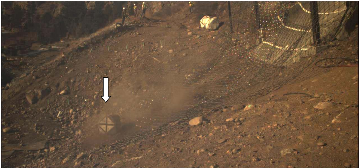
FIGURE 52 Rock fully released at much reduced velocity (at this point, would begin to reaccelerate until it impacts another attenuator or final catchment or barrier).
