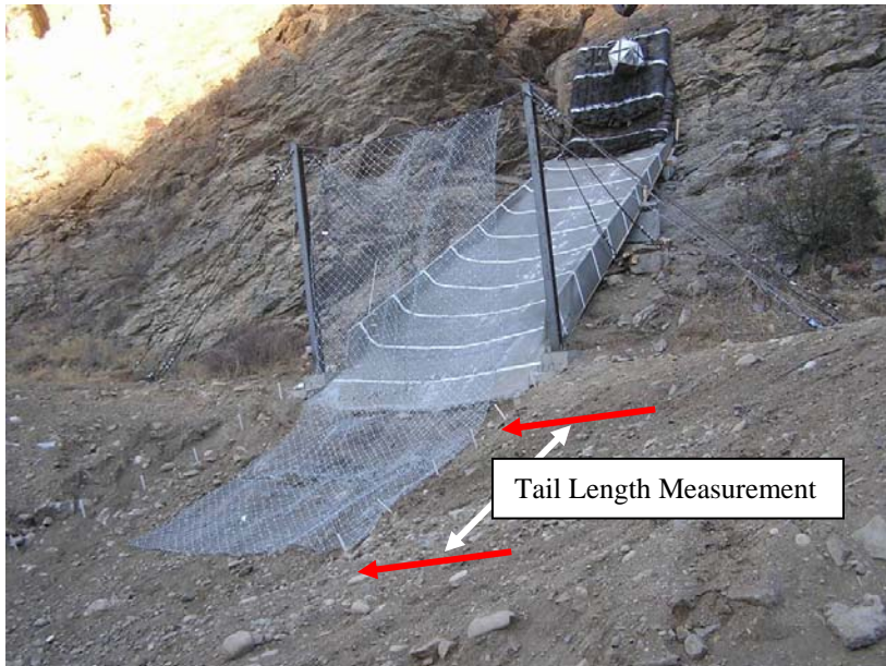
FIGURE 45 Measurement of tail length for net panel in contact with ground.
