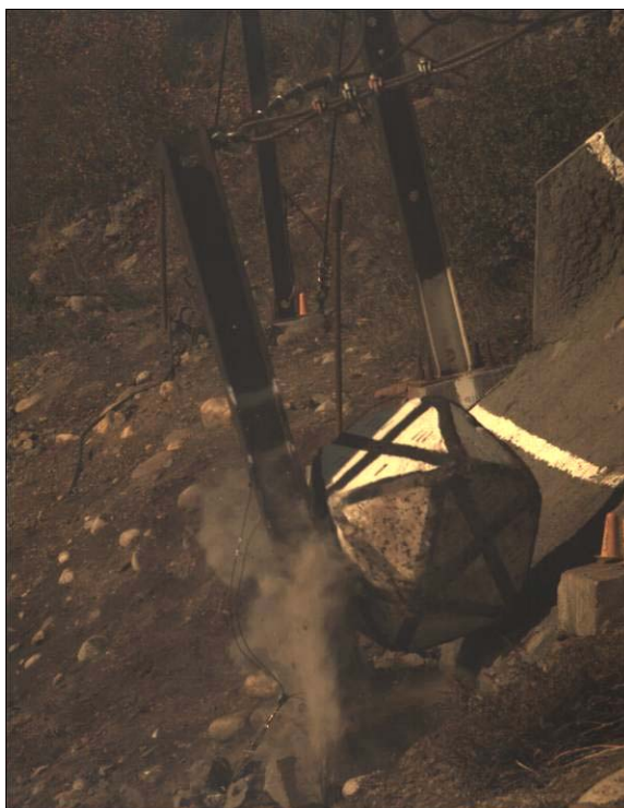
FIGURE 67 Fixed-connection post during impact (Test No. 122).
