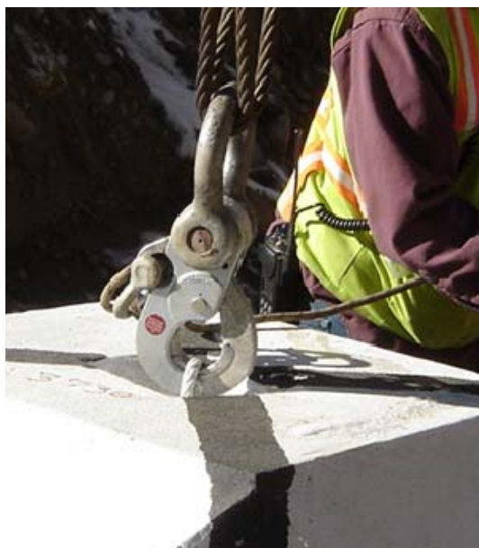
FIGURE 40 Release mechanism attached to a cuboctahedron test block.
