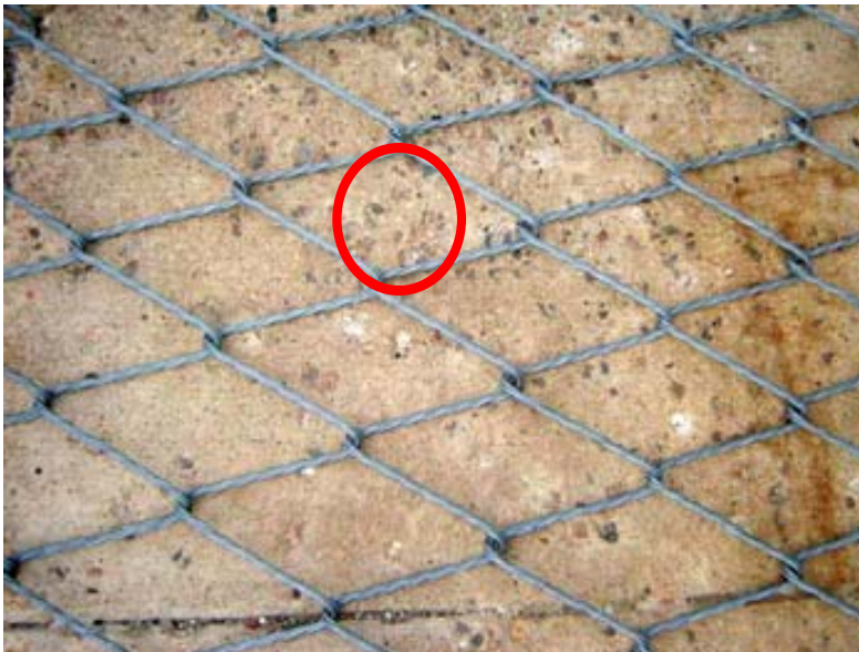
FIGURE 27 Spiral-wire net with aperture opening of 130 mm depicted by red circle. Long axis oriented horizontally showing how net was hung from support rope on attenuator system (support rope would be at top of photograph).
