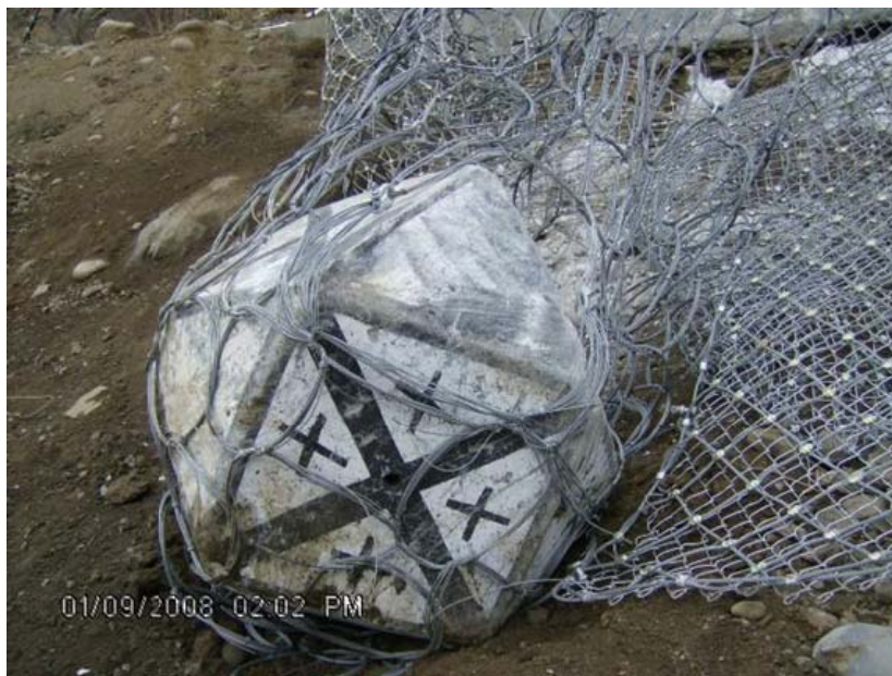
FIGURE 53 Deformation of large-aperture ring net.
