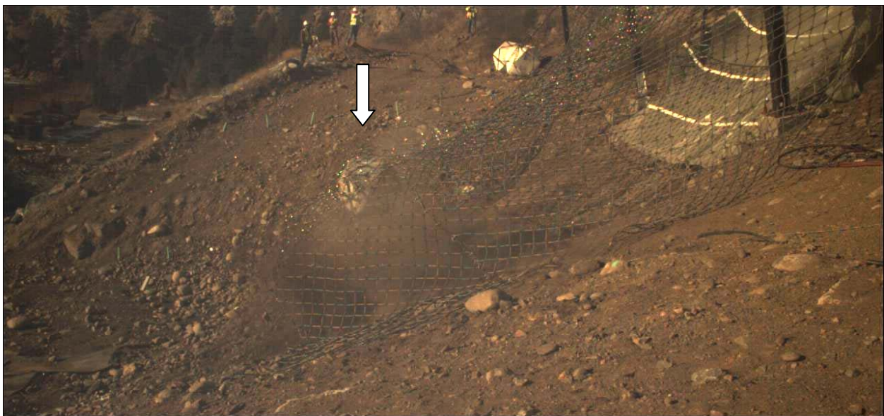
FIGURE 50 Rock momentum greatly reduced as panel and rock vertically rise.
