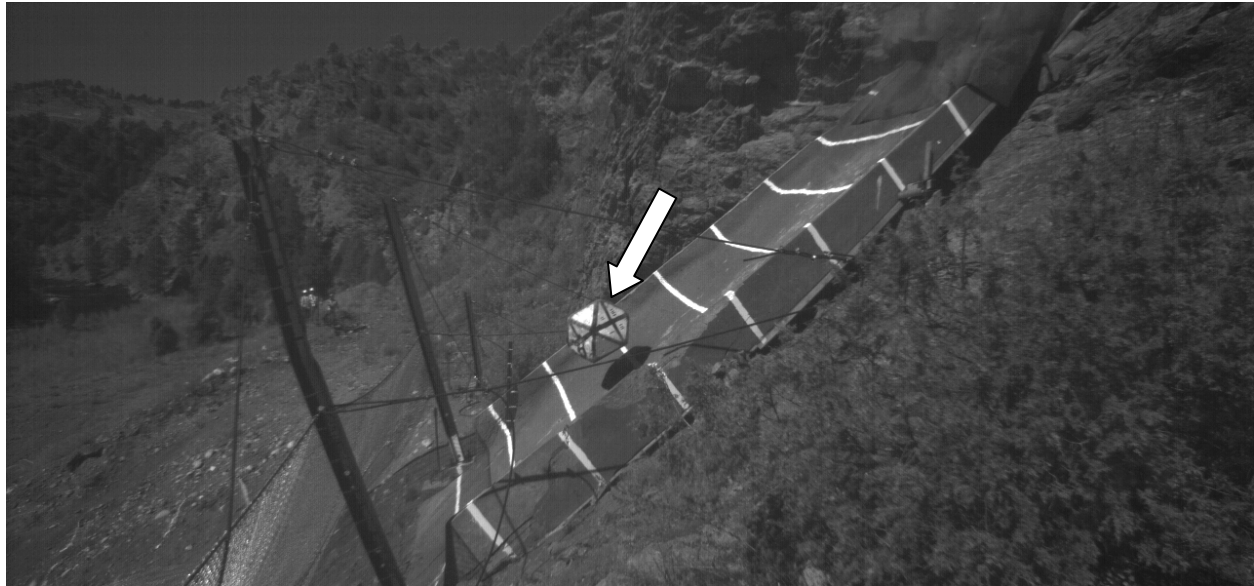
FIGURE 19 Example of photograph taken with Camera 1 prior to impact with net, above post support (white strips are marked on 1.5 m [5 ft] centers; white arrow depicts location of rolling boulder).
