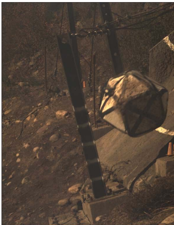
FIGURE 66 Fixed-connection post just prior to impact (Test No. 122).
