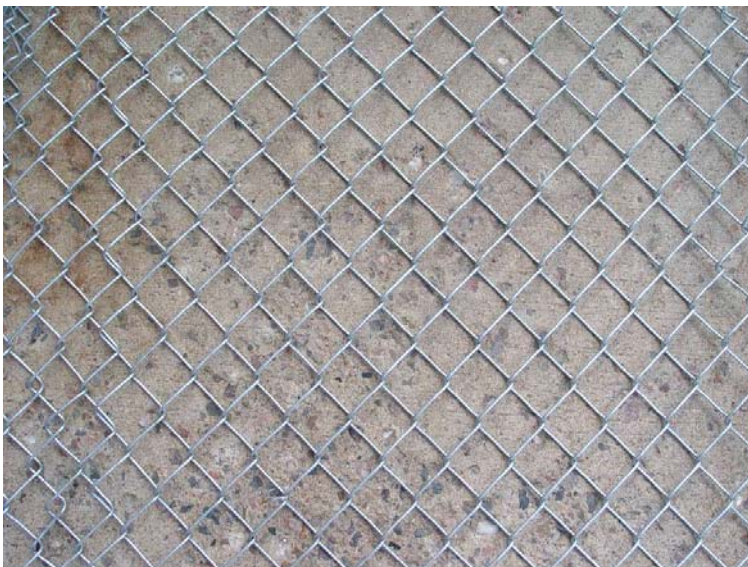
FIGURE 29 Close-up of steel wire (chain link), wire continuous in a vertical orientation showing how net was hung from support rope on attenuator system (support rope would be at top of photograph).
