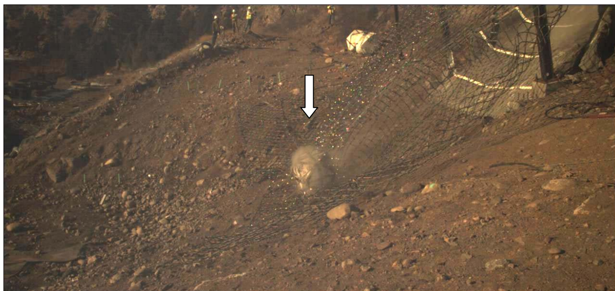
FIGURE 48 Rock engaging panel and beginning to lift tail portion.
