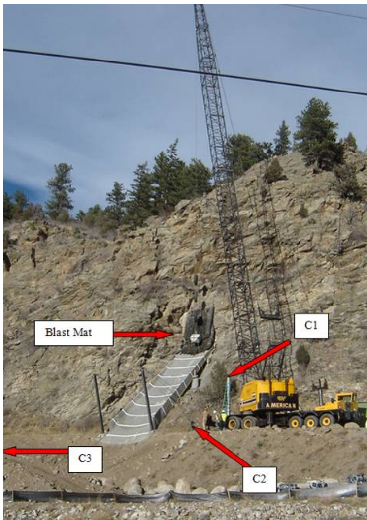
FIGURE 18 Completed Hidden Valley test facility (red arrows depict high-speed camera locations C1, C2, and C3).
