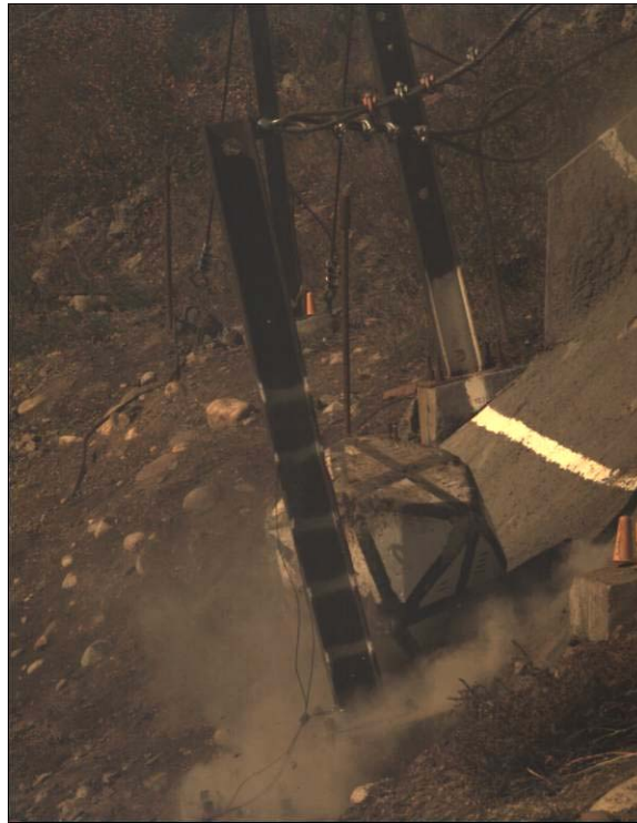
FIGURE 68 Fixed-connection post after impact (Test No. 122).
