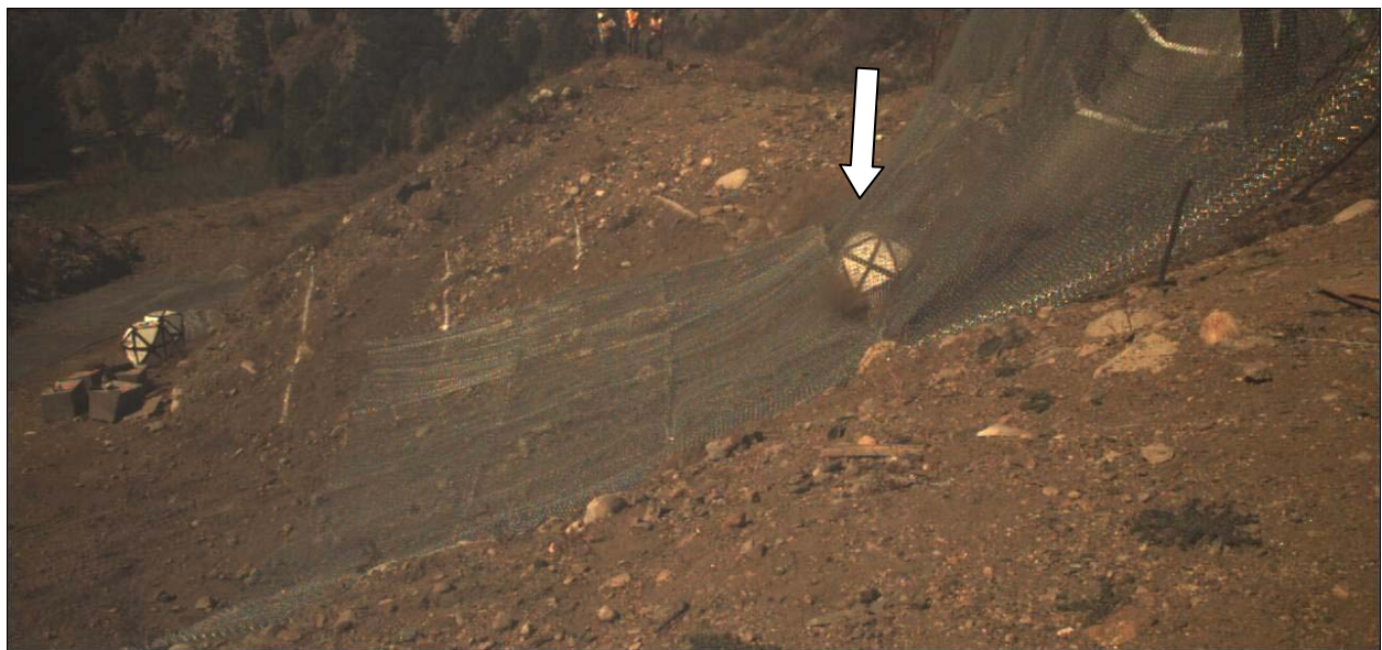
FIGURE 20 Example of photograph taken with Camera 2 during impact with net, below post support (white arrow depicts location of rolling boulder).
