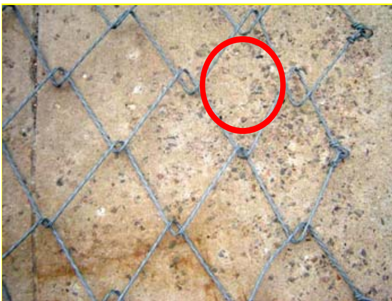
FIGURE 26 Spiral-wire net with aperture opening of 230 mm depicted by red circle. Long axis oriented vertically showing how net was hung from support rope on attenuator system (support rope would be at top of photograph).
