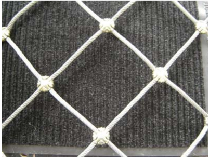
FIGURE 24 Cable net made with 8-mm diameter wire and overlap clamp style (diagonal weave 150 mm by 150 mm).
