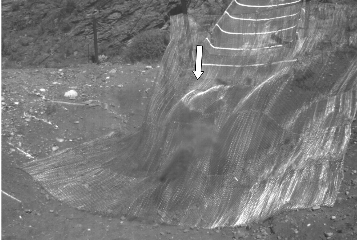
FIGURE 21 Example of photograph taken with Camera 3 during impact with net, below post support (white arrow depicts location of rolling boulder).
