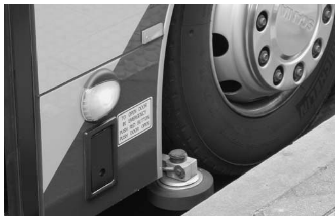
Figure 7 Horizontal guide wheels engage raised concrete edges on the O-Bahn track to automatically steer the bus.
